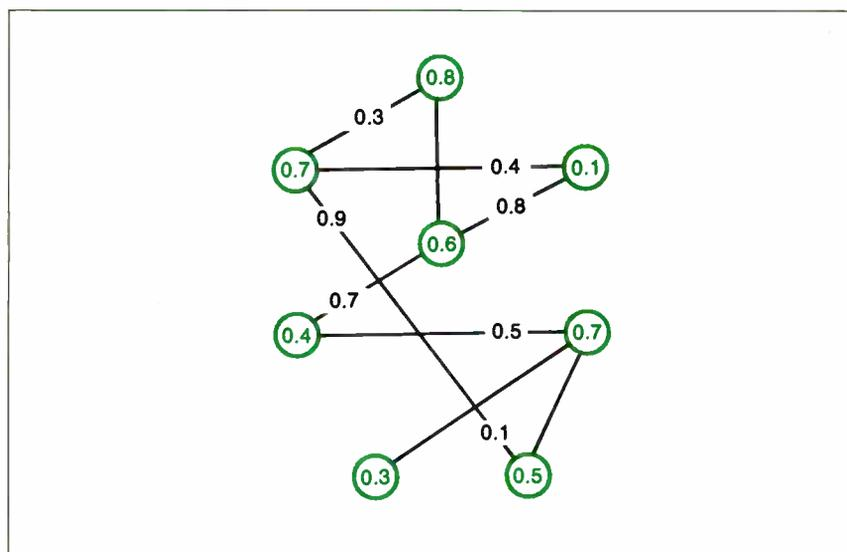
**Figure 1:** In a typical neural network, every node has an activation, and every connection between nodes has a weight. A rule, which varies from network to network, governs the way in which weights and activations change over time.
