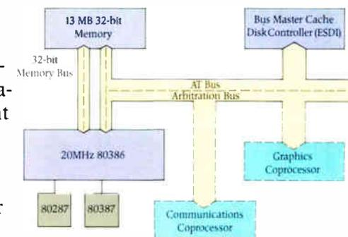
AST's Multimaster Bus technology allows direct access to main memory for faster overall system throughput.
