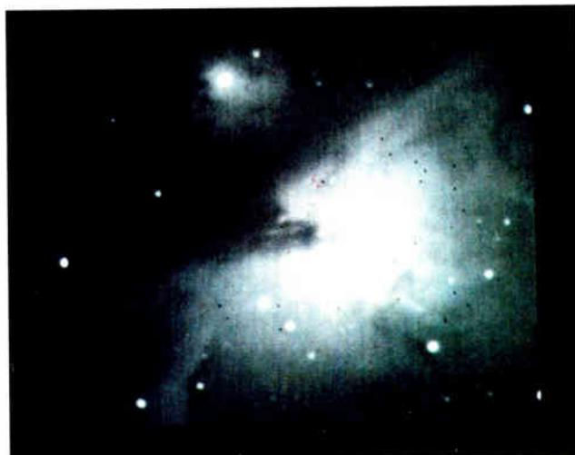
**Photo 1a:** This raw image of M42, the Orion nebula, was taken with a 1-minute exposure and a warm (5°C) imager. The image has a substantial background of thermal noise and numerous hot spots or saturated pixels.
