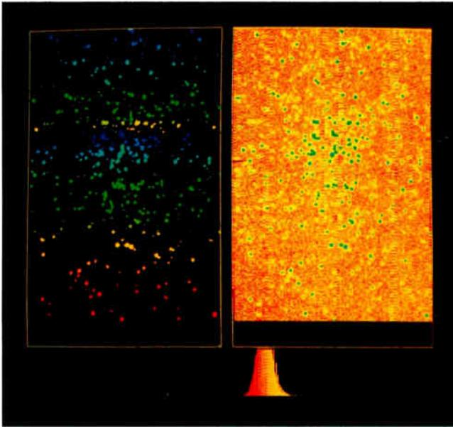
**Photo 7:** The enhanced image of the star cluster M37 is on the right. The Groups subroutine assigns to an appropriate group each star in the cluster that has a pixel value exceeding a certain threshold value. Then the subroutine assigns each group a number for color coding as the groups are plotted on the left. The bottom of each image has been clipped because of high noise levels in this area.
