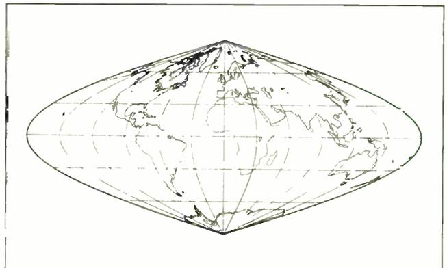
**Figure 2:** Sinusoidal projection is easy to compute and preserves the relative area of land masses, but it distorts their shape.
