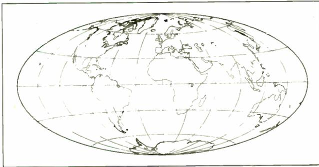
**Figure 5:** The Hammer is another equal-area projection. It is more realistic than the Sinusoidal, but its curved parallels and meridians make it more difficult to construct.
