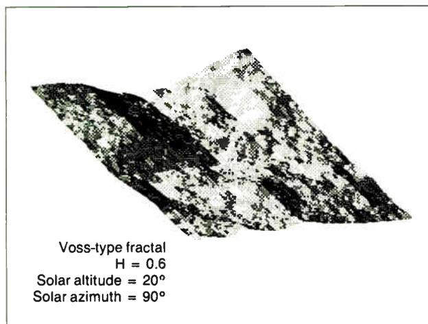
Figure 10: A shaded three-dimensional projection of a fractal surface.
