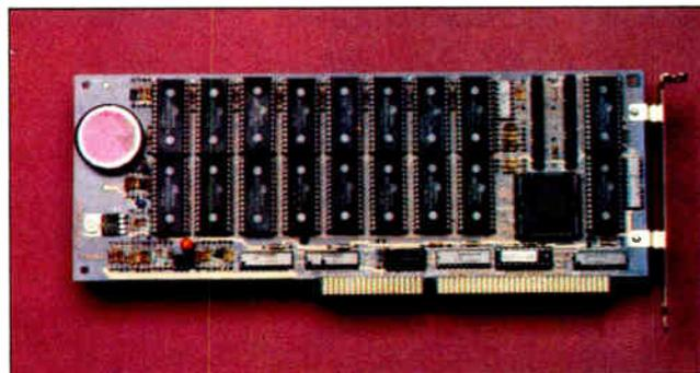
The Awesome I/O card is designed to improve the throughput, capacity, and reliability of your hard disk. Using on-board nonvolatile CMOS RAM (256K or 512K bytes, 100 nanoseconds) managed by an intelligent control unit called the Heuristic Adaptive I/O Controller, the Awesome I/O card determines and caches your most frequently used hard disk data.
