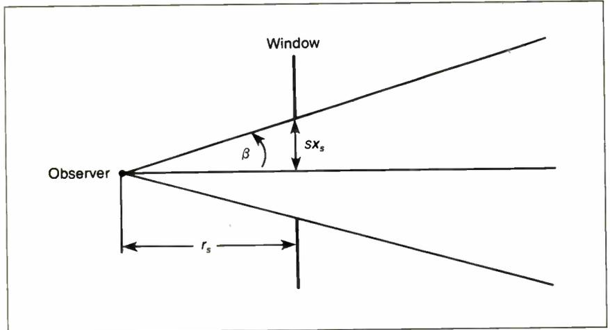
**Figure 4: Viewing an object through a window.** Here, we are measuring the size of the object's image,  $sx_o$ , in relation to other angles and distances.
