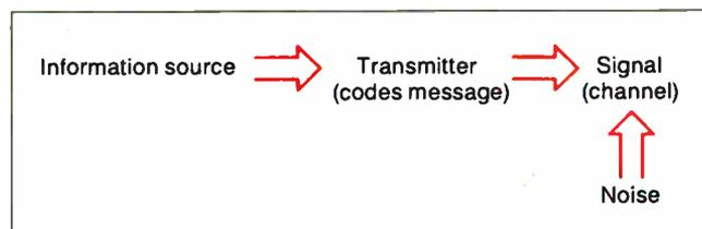
Figure 1a: The process that occurs at the transmission end of communicating a message.
