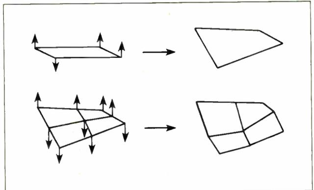
**Figure 2:** Steps 1 and 2 of the midpoint-displacement algorithm.
