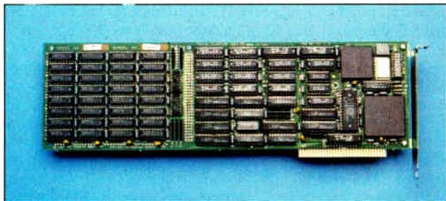
The PC-Elevator 386 is an unusual 16-megahertz 80386 add-in board for the IBM PC, XT, or AT. The base unit (\$1995) comes with 1 megabyte of on-board 100-nanosecond memory, a socket for an optional 80387 coprocessor (\$795), disk caching and EMS (Expanded Memory Specification) memory management software, and a bus for attaching up to 16 megabytes of memory via optional daughtercards (\$2000 for each 4-megabyte daughtercard).
