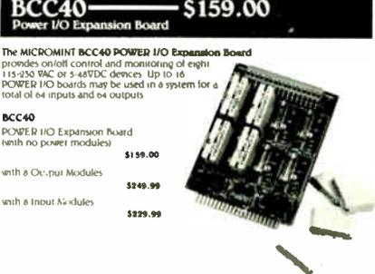
The MICROMINT BCC40 POWER I/O Expansion Board provides on/off control and monitoring of eight 115-230 VAC or 5-48VDC devices. Up to 16 POWER I/O boards may be used in a system for a total of 64 inputs and 64 outputs.
