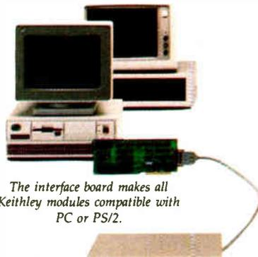
The interface board makes all Keithley modules compatible with PC or PS/2.
