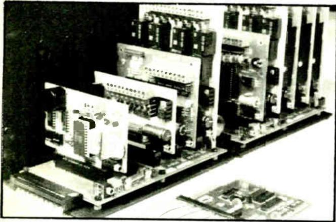
An A-BUS system with two Motherboards
