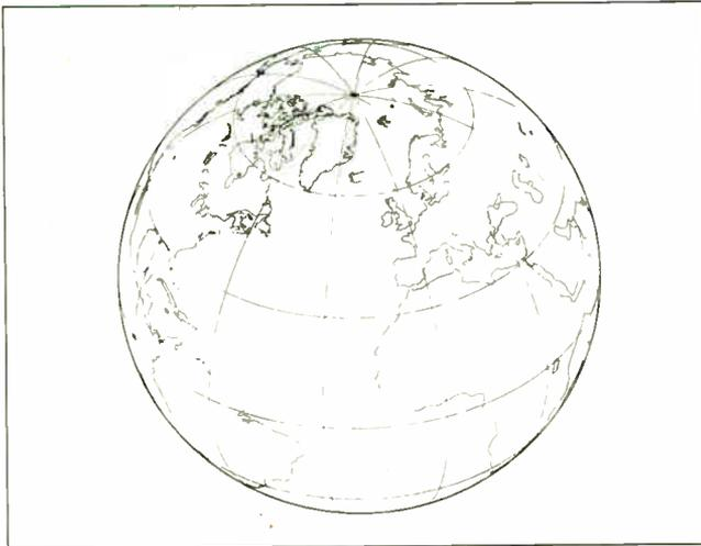
**Figure 4:** Orthographic projection displays only one hemisphere at a time. The center of the map is the only point without distortion.
