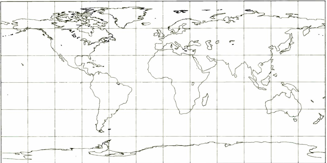
**Figure 1:** *Equidistant Cylindrical projection is easy to implement, but it distorts both the shape and the area of land masses.*
