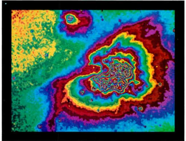
**Photo 1c:** Application of the median-value filter has smoothed the image somewhat and removed the defective pixel values.
