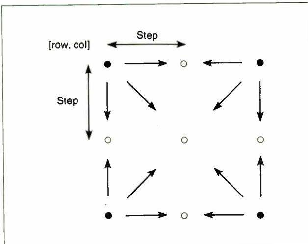
**Figure 3:** Finding new points in the calculations of the midpoint displacement.
