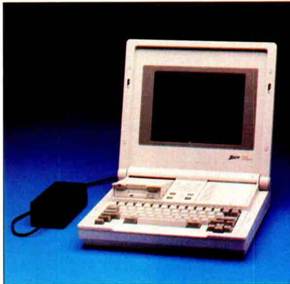
nearly 2 inches in depth and ½ inch in width and height. More significantly, the inclusion of the hard disk drive and a larger battery pack has increased the computer's weight from 12 pounds to almost 16 pounds.
