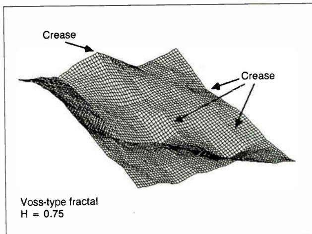
**Figure 6: Creases generated by the Voss fractal algorithm.**
