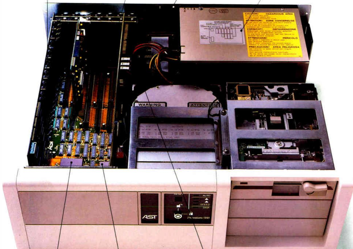
20 MHz, 80386 processor for high performance, AT-compatible desktop computing.
