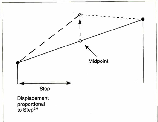
**Figure 4:** Calculating the height of a new point by the midpoint-displacement method.
