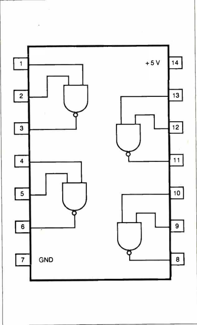
**Figure 1: Pin-out for a 7400 quad two-input NAND gate.**
