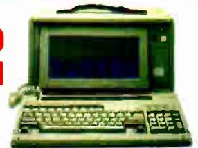
■ Liquid Crystal Display Combining Rat Panel, Super Twist Display Technology with Electro Luminescent Backlight.
