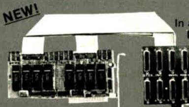
In a class all by itself, the NEW PCSS-8X Multiport Serial Board has impressed the market with its unlimited functions. This board has 100% Dos compatibility on all 8 ports and an enhanced INT 14H Bios device driver. A truly state-of-the-art product.
