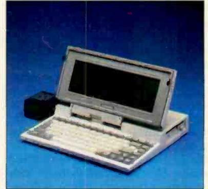
**Photo A:** *The Toshiba T1000 is a 6½-pound 80C88-based laptop that operates from rechargeable batteries.*
