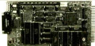
The BCC180, only 4.5" x 8.5", uses the same 68418i CMOS 2.80 instruction compatible processor as Micromint's SB180 and SB180FX single board computers. Configured primarily for process control w/584K of memory, 6 parallel I/O ports, a console serial port, RS-232C/485 selectable auxiliary serial port, and an interrupt driven ROM resident multitasking BASIC-180 compiler, the BCC180 uses the same 44-pin I/O expansion bus as Micromint's BCC52 controller board.
