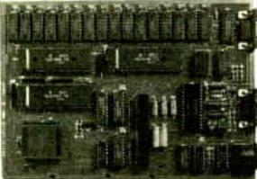
The GT180 has both TTL RGB (red-green-blue intensity) and analog RGB outputs. It is totally compatible with virtually all standard and multisync CRT monitors and has a connector for an IBM PC keyboard.
