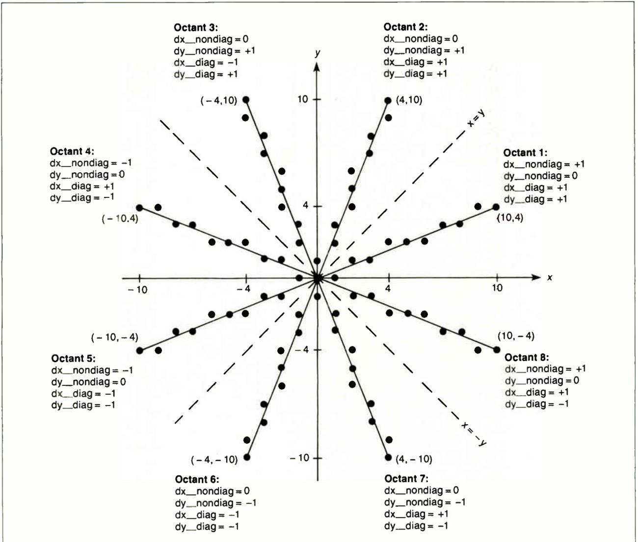
Figure 4: Eight-way symmetry used for the general algorithm.
