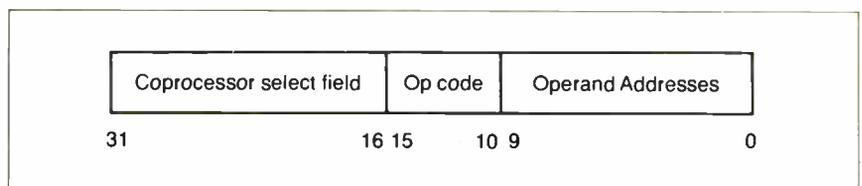
Figure 2: The Weitek 1167 view of the 80386 address bus.
