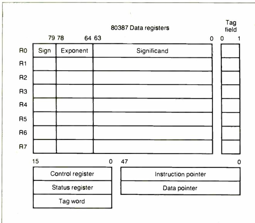
Figure 1: The register model of the 80387.
