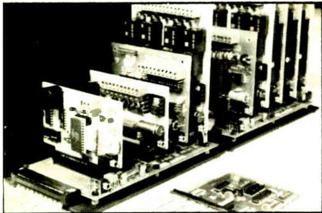
An A-BUS system with two Motherboards
