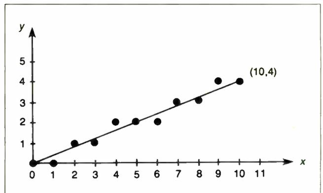
Figure 2: Pixel approximations of line from origin to (10,4).
