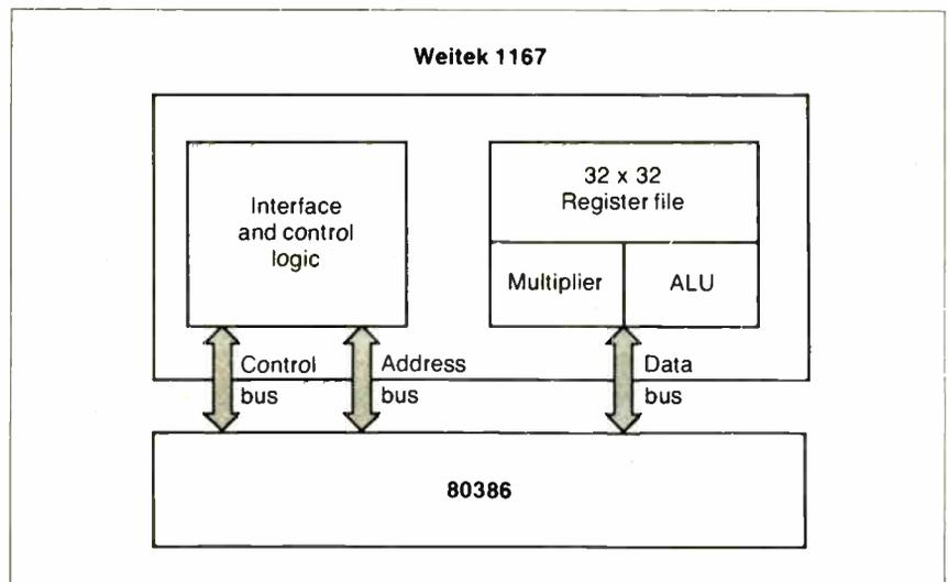
Figure 1: A block diagram of the 80386/Weitek 1167 interface.
