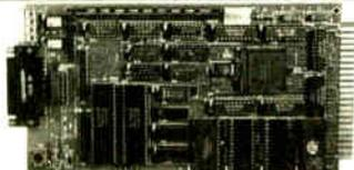
The BCC180, only 4.5" x 8.5", uses the same 68418i CMOS 2.80 instruction compatible processor as Micromint's SB180 and SB180FX single board computers. Configured primarily for process control w/584K of memory, 6 parallel I/O ports, a console serial port, RS-232C/485 selectable auxiliary serial port, and an interrupt driven ROM resident multitasking BASIC-180 compiler, the BCC180 uses the same 44-pin I/O expansion bus as Micromint's BCC52 controller board.
