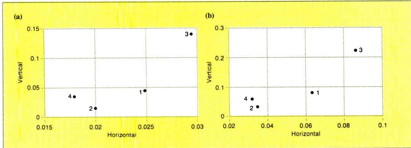
SuperMac card. Other measurements, such as line variation, were better for the SuperMac; this suggests sample-to-sample variations in factory adjustments. The Machroma monitor had the largest spot size and the largest variation between the center and the corner of the screen.
