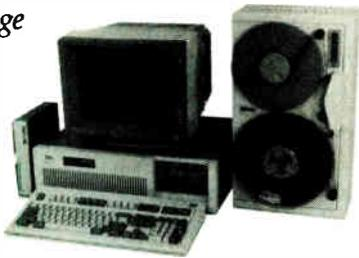
With 9-track tape, you are free to exchange data files with any mainframe or minicomputer in the world.
