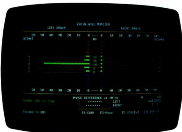
**Photo 3:** While testing HAL, I injected a 10-Hz sine wave through the headset electronics. The resulting output, shown here, indicates that the system works properly.
