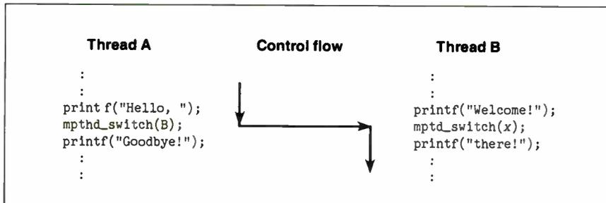
**Figure 1:** Context switching as performed by `mpthd_switch()`. The output from this context switch would be "Hello, there!"; "Hello," comes from thread A, which switches to thread B for "there!".
