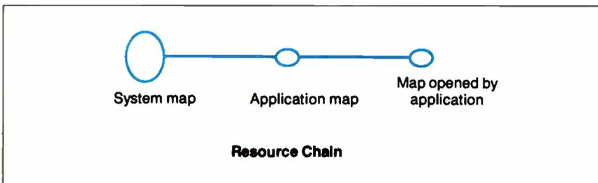
Figure 2a: The original MultiFinder plan for sharing resources involves searching a resource chain like this one.
