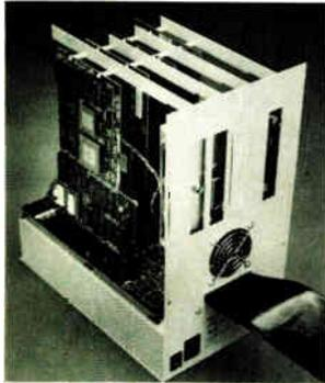
Second Wave expansion chassis come complete with an interface card, cables, and the chassis with SE or NuBus slots, a power supply and fan.
