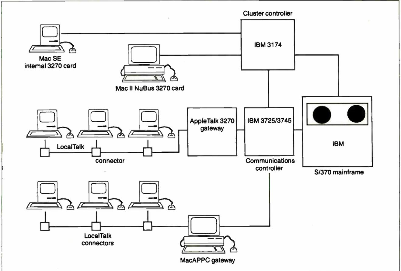
Figure 3: MacAPPC goes beyond 3270 terminal emulation and 3270 gateways to let the Mac act as an intelligent peer node on an IBM SNA network.
