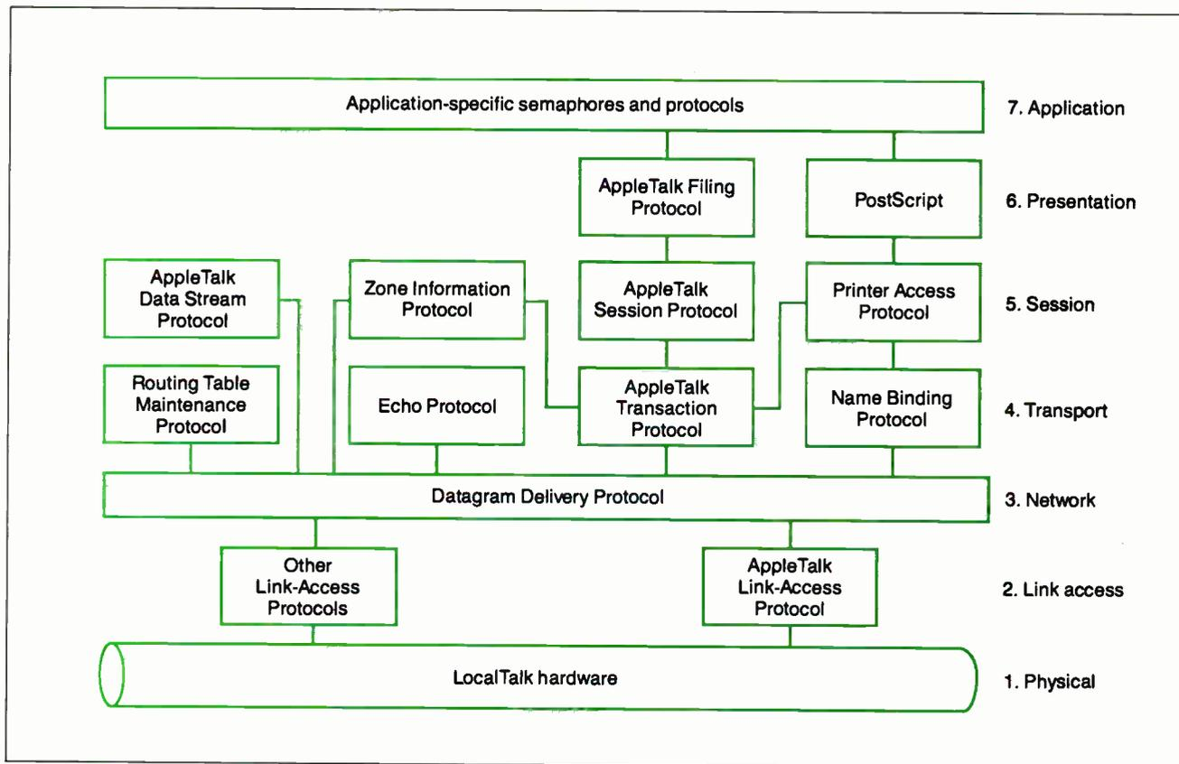
**Figure 1:** AppleTalk's seven-layer architecture is similar to that of the OSI reference model. The protocols, however, are proprietary.
