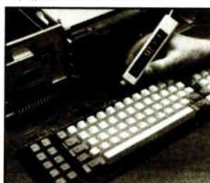
After you build this digital logic probe, you'll explore the operation of the Sanyo detached "intelligent" keyboard and its dedicated microprocessor.
