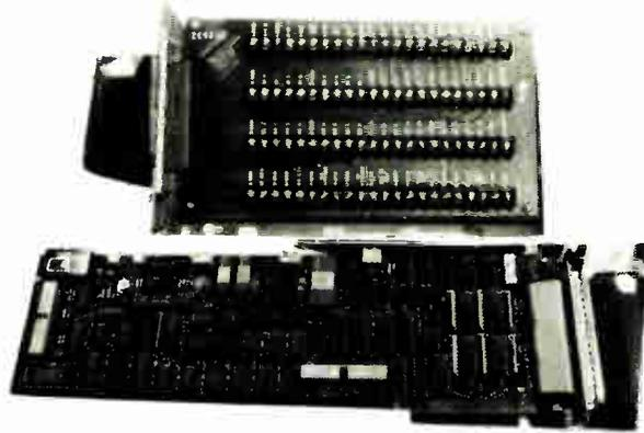
**IBM PC\*DATA ACQUISITION AND CONTROL ADAPTER** provides an easy to use interface for accessing the ANALOG and DIGITAL I/O. Integrates analog, binary and time/counter devices on a single adapter card.
