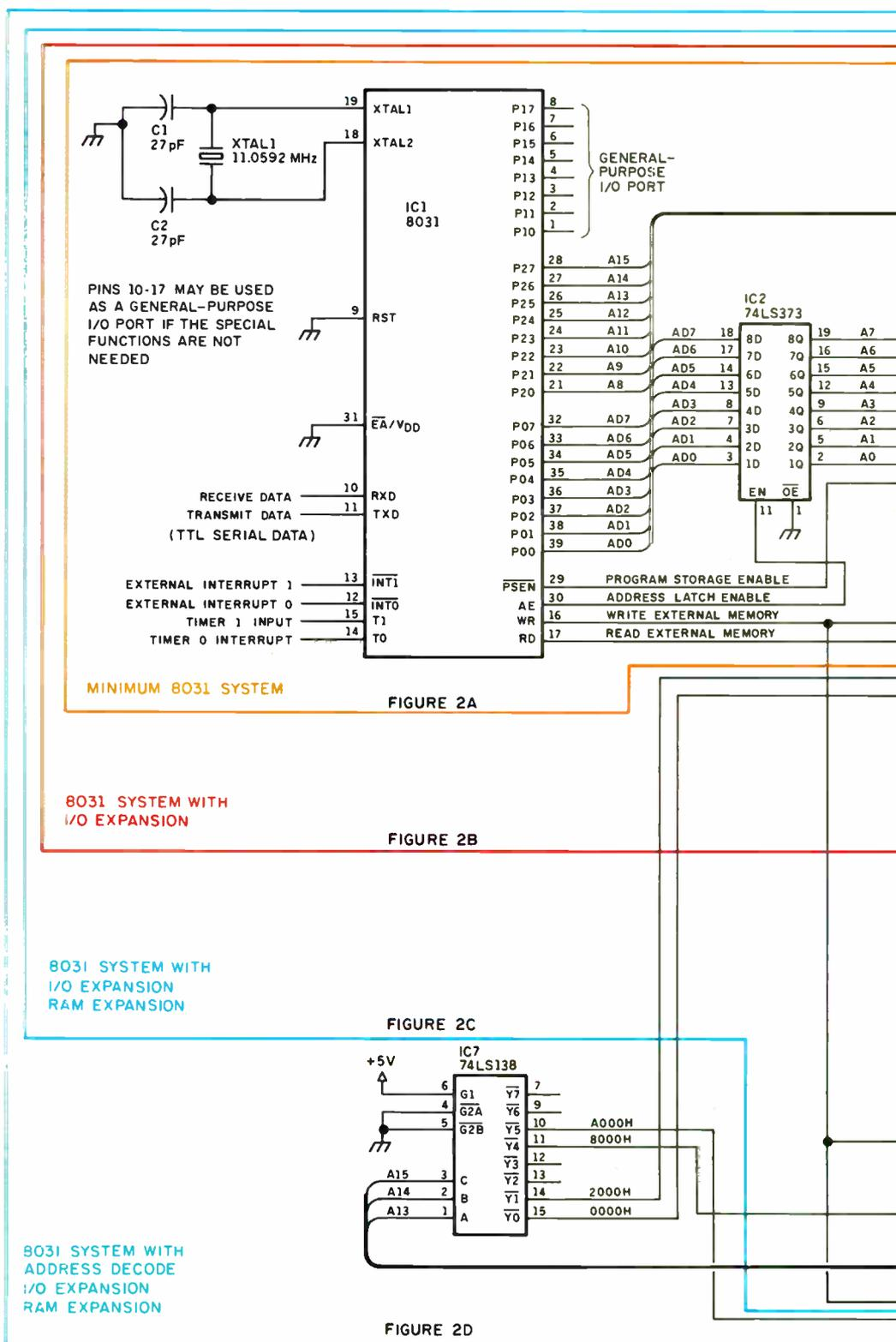
Figure 2: Growing an 8031 system. (a) A minimum configuration, (b) minimum system with I/O expansion, (c) system with I/O and RAM expansion, and (d) system with address decode logic and even more RAM and I/O.
