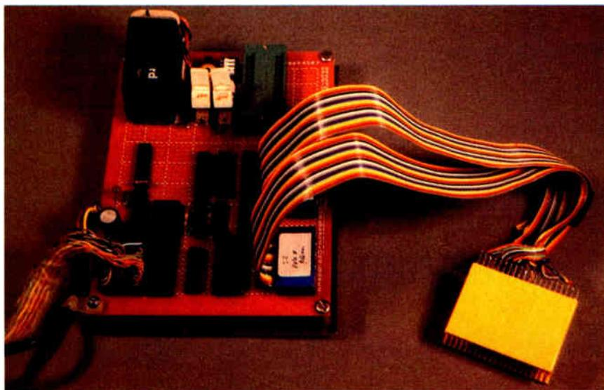
**Photo 2:** A prototype of the DDT-51 development system. Note the DIP clip at the end of the cable for attaching onto the target system's processor.
