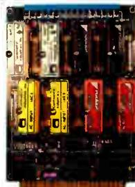
The Micromint BCC40D is an 8-channel optoisolated input/output expansion board designed for use with Micromint's family of BCC-bus Computer/Controllers. Using industry-standard optoisolated I/O modules, the BCC40D provides on/off control and input monitoring of eight 115-230VAC or 5-48VDC devices used in data acquisition and control applications.
