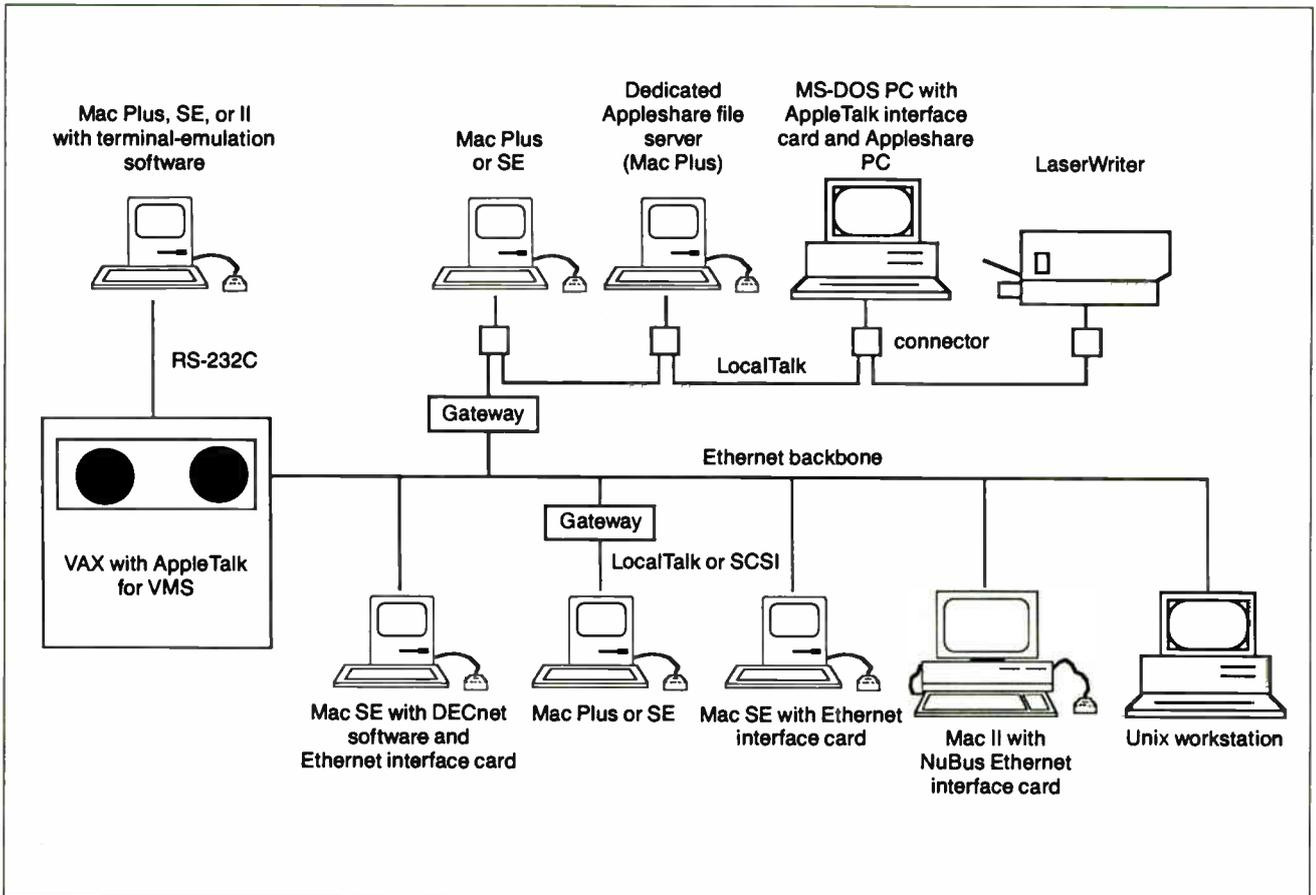
Figure 2: Macs connected to DECnet's Ethernet backbone can function as DECnet nodes, or the VAX can act as an AppleTalk file server.
