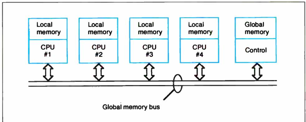
**Figure 13:** A four-way direct-connected multiprocessor system.
