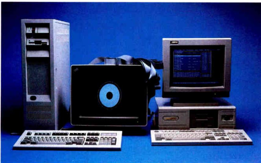
Photo 3: Remote debugging with Turbo Debugger. The machine on the left is executing the BYTE low-level graphics benchmark program, controlled via a serial connection with the machine on the right running the debugger.
