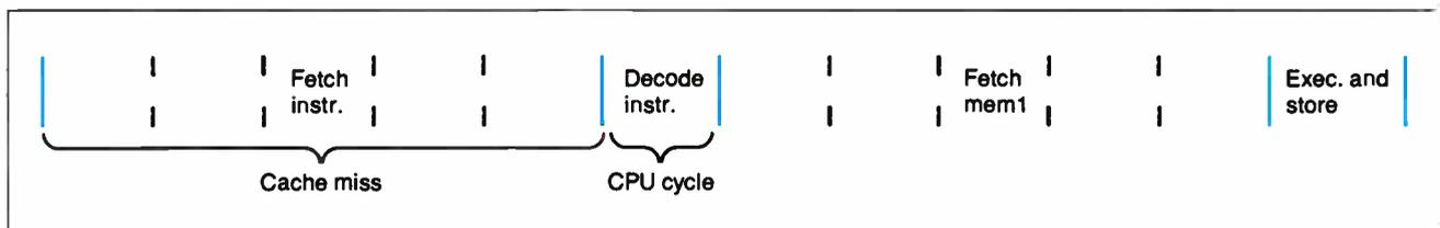
**Figure 7b:** Executing the same instruction as in figure 7a with five-cycle cache misses.
