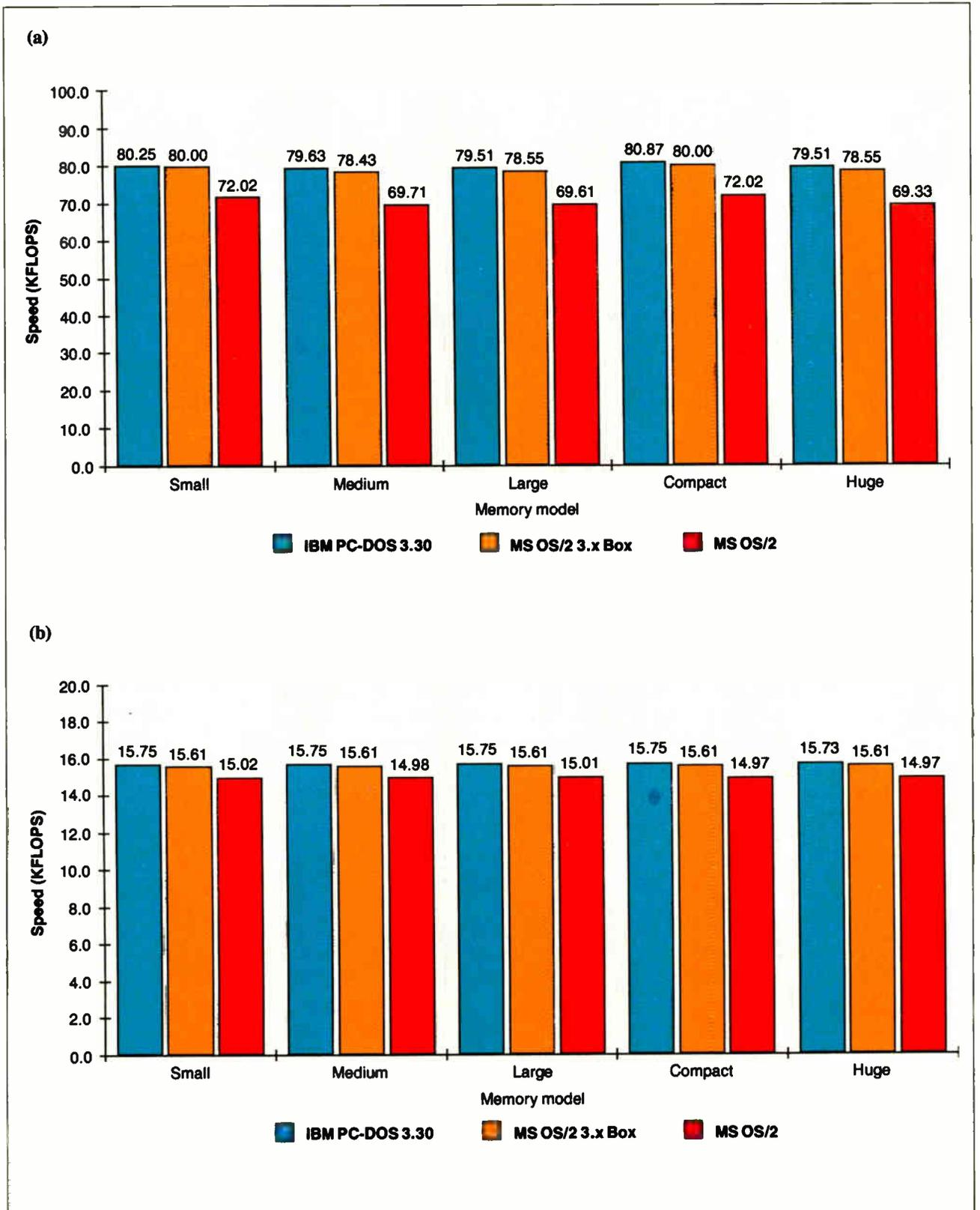
**Figure 2:** Floating point rate (in kiloflops) of the Savage floating point benchmark run under DOS, the OS/2 compatibility box, and OS/2 protected mode. Note that the compatibility box slowed the programs by a few percent, while OS/2 slowed them by about 10 percent on the Trillian Power Systems 386 (a), and 5 percent on the IBM PC AT (b).
