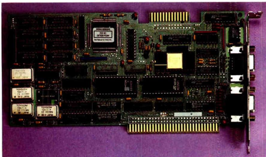
An intelligent graphics card that offers a universal solution to the multiple PC display standards. It supports all the current IBM PC and PS/2 display modes and monitors and it's 100% hardware compatible in all modes. Ideal for use with the NEC Multisync II
