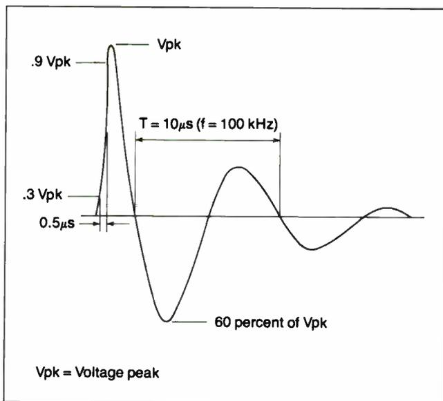
**Figure 5:** The IEEE 587 ring wave is a testing standard for surge-suppression products. Engineers have found this wave shape to be typical of what might appear on 120-V circuits leading to your computer.
