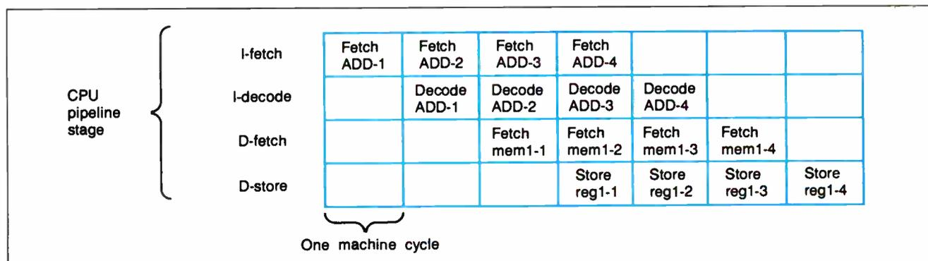
Figure 9: The CPU from figure 8 executes a series of ADD mem1, reg instructions.
