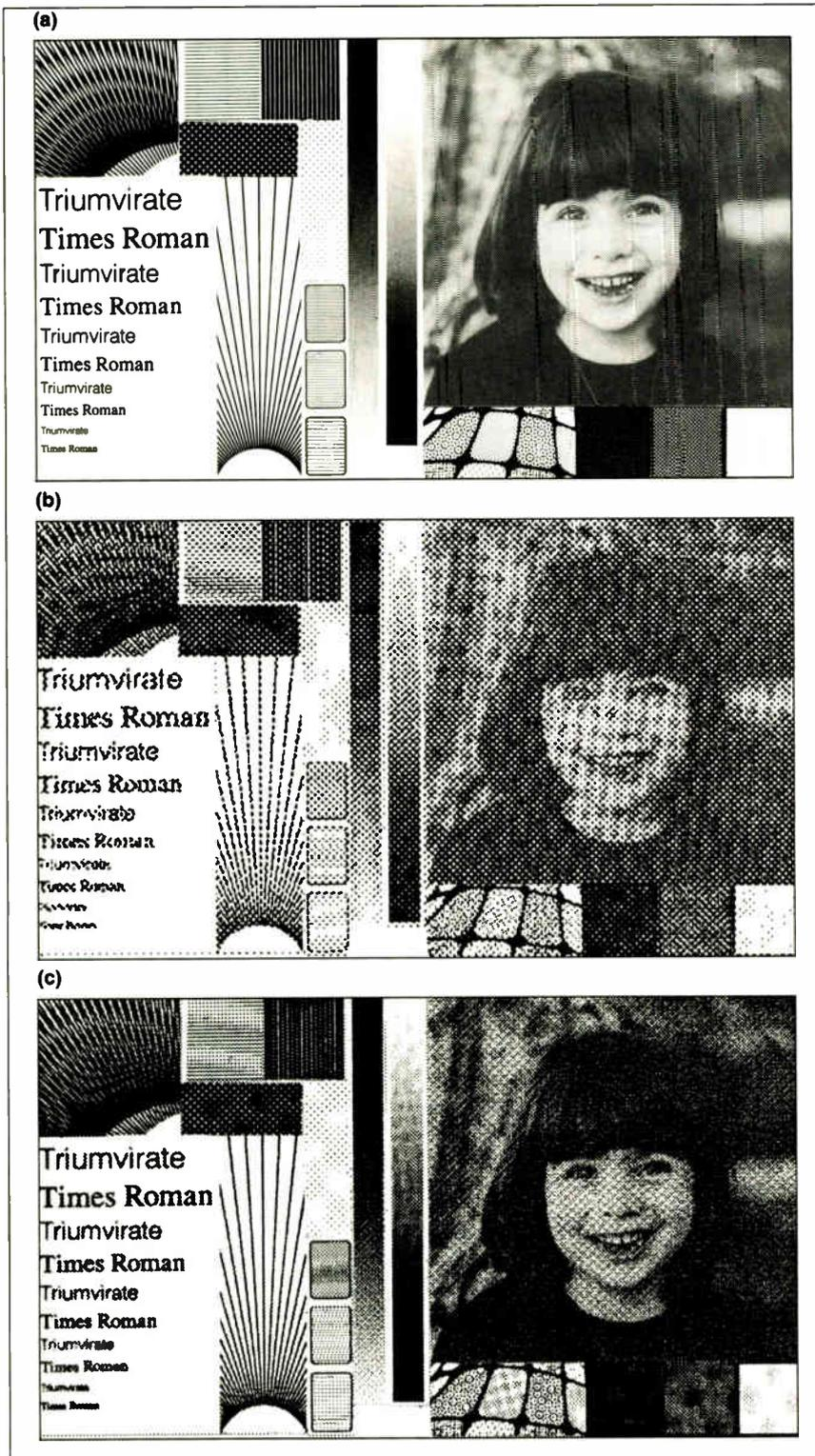
**Figure 1:** (a) *BYTE's* test pattern for scanner quality. (b) The test pattern scanned at 150 dpi. The Microtek scanner was adjusted for halftone scanning to accommodate the halftone image. When the scanner was adjusted for line art, the lines and patterns looked considerably better, but the halftone's quality suffered. (c) The test pattern scanned at 300 dpi, halftone setting. Notice the improvement in the lines and patterns as well as in the halftone image. All images are actual size.
