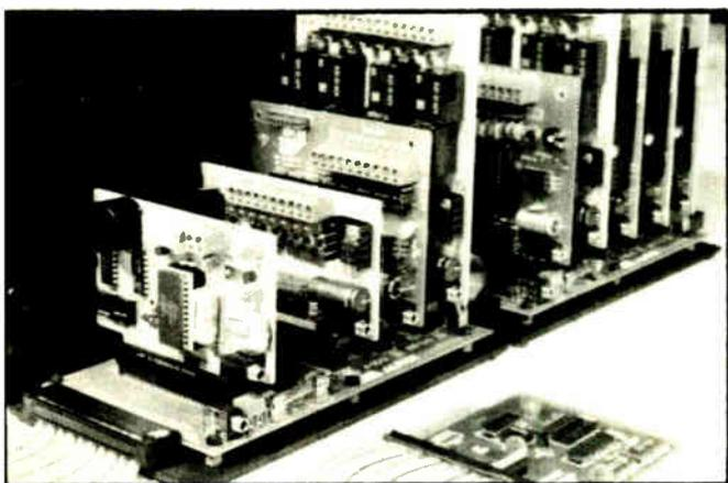
An A-BUS system with two Motherboards
