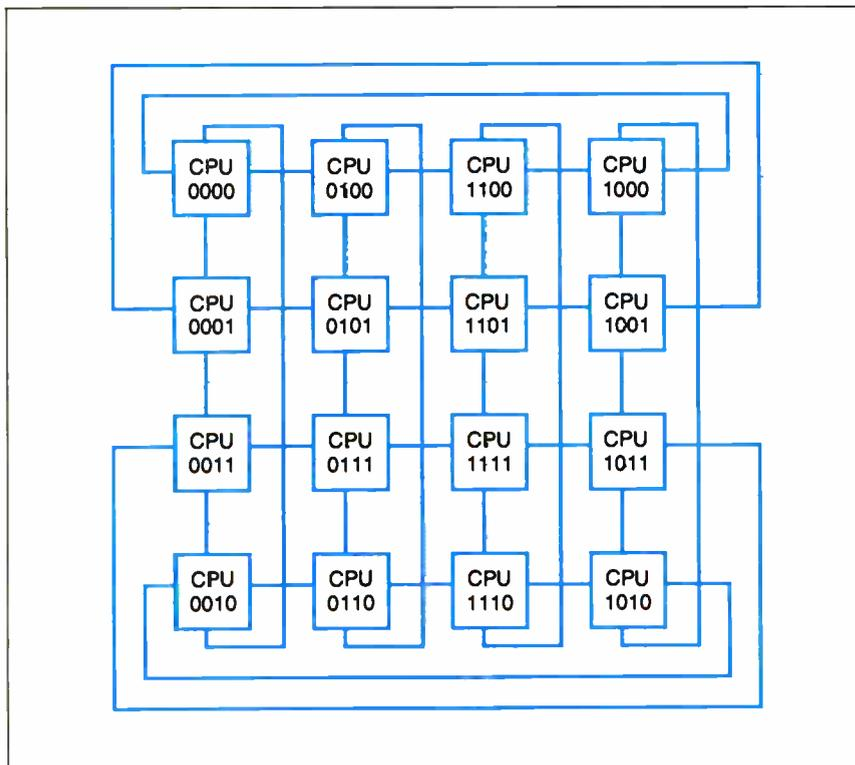
**Figure 16:** The processors from figure 15 are each assigned an ID number to simplify message passing.
