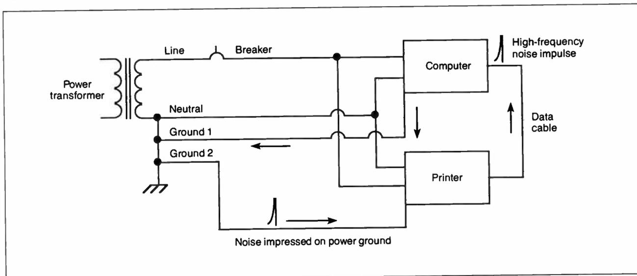
**Figure 4:** Noise current will take the path of least resistance, a situation that may interfere with the transmission of data between devices or even cause damage.
