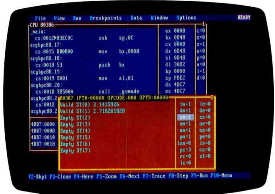
**Photo 2: Turbo Debugger's numeric coprocessor window lets you dive into your system's floating-point unit (in this case, an 80387). Notice that you can enter numbers directly into the coprocessor's registers.**
