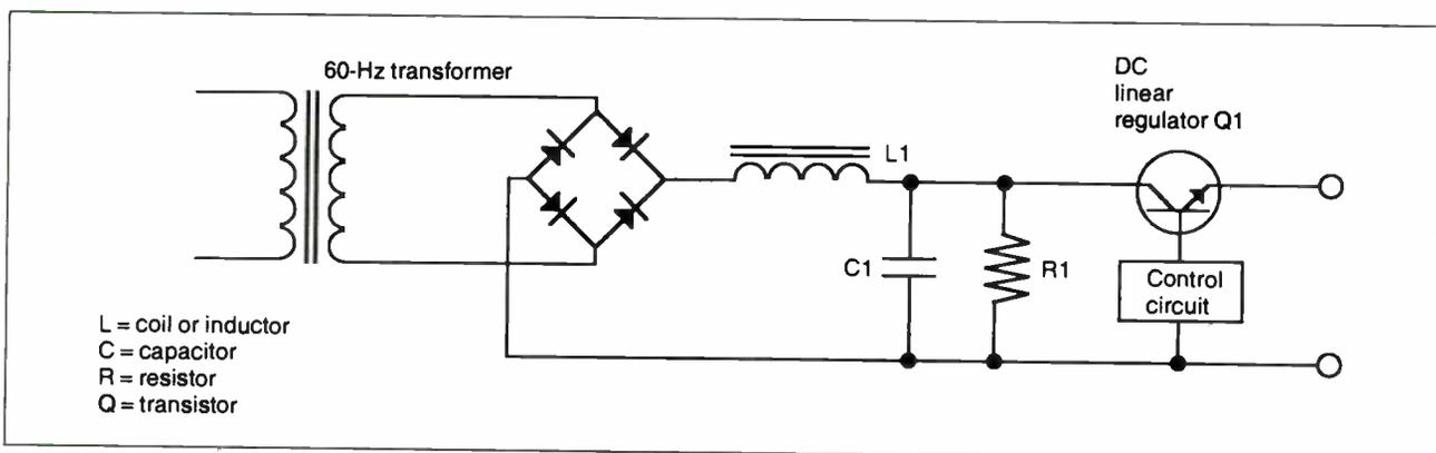
**Figure 1:** Linear power supplies, used in small computers up until a few years ago, featured a large 60-Hz power transformer connected across the input. Such power supplies were sensitive to variations in voltage and made power supplies bulky.
