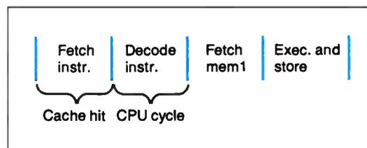
**Figure 7a:** Executing the instruction ADD mem1, reg on the cached system, assuming one-cycle cache hits.
