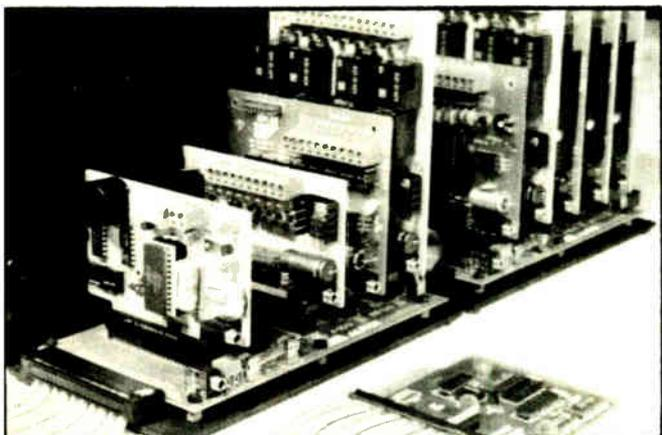
An A-BUS system with two Motherboards
