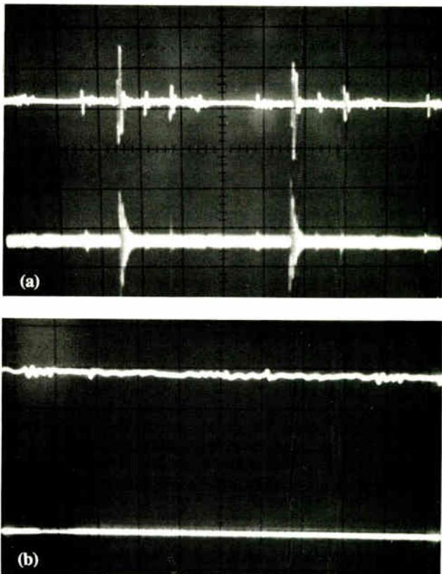
Photo 2: These photos show noise in an electrical circuit, (a) before and (b) after insertion of a power-line conditioner. In both photos, the top trace is normal-mode noise and the bottom trace is common-mode noise.
