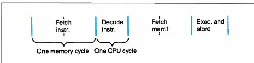
**Figure 4:** *Execution sequence for ADD mem1, reg. Note that memory access is now two CPU cycles (see text).*
