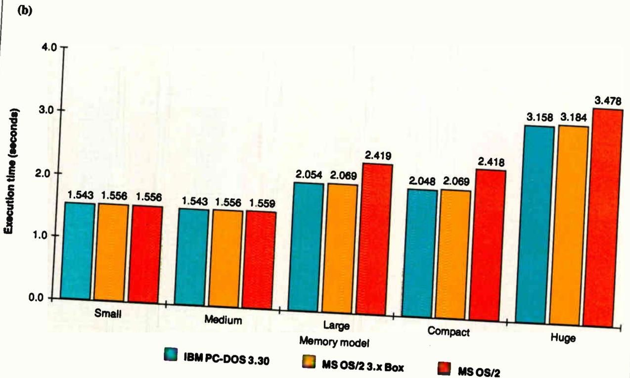
**Figure 1:** According to my tests with small memory models, the Sieve of Eratosthenes took somewhat longer to run in the compatibility box and in OS/2 protected mode than in DOS. Using larger memory models, however, OS/2 took as much as 44 percent longer on a 16-MHz Trillian Power Systems 386 (a), and 18 percent longer on an 8-MHz IBM PC AT (b).
