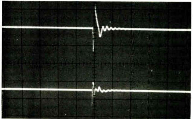
Photo 1: As the impulse in the normal mode (top trace) is conducted by the MOV from line to neutral, another impulse (bottom trace) appears between neutral and ground, the common mode.
