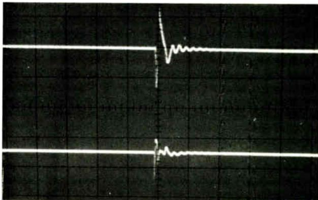
Photo 1: As the impulse in the normal mode (top trace) is conducted by the MOV from line to neutral, another impulse (bottom trace) appears between neutral and ground, the common mode.
