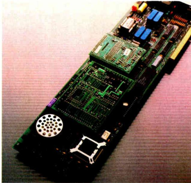
Connection Coprocessor multitasking board from Intel.
