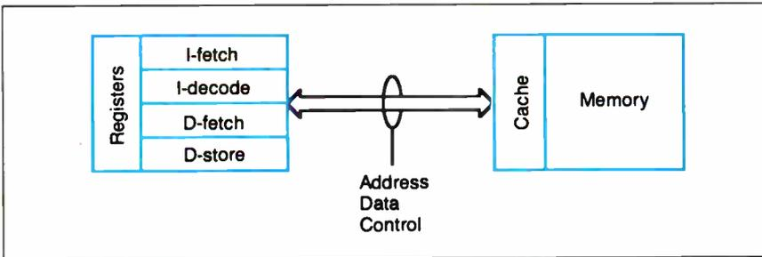
Figure 8: In a final attempt to improve throughput, pipelining is added to the CPU.
