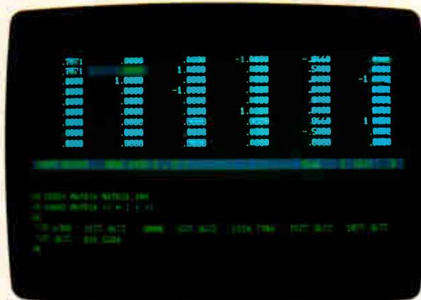
It takes just one command and 47 milliseconds to calculate the inverse of a general 9 x 9 matrix.
