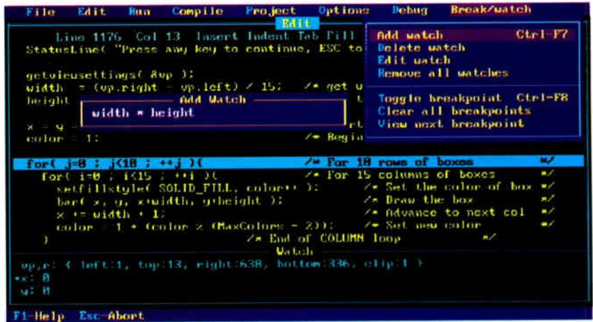
Debugging in the Turbo environment: shown here an expression is being added to the Watch window in Turbo C. The Execution Bar highlights the next line the debugger will execute.
