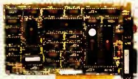
The JE1050 is a monochrome graphics card with parallel printer port and features the following: • Text mode: 80 x 25; Graphics mode: 720 x 348 • Compact half-card • Parallel printer interface with transfer rate up to 1000 characters per second • Manual included
