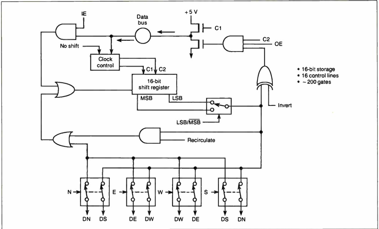
Figure 4: The Shifter wafer type (formerly memory).
