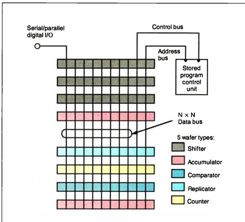
**Figure 2:** Schematic of the system organization. The silicon wafers are represented by horizontal rectangles, and the vertical lines running through the stack depict the data, control, and I/O buses.
