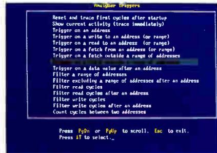
**Analyzer Triggers.** Commonly used triggers can be selected quickly from a list of standard and user-defined triggers.
