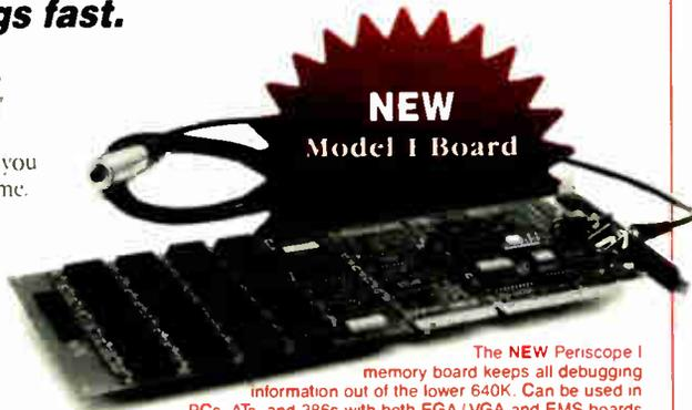
The **NEW** Periscope I memory board keeps all debugging information out of the lower 640K. Can be used in PCs, ATs, and 386s with both EGA/VGA and EMS boards installed. The Periscope break-out switch enables you to recover from a hung system. Included with Models I, II, and III.
