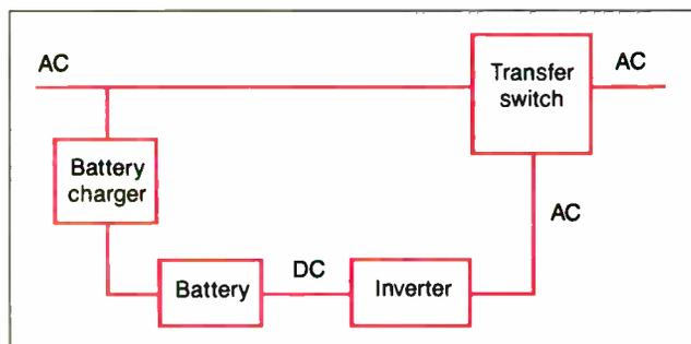
**Figure 1:** The building blocks of an SPS are the battery and the inverter. The battery powers the inverter, which converts DC into AC. Notice that these blocks only operate when the transfer switch senses that utility power has failed.
