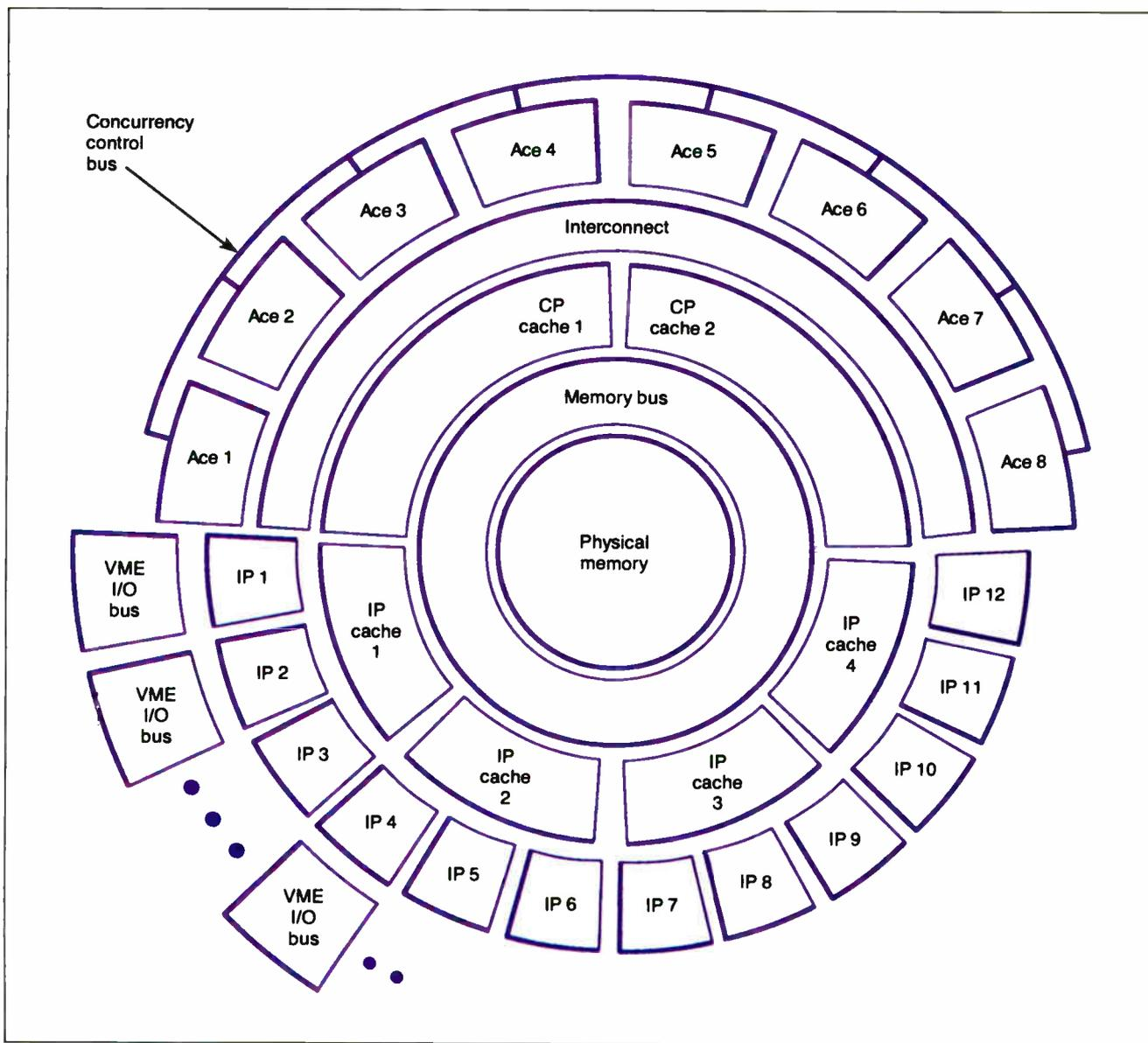
**Figure 2a:** The FX/8 system's common-bus architecture. The ACE processors (Advanced Computational Elements) function as application processors. I/O and operating-system jobs are performed by the interactive processors, which are 68020-based.
