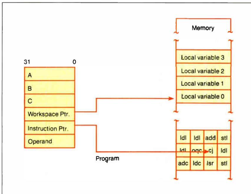
**Figure 3:** The T800 integer CPU has three accumulators, registers A, B, and C, arranged as a stack for expression evaluation. Zero-address instructions operate on values in the stack; single-address instructions load values from memory into the stack, and so on.
