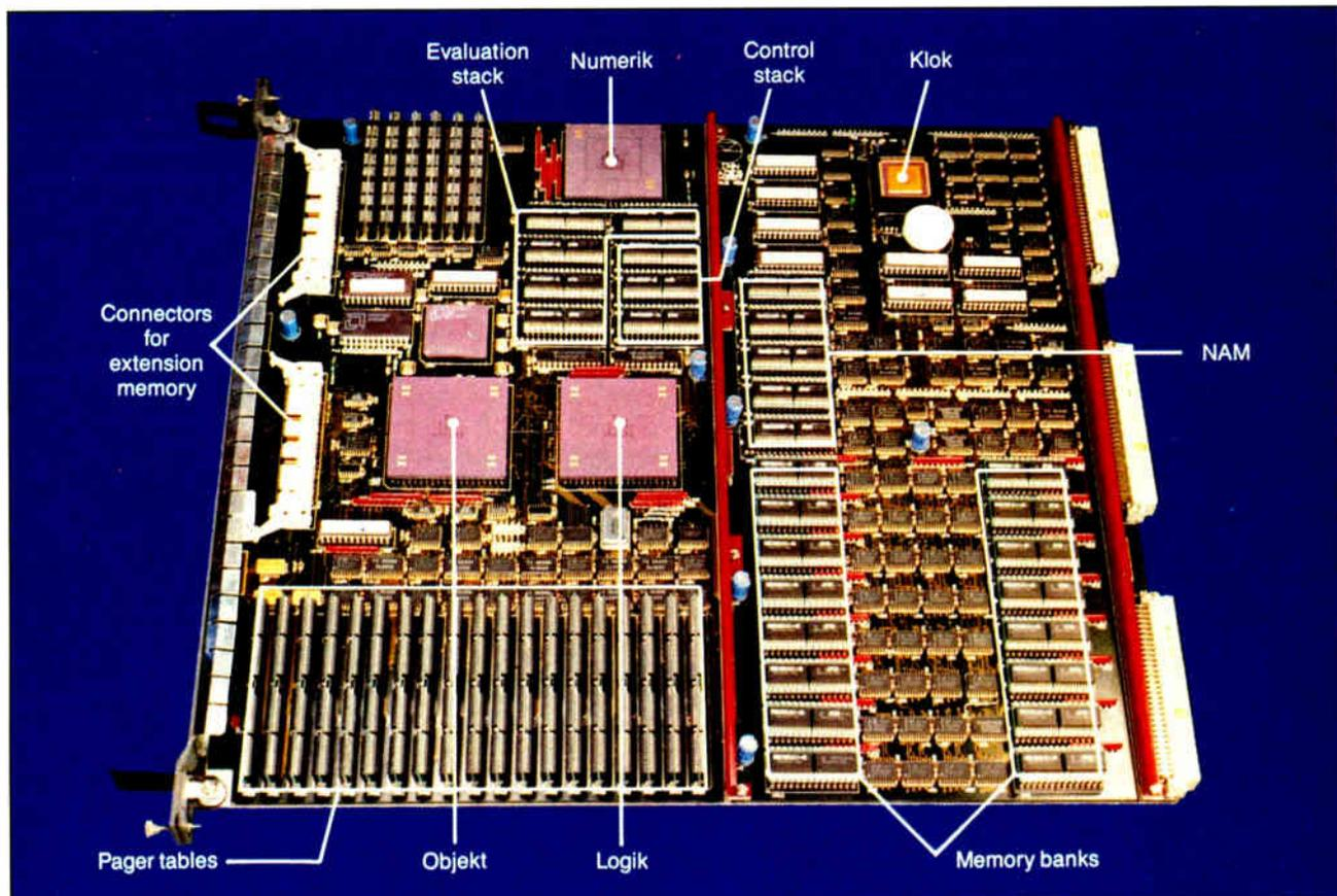
**Photo 1:** This VME board, called HADES, is the first working Rekursiv system. The main units are three gate arrays called Numerik (the ALU), Logik (the sequencer/stack unit), and Objekt (the object memory manager).
