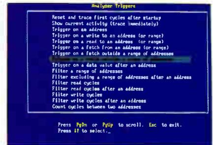
**Analyzer Triggers.** Commonly used triggers can be selected quickly from a list of standard and user-defined triggers.
