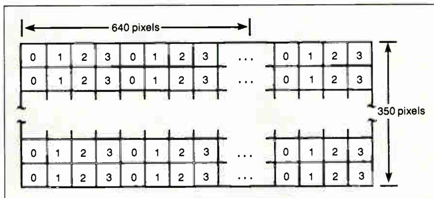
**Figure 5:** Assigning pixels to processors. If you're running a four-processor engine, the control program assigns pixels to successive processors by moving through the screen buffer horizontally left to right, then down.
