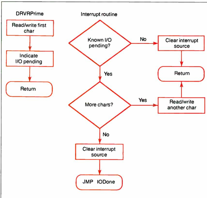
Figure 4: Flowchart illustrating read- and write-completion logic.
