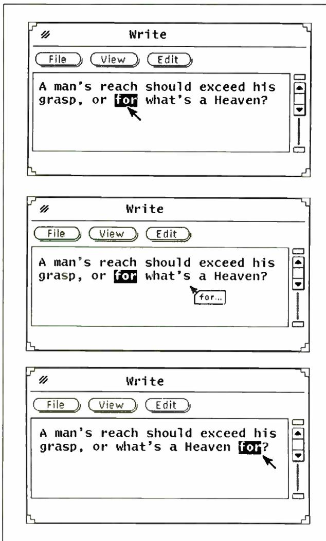
**Figure 5:** While earlier graphical interfaces pioneered the direct manipulation of graphics objects, Open Look extends this, allowing you to select and drag arbitrary pieces of text as well.
