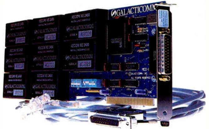
Our multi-modem PC cards are available in several configurations: 2 to 8 modems per card at 2400 baud, or 2 to 16 modems per card at 1200 baud. These are true single-slot cards with the modems built right in — no additional serial ports, power supplies, or external boxes of any kind are required.
