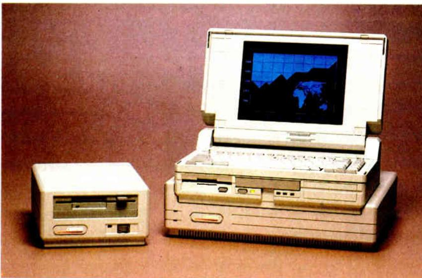
**Photo 1:** At the office, the Compaq 286 SLT can be placed in its optional Desktop Expansion Base, which contains two standard expansion slots. At the left is another option, a 5¼-inch external floppy disk drive.
