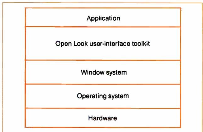
**Figure 6:** Toolkits for the Open Look user interface will allow software developers to develop applications for a variety of windowing systems running on widely disparate hardware and operating systems. The first toolkits available will be for Unix systems.
