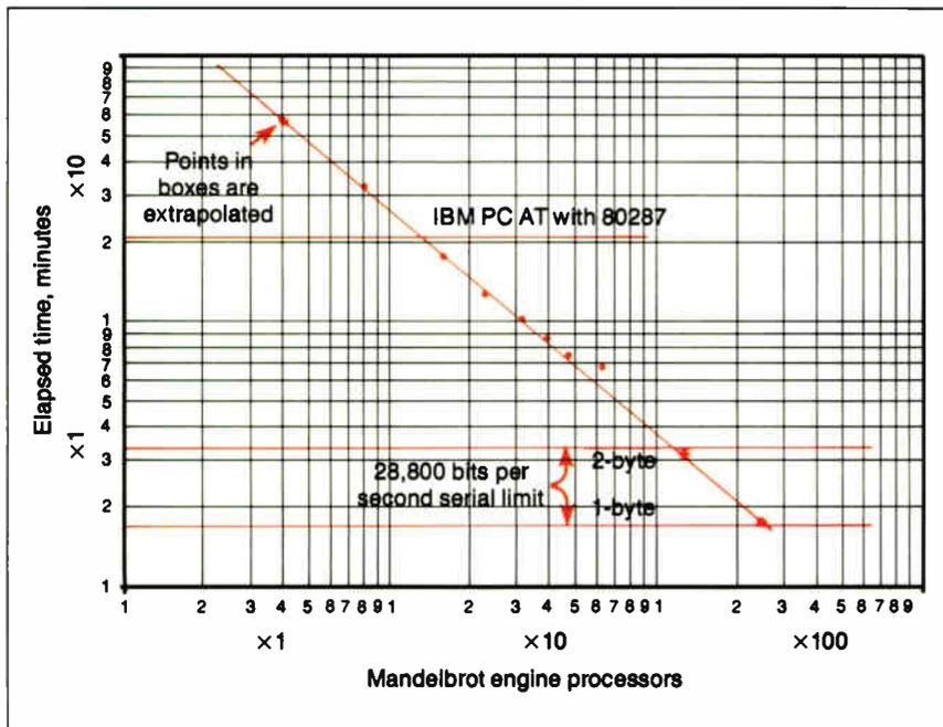
**Figure 7:** The log-log plot of elapsed time to calculate a given portion of the set versus number of processors. Also shown is the time for an AT to plot the same image.
