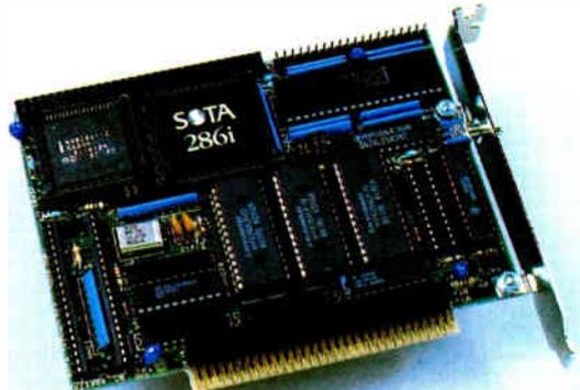
What's going on here is the 286i running the programs with no wait states on most read and write cycles.
