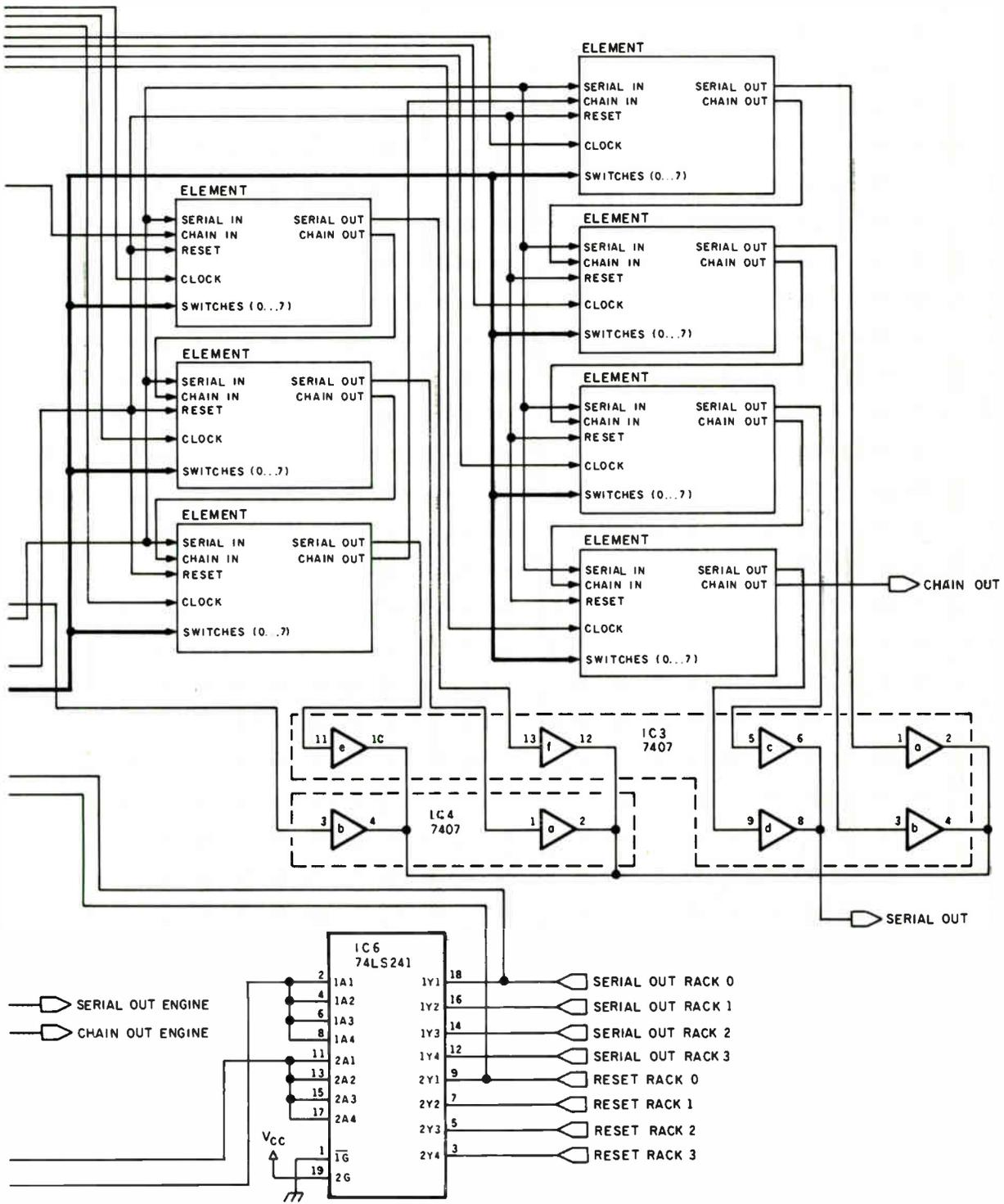
Each card has a single serial output line from all the processors on the card. All eight outputs in a rack are connected in common, so 64 open collector gates are tied together. Because I didn't think connecting 256 gates in four racks together made much sense, the Array Master card has a 74LS21 gate to combine the four signals into one. Remember that only one 8751 will be transmitting data on the serial line at a time, so only one of the 256 gates will be active.
