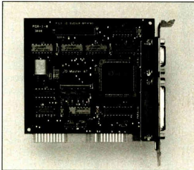
*Boca Research's IOAT41 in a 25-pin/9-pin configuration.*
