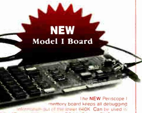
The **NEW** Periscope I memory board keeps all debugging information out of the lower 640K. Can be used in PC, AT, and 386 with both EGA/VGA and EMS boards installed. The Periscope break-out switch enables you to recover from a hung system. Included with Models I, II, and III.
