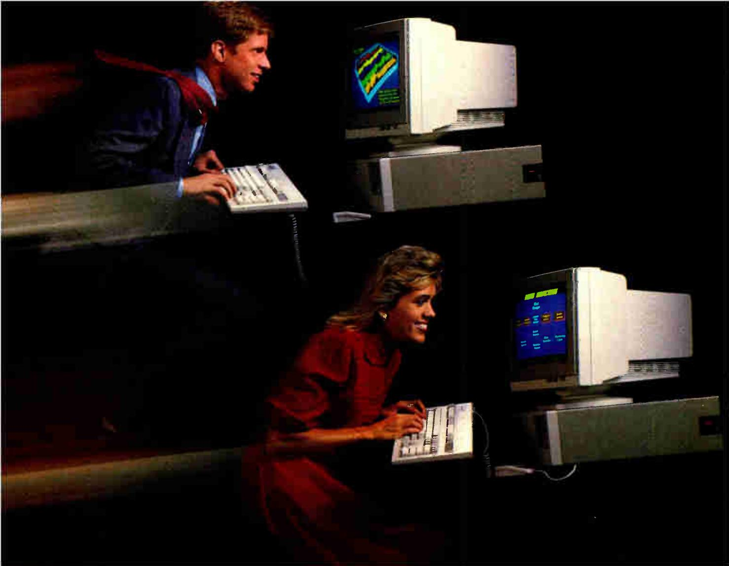
**The 386/20.** It's made for those who want to fly to the outer limits. With an Intel 80386 micro-processor operating at 20 MHz (with zero wait states) it'll move through the most complex applications with astounding ease. And you won't have to worry about running low on memory either. It not only features 1024KB of RAM and a 1.2MB floppy disk drive, it also has a 64KB cache memory. Naturally, it comes equipped with serial/parallel/game ports and a 101-key keyboard, too.
