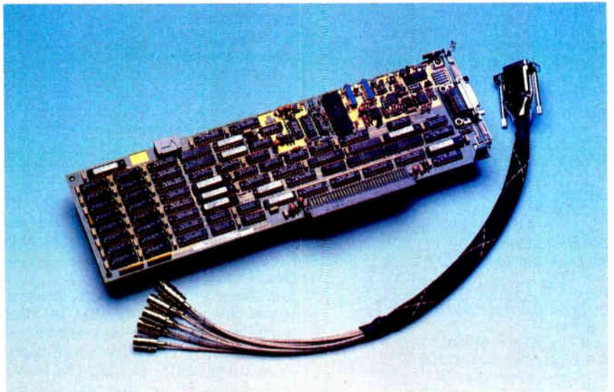
**A** new generation of devices for the Macintosh promises to do for data input what the Laser-Writer did for output. One such product is Data Translation's QuickCapture package (\$1139), consisting of a video digitizer board (or "frame grabber") and software for the Mac II.
