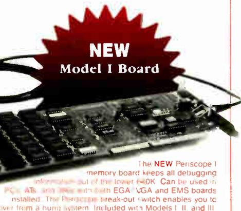
The **NEW** Periscope I memory board keeps all debugging information out of the lower 640K. Can be used in PC, AT, and 386 with both EGA/VGA and EMS boards installed. The Periscope break-out switch enables you to recover from a hung system. Included with Models I, II, and III.
