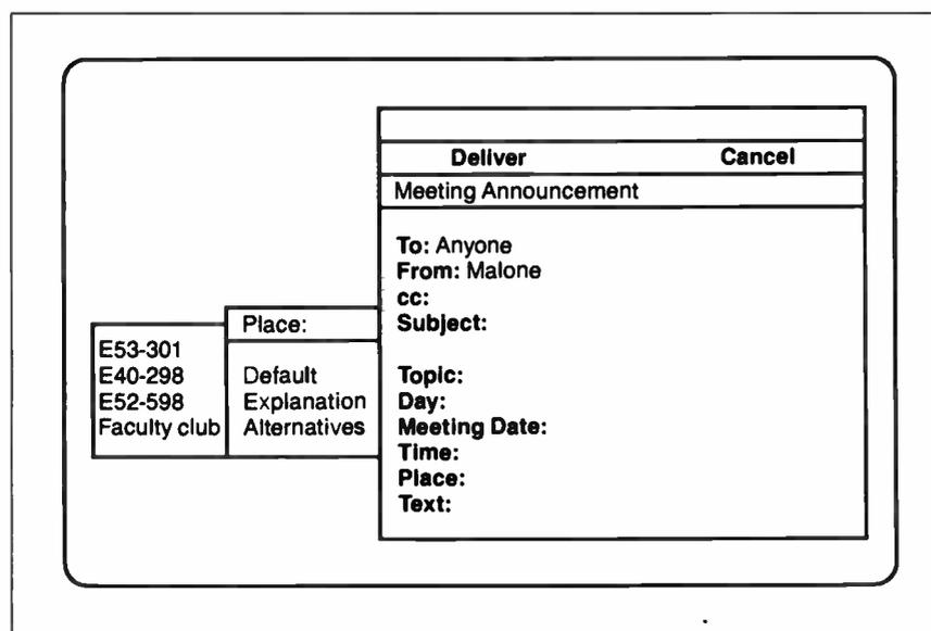
Figure 1: The format of the message screen from the Information Lens. Messages are composed with a display-oriented editor and templates that have pop-up menus associated with the template fields.
