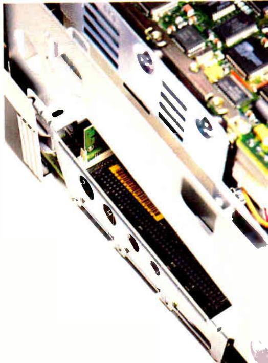
**Photo 2b:** The expansion board mounts vertically in the chassis. In the original Mac SE, the expansion board mounted horizontally under the main logic board.
