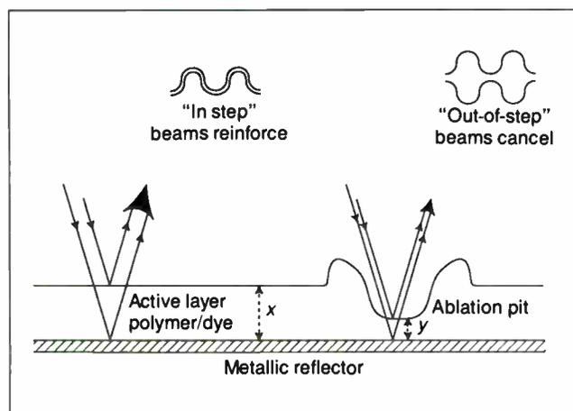
**Figure 2:** Optical data is encoded on digital paper by burning pits in the active dye/polymer layer. Here,  $x$  is a whole number of half-wavelengths of the laser light, while  $y$  is not. The pits alter the path length that light from the read laser must traverse, thereby weakening the reflected beam.
