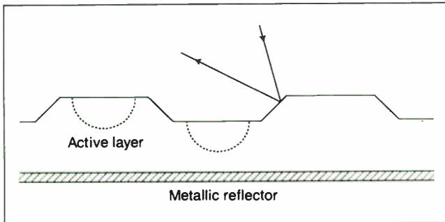
**Figure 3:** To enable the read laser to track accurately, digital paper must be preformatted, which is done by embossing grooves into the active layer. The flanks of these grooves deflect the straying laser beam and so cause a detectable error signal that is fed back in a servo loop to realign the beam.
