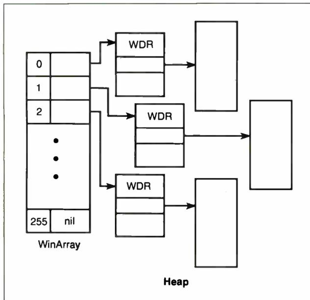
**Figure 1:** The structure of the window information consists of a 256-element array of pointers. When a window is defined, the array element points to the window structure, which in turn includes a pointer to a block of memory (heap) that holds either the screen data that is obscured by the window or the screen of a hidden window.
