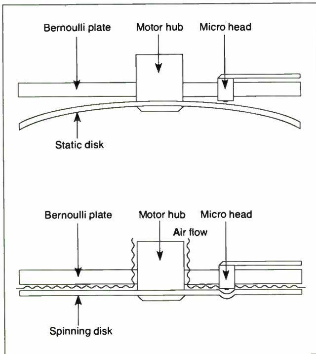
**Figure 4:** The Bernoulli effect produces lift when air flows faster over the upper surface of the disk than under it. The lift makes the disk "fly" at a close and constant distance from the Bernoulli plate and record head, a feature that is very advantageous for optical recording.
