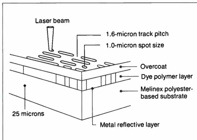
**Figure 1 :** Digital paper is a flexible optical recording medium made from a "sandwich" of thin polymer films. This cross section shows the various functional layers and the approximate dimensions.
