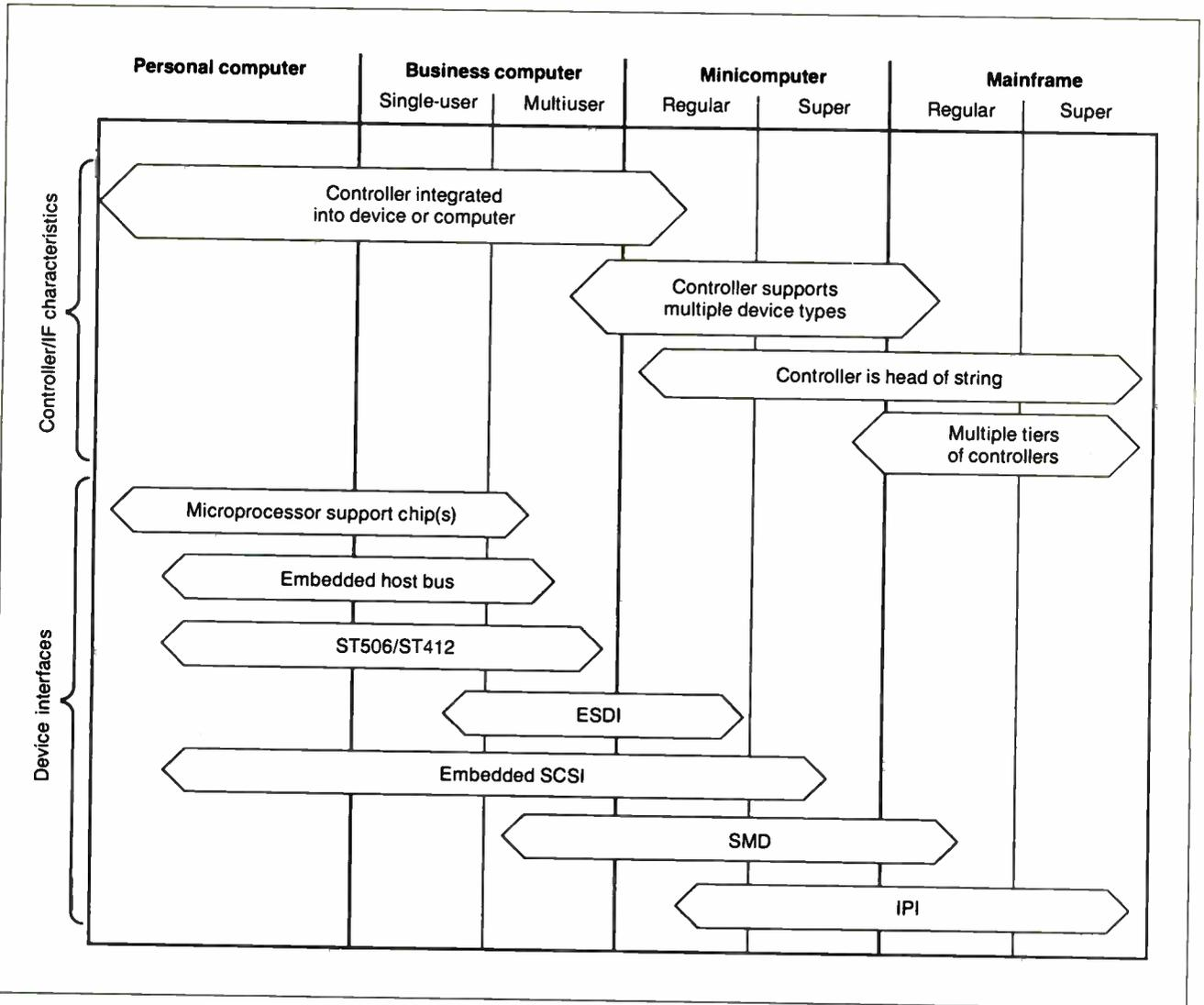
**Figure 1:** The solution regarding which hard disk drive interface is best suited to your computer depends on your machine's complexity and performance. (Figure courtesy of ENDL Consulting. Used with permission.)
