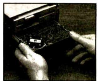
Next, you install the 5¼" floppy disk drive, learning disk drive operation and adjustment. You later improve your data storage capacity dramatically by installing a powerful 20 meg hard drive.
