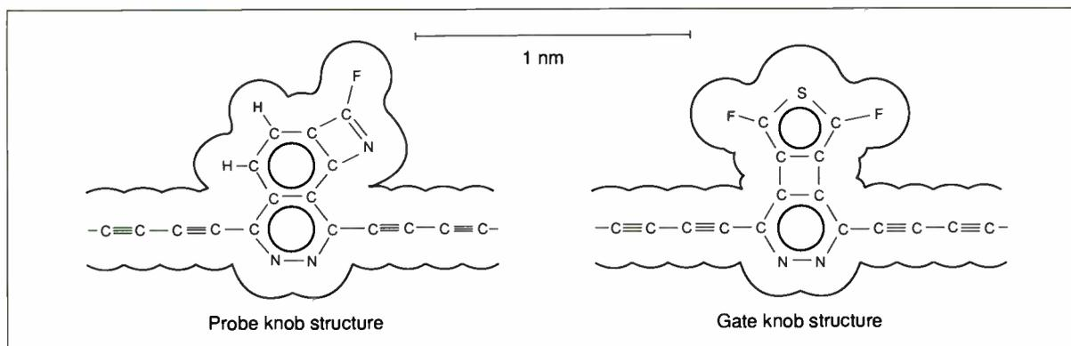
**Figure A:** The rods are atoms of carbon strung end-to-end. The knobs are specifically designed not to interact with each other. (Source: K. Eric Drexler, Foresight Institute, Palo Alto, CA)
