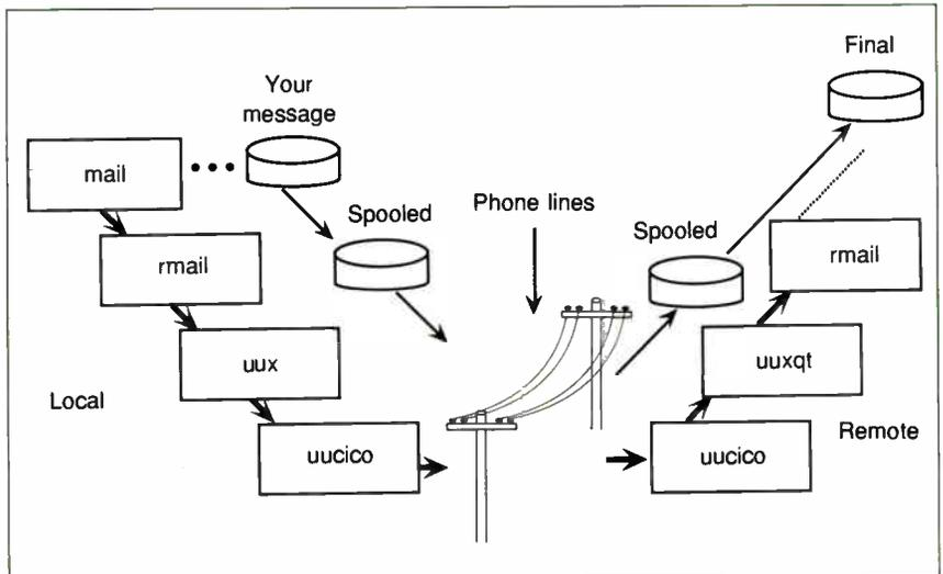
**Figure 3:** How mail is delivered to remote sites. UUCP recognizes when the mail recipient is on another system. Instead of putting the mail-delivery request in the local mail spooler, UUCP passes it to uux to deliver at the remote site with rmail.
