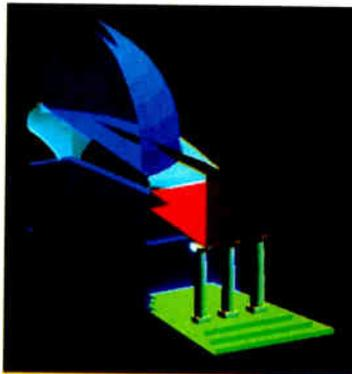
to build the pendentives. First, we established a 90-degree arc at the base of the dome—actually, a *shape* made of two arcs joined at the endpoints—so we could model the dome with thickness. Then we set a point directly above the corner of the building at the same elevation as the base of the dome. With the system's scaling factor set to 0.8 and that point as a reference, we repeatedly executed the PROJECT SURFACE command.
