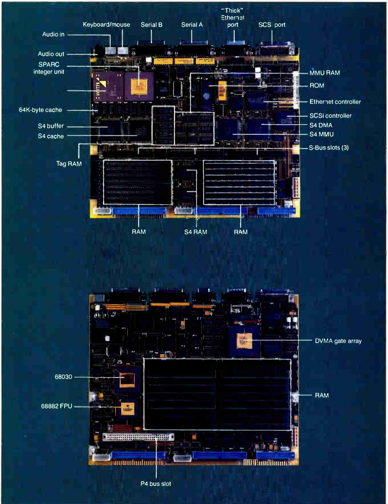
**Photo 2:** The logic boards for (a) the SPARCStation 1 and (b) the Sun-3/80. The SPARCStation board has three S-Bus expansion slots, versus the single P4 bus slot on the 3/80 logic board. Note the S4 DMA controller, which controls the DMA of the SCSI, Ethernet, and serial ports to the S-Bus. The SPARCStation board also features a 20-MHz SPARC CPU and custom FPU. The 3/80 features the 20-MHz 68030 and 68882 FPU.
