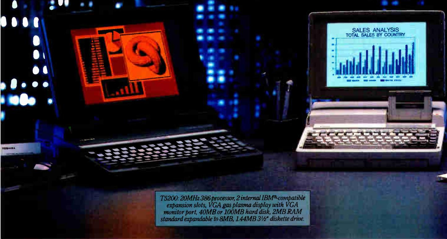
*T5200: 20MHz 386 processor, 2 internal IBM<sup>®</sup> compatible expansion slots, VGA gas plasma display with VGA monitor port, 40MB or 100MB hard disk, 2MB RAM standard expandable to 8MB, 1.44MB 3½" diskette drive.*
