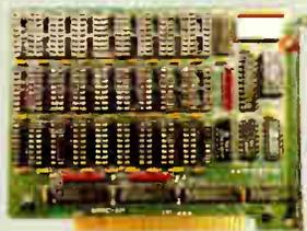
• Expands your system to the maximum 640K (zero-K on-board) • Accepts either 64K memory chips (4164) or 256K chips (41256) • Eight possible memory configurations ranging from 64K to 576K • Fits any slot (except slot 8 on IBM XT) • Recommended for systems running at 4.77MHz • Manual included
