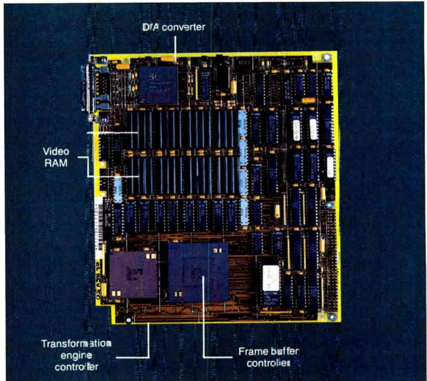
**Photo 3:** The GX graphics accelerator card. Note the two gate arrays on the lower left side of the board. The left chip is the coordinate transformation engine. The right one is the frame buffer controller.
