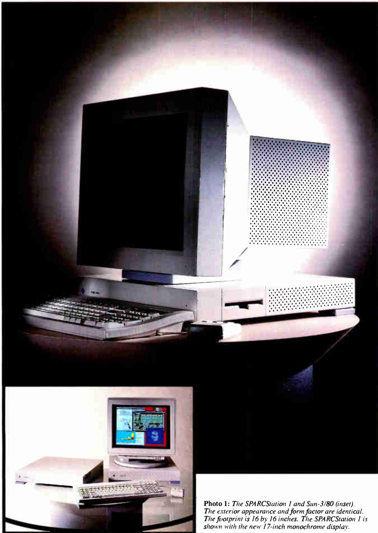
**Photo 1:** *The SPARCStation 1 and Sun-3/80 (inset). The exterior appearance and form factor are identical. The footprint is 16 by 16 inches. The SPARCStation 1 is shown with the new 17-inch monochrome display.*
