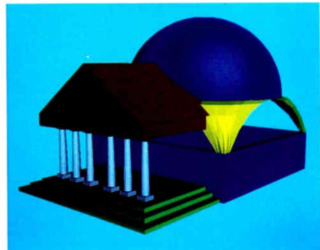
We succeeded in rendering simple entities, but because Solids Synthesis is picky about the geometry you ask it to analyze (e.g., every entity must help to define a closed surface), we bogged down trying to create a pantheon rendering.
