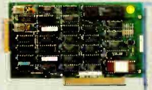
• The JE1043 allows connection of one or two 360KB, 720KB, 1.2MB or 1.44MB floppy disk drives • The JE1049 allows connection of up to four 360KB, 720KB, 1.2MB or 1.44MB floppy disk drives • JE1049 only: To add two external drives use cable Part No. ECC to add two internal drives use cable Part No. TDC • Both units include cable for two internal disk drives and manual
