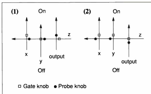
**Figure B:** (1) Schematic of a rod logic NAND gate. As long as the gate knob on either the x or y input blocks the intersection, the output rod is free to slide. (2) If x and y are both on, rod z is free to slide, blocking the output rod.
