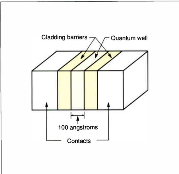
**Figure 1:** The underlying principle crucial to the development of the quantum transistor is the quantum well, created by sandwiching an ultrathin film between two walls of a second semiconductor material.
