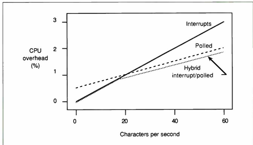
**Figure 2: Comparison of device and driver performance for interrupts, polling, and hybrid interrupt/polling.**
