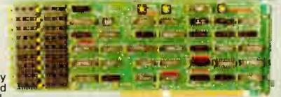
• 2MB (zero-K on board) memory expansion cards for the IBM AT and compatible computers • JE1081 utilizes (7) 41256-120ns chips to reach 2MB • JE1083 utilizes (18) 511000P-10 chips to reach 2MB (JE1083 requires full 2MB for operation) • LIM EMS 4.0 drivers • Both cards offer conventional, expanded and extended memory capabilities • Auto-parity check • RAM disk and Print Spooler software included • Manual included
