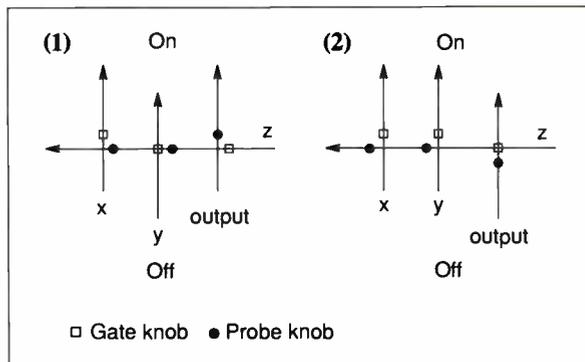
**Figure B:** (1) Schematic of a rod logic NAND gate. As long as the gate knob on either the x or y input blocks the intersection, the output rod is free to slide. (2) If x and y are both on, rod z is free to slide, blocking the output rod.
