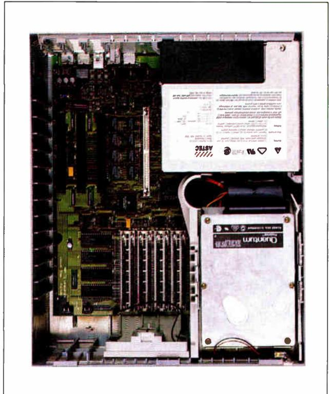
**Photo 2:** An overhead view of the internals of the Mac IICx. The cover snaps off at the rear, allowing easy access to the components inside. The entire machine can be disassembled in a few minutes. Notice the three NuBus slots at the upper left.
