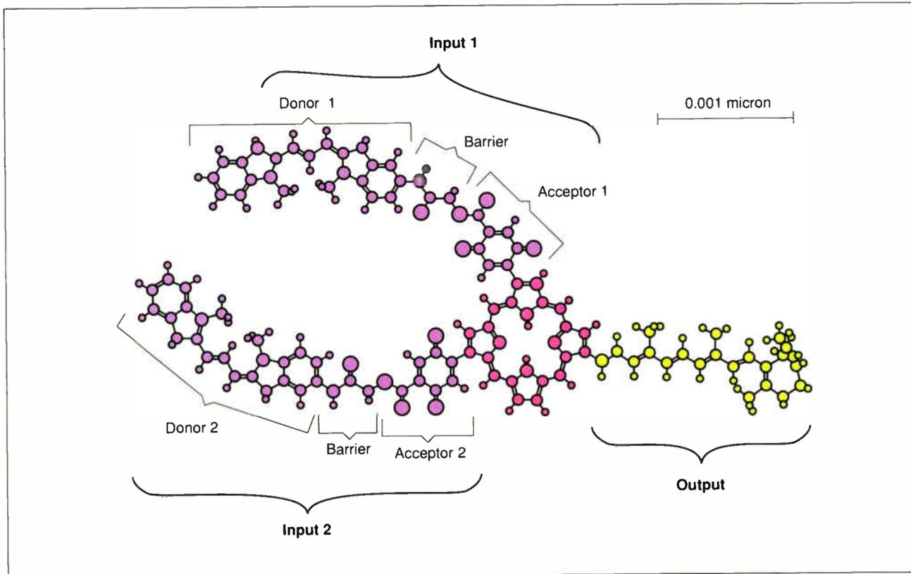
**Figure 1:** A molecular NAND gate, driven by laser light. It is four-billionths of a meter across and 10,000 times faster than similar silicon gates. (Source: Center for Molecular Electronics, Syracuse University, Syracuse, NY)
