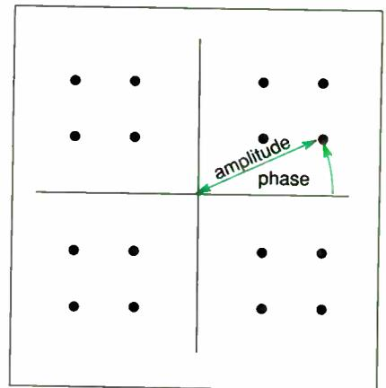
**Figure 3:** A Quadrature Amplitude Modulation constellation. Each point in the graph of a 16-point constellation represents a phase-amplitude state that the encoding scheme uses. CCITT V.22 bis uses a 16-point constellation.
