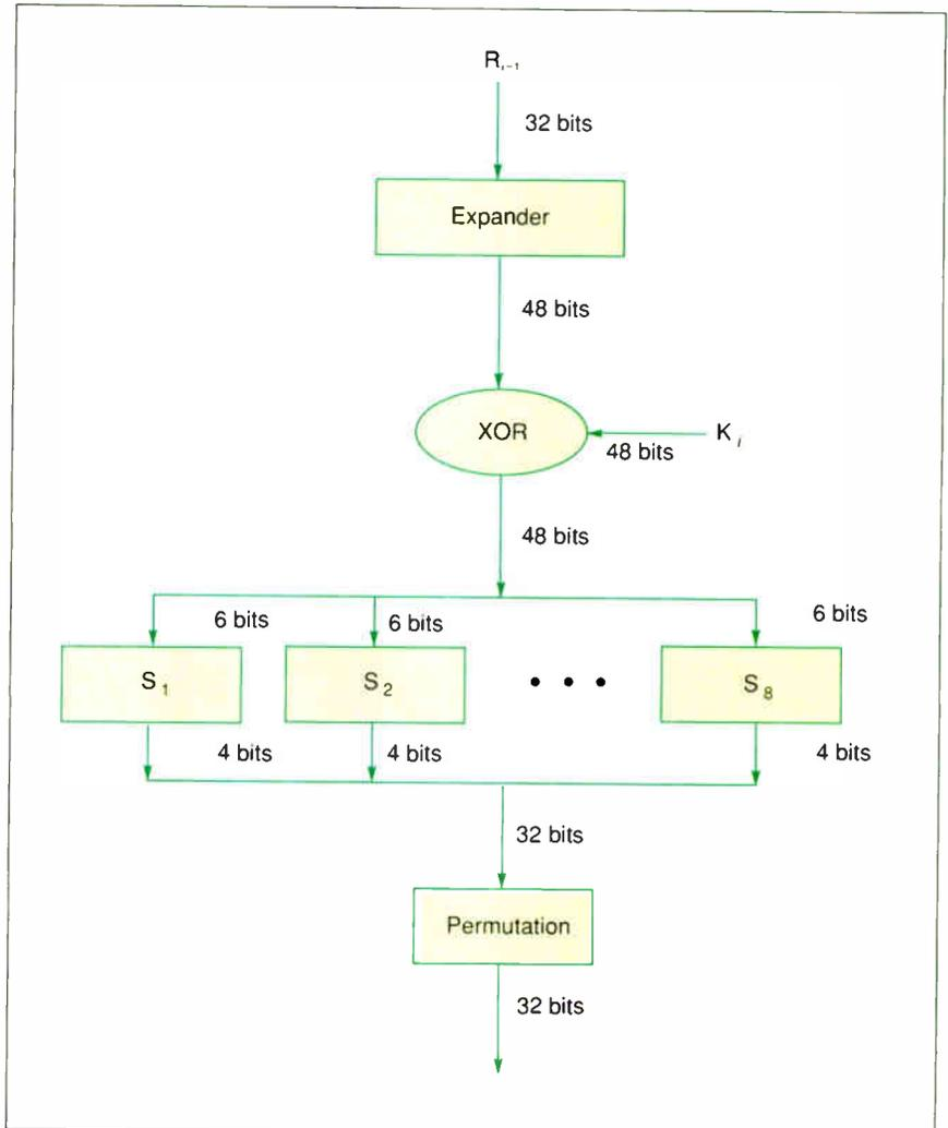
**Figure 4:** Cipherfunction  $f$  from figure 3. Its output comes from the old R part ( $R_{i-1}$ ) and the current key ( $K_i$ ). The inputs use eight S boxes to perform substitution and then permute their combined output to give the function's output.
