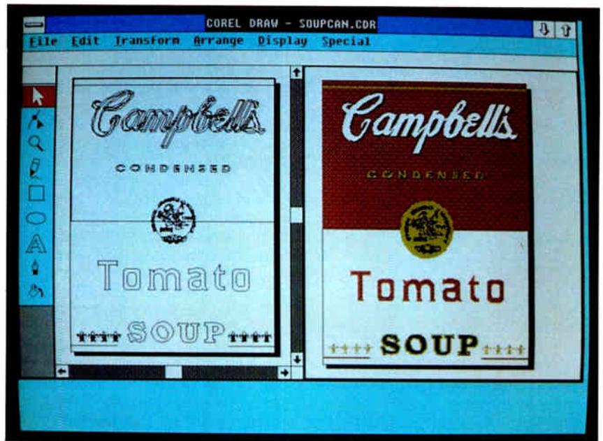
great versatility. Corel Draw has no rounded rectangle tool because you create rounded rectangles by pushing on one corner of a rectangle with the shape tool. It has no separate arc or wedge tools because the shape tool creates them from ellipses.
