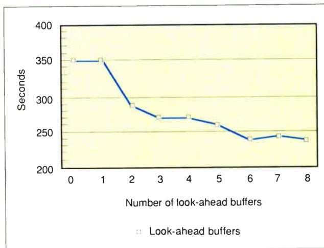
**Figure 3:** The performance improvements from using look-ahead buffers with 12,800 sequential-sector reads and writes on a 256K-byte file.
