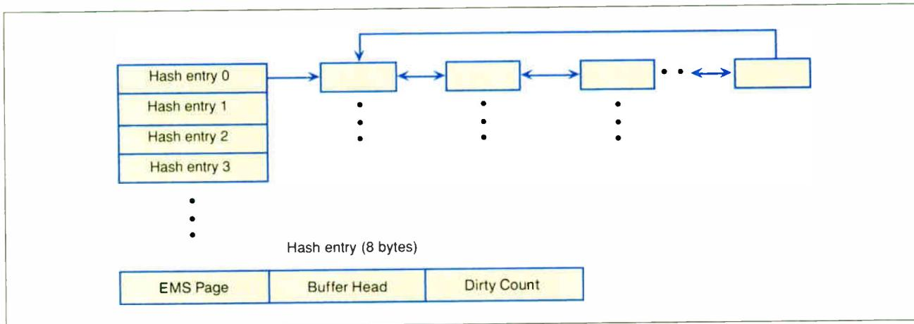
**Figure 1:** The structure of the information for large buffers consists of a hash table (in conventional memory). Each 8-byte entry in the table contains an extended-memory page number and a doubleword segment offset (address) of the first buffer in the list of 15 buffers that reside in the expanded memory. In addition, each table entry contains a Dirty Count of the number of changed buffers.
