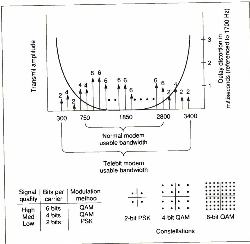
**Figure 4:** Telebit's Dynamically Adaptive Multicarrier Quadrature Amplitude Modulation encoding scheme. The Telebit Trailblazer modems use many small channels, modulated at low speeds, to make the best use of a phone line's available bandwidth. The signal quality of each 7.8-Hz channel determines what modulation scheme, if any, is used for that channel.
