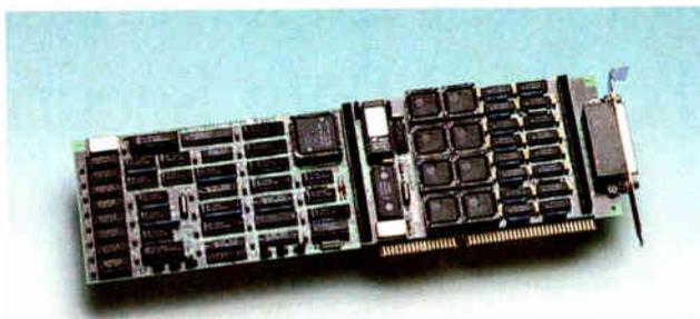
**Photo 6:** An EtherCard Plus from Western Digital (\$399) allowed us to connect to either a standard Ethernet LAN coaxial cable or a Thin Ethernet cable.
