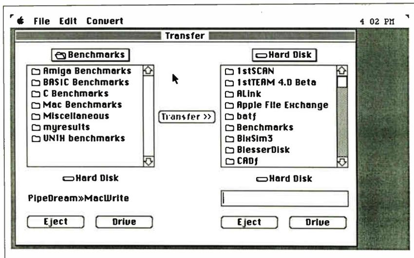
*The Link application in operation on the Mac. It manages the transfer of files between the Z88 and the Mac and provides format translation as required. It's similar in operation to the Apple File Exchange application, which handles the transfer of MS-DOS files to and from an MS-DOS floppy in the Mac's floppy disk high-density drive.*
