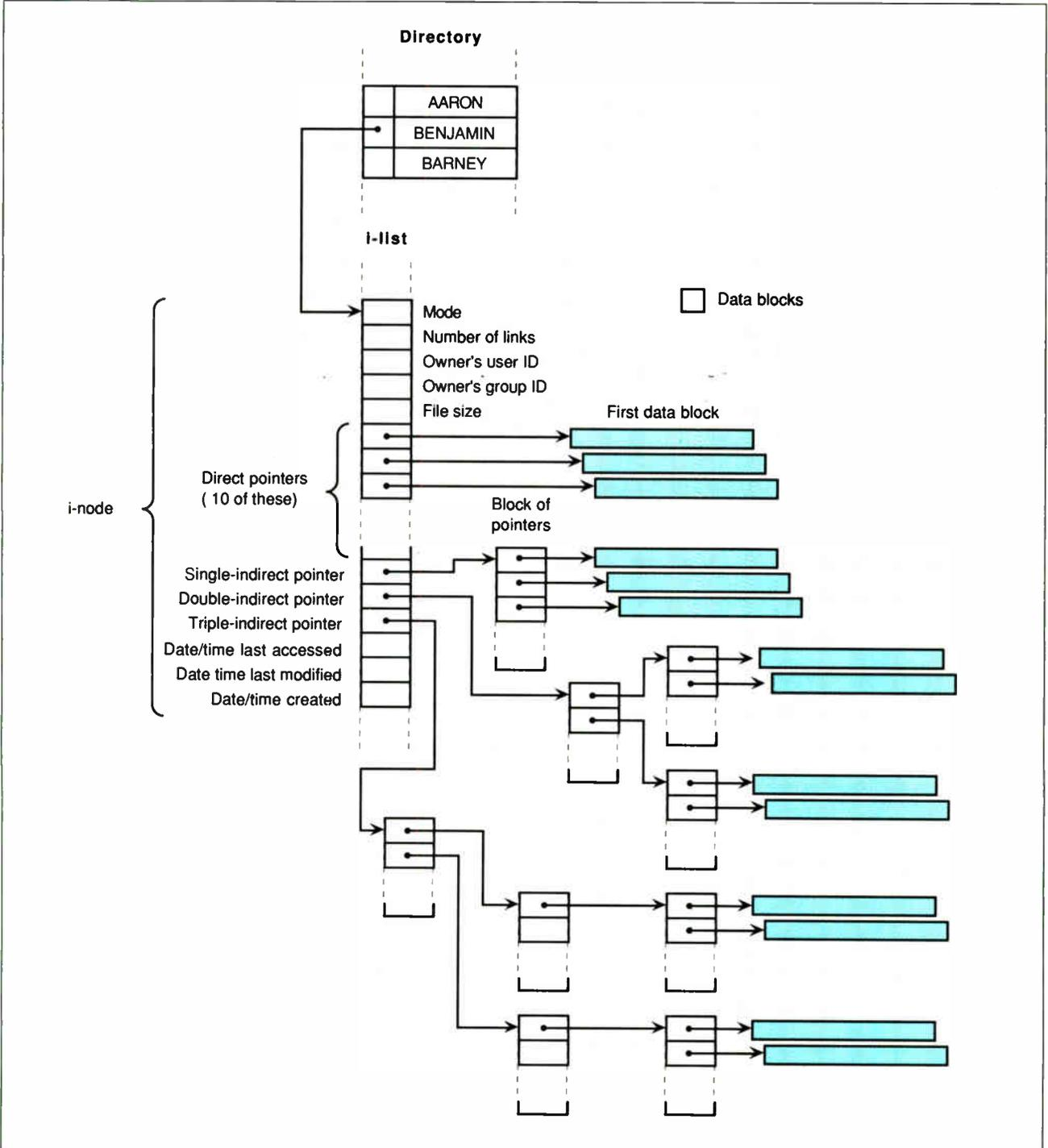
**Figure 2:** Finding the file **BENJAMIN** on the Unix system consists of searching the directory for the filename and using the associated **i-node** number to retrieve the physical location from the **i-list** structure.
