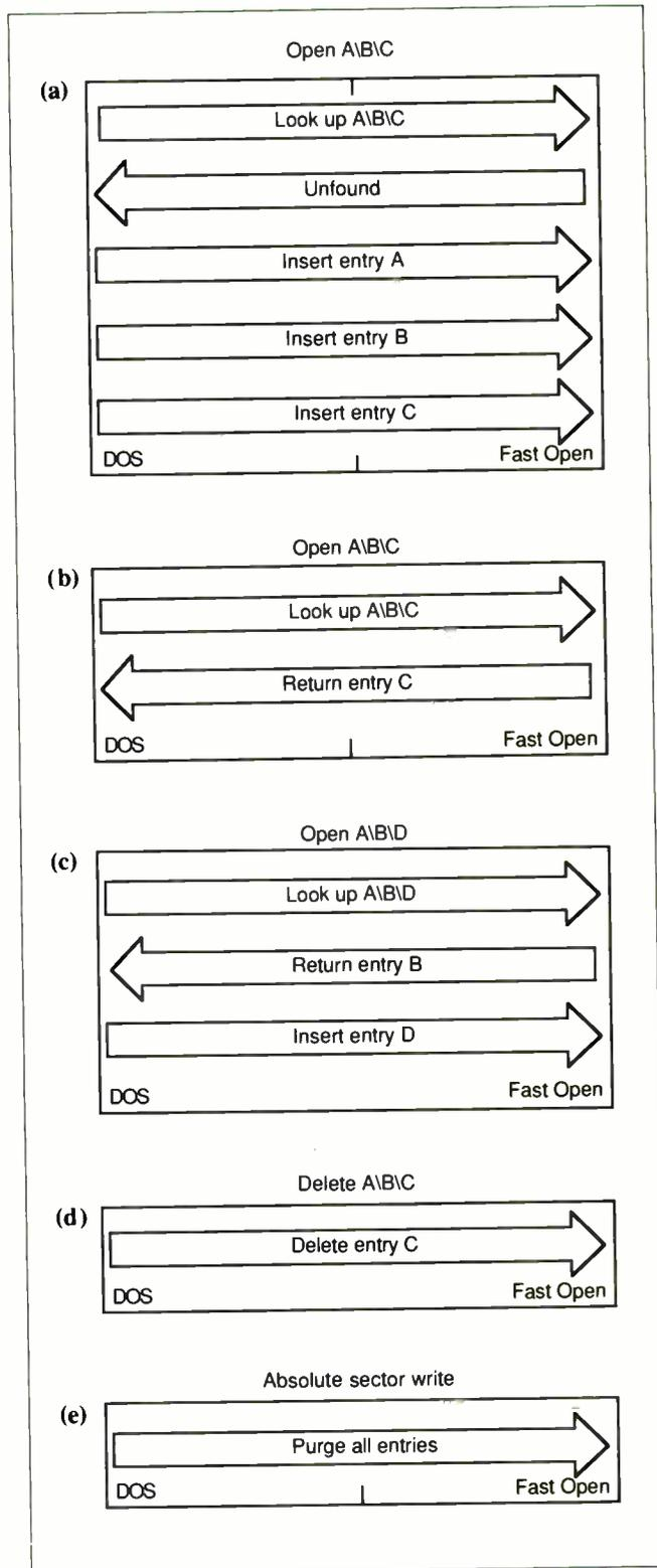
**Figure 4:** The interactions between the DOS kernel and Fast Open operations: (a) initial Lookup; (b) Lookup with complete table; (c) Lookup for a different filename; (d) deleting an entry from Fast Open table; (e) absolute sector writes, which invalidate all entries.
