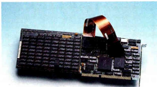
with an Inboard piggyback card. The card snaps onto the Inboard 386, allowing the processor to directly access the additional fast memory. At this writing, you are limited to 3 megabytes of 32-bit RAM with the Intel card. The Inboard will support other memory cards, such as the AST RAMpage Plus or the Intel Above Board 286, but you're back to the slower, 16-bit variety.
