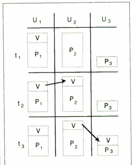
Figure 1: A picture through time of a virus infecting a system. A virus, V, infects user U<sub>1</sub>'s program P<sub>1</sub> at time t<sub>1</sub>. At t<sub>2</sub>, U<sub>1</sub> shares information with U<sub>2</sub> and infects P<sub>2</sub>. When U<sub>2</sub> shares data with U<sub>3</sub> at t<sub>3</sub>, P<sub>3</sub> becomes contaminated. (Figure courtesy of Fred Cohen)
