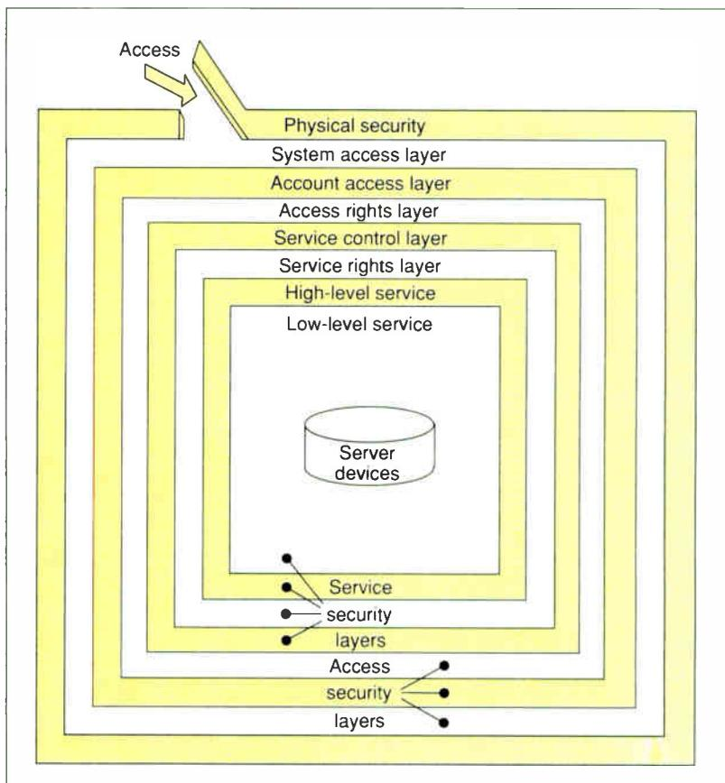
**Figure A:** Like an onion, good security is composed of layers wrapped on layers. In the file-server model, access to the actual device must go through three layers of access security and four layers of service security.
