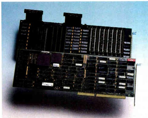
plugged in its slot. By simply loading a device driver, you can then hot-key between the two processors. Even when the 80386 takes precedence, the 80286 does not lie dormant. It acts as an intelligent controller, busily polling interrupts and passing control to its more powerful cousin. This makes the installation of the AOX board much easier than that of the Inboard.
