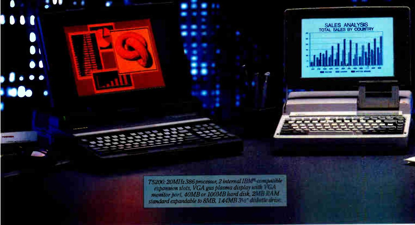
*T5200: 20MHz 386 processor, 2 internal IBM<sup>®</sup> compatible expansion slots, VGA gas plasma display with VGA monitor port, 40MB or 100MB hard disk, 2MB RAM standard expandable to 8MB, 1.44MB 3 1/2" diskette drive.*
