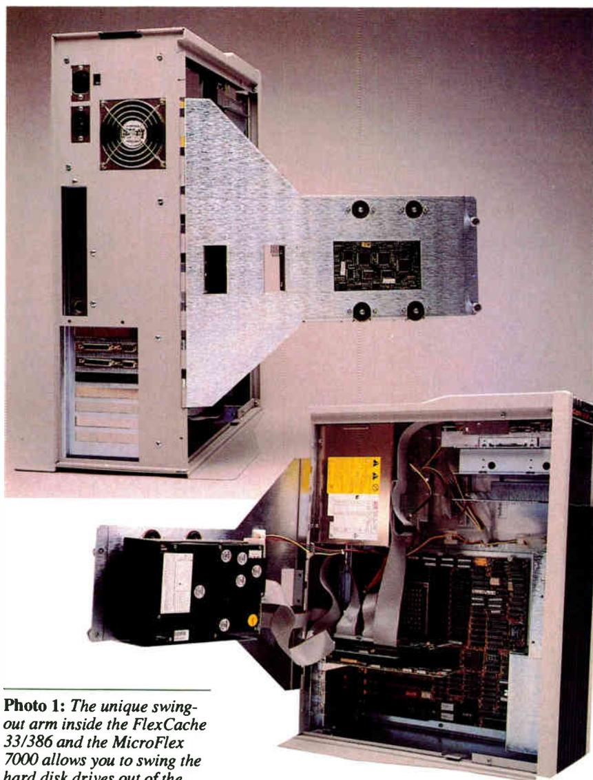
**Photo 1:** The unique swing-out arm inside the FlexCache 33/386 and the MicroFlex 7000 allows you to swing the hard disk drives out of the way to add extra memory or a math coprocessor.
