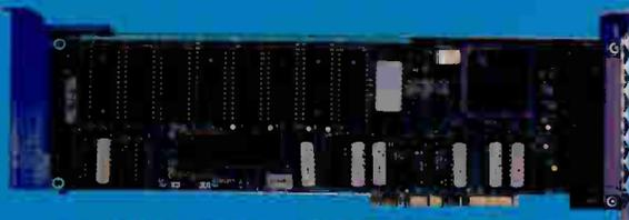
The **MCSS-9IM** is GTEK's newest intelligent card for the Micro-Channel. The **MCSS-9IM** provides up to 9 serial channels and up to 1 Megabyte of memory. The **MCSS-9IM** comes with 32K of **Dynamemory**, and is user upgradeable to 1 Megabyte.
