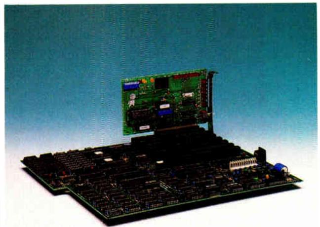
**A**ward Software's aptly named **POSTcard** is an add-in card that monitors your IBM PC during the POST (power-on self test) sequence that's run from the ROM BIOS every time you turn on your system. POSTcard has both a dual-digit LED display and a setup of 10 individual LEDs that tell you (in hexadecimal and binary, respectively) what tests are being performed. If your system locks up, it tells you exactly where the problem lies.
