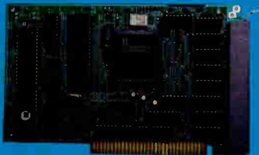
The **PCSS-8I** is GTEK's most popular intelligent serial I/O card. It provides 8 channels for PC/XT/AT/PS2-286 and is DOS Compatible. The **PCSS-8I** has 32K of **Dynamemory**, user upgradeable to 128K bytes.
