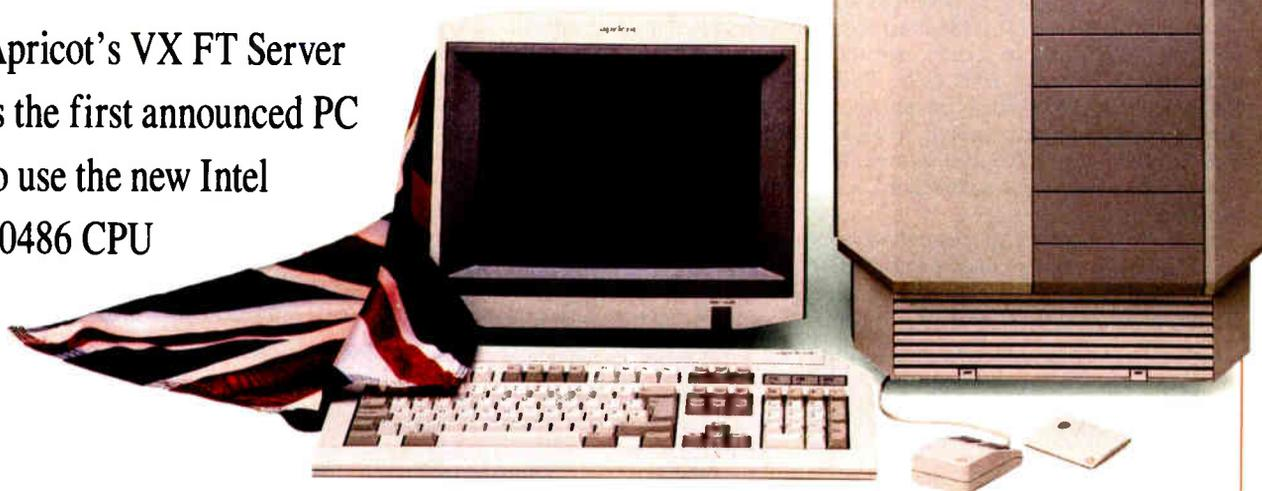
**W**hile IBM and Compaq have been loudly engaged in a one-upmanship battle over who leads the market, Britain's Apricot has quietly introduced the first PC based on Intel's 80486 CPU. Unlike IBM's recently announced 80486 Power Platform upgrade for the PS/2 Model 70, the Apricot VX FT Server, based on the Micro Channel architecture (MCA), is an entirely new system with an external RAM cache. This cache memory provides a significant performance advantage over IBM's product.
