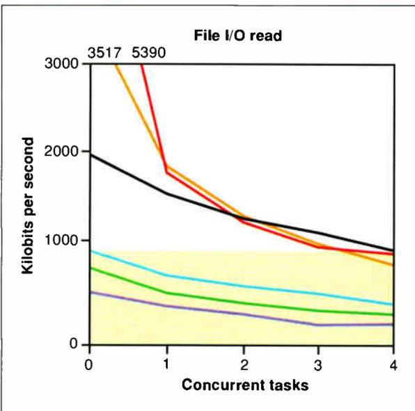
**Figure 3:** Accessing the file system. Again, PC-MOS displays strong single-user performance, but it degrades quickly.
