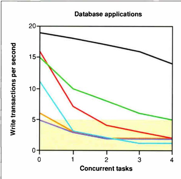
**Figure 1:** Multiuser performance on our network-based database test. The graph also depicts how much degradation you might expect from each system. PC-MOS outperforms the others when unloaded, but 386/MultiWare holds up to increasing loads.
