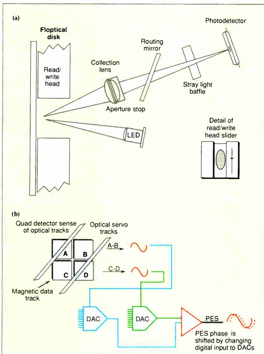
**Figure 3:** (a) The Floptical disk technology increases data density by using an optical track to generate precise tracking of the read/write head. (b) Alignment of the head to optical servo tracks is accomplished with a Phase Error Signal shift technique using multiple digital analog converters.
