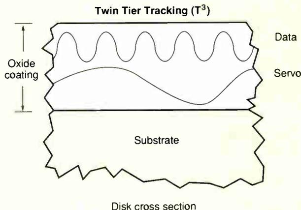
**Figure 4:** Brier's  $T^3$  (Twin Tier Tracking) Servo System uses two layers of magnetic information. The deeper layer is permanent and provides the tracking information.
