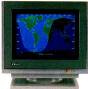
**TM5154 Specifications:** EGA/CGA compatibility • Input: DB9 (TTL) • Hor. Scanning freq.: 15.75-21.85kHz • Resolution: 720 x 350 (max.) • Bandwidth: 25MHz • Size: 15"W x 14.25"D x 14"H • Weight: 35 lbs. • One-Year Warranty
