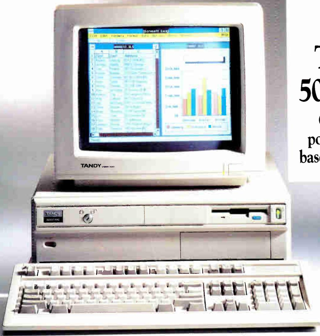
The remarkable Tandy 5000 MC Professional System is pure performance, from the Intel® 80386 processor operating at 20 MHz to the high-speed memory with cache controller that provides RAM-fast access to your data.
