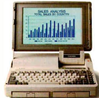
*T1600: Battery-powered 80C286/12MHz, 20MB hard disk at 27msec, 144MB 3½" diskette drive, 1MB RAM expandable to 5MB, detachable backlit EGA-compatible LCD, removable rechargeable battery pack, coprocessor socket, 7 standard interfaces, 2 expansion slots for general purpose options. For information call 1-800-457-7777. Toshiba PCs are backed by the Exceptional Care Program (enrollment required).*
