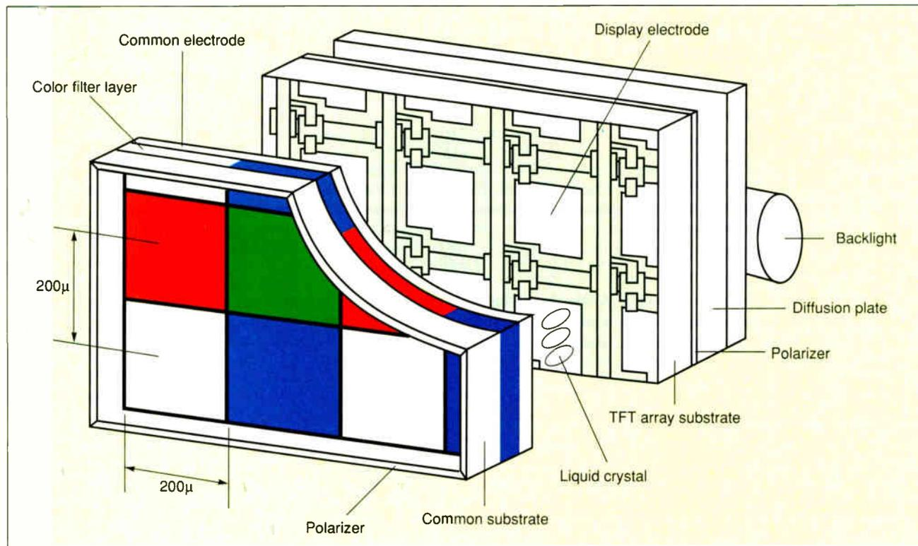
**Figure 2:** IBM and Toshiba are jointly developing a high-resolution color LCD screen. The 14-inch display contains 1.5 million color dots. Four dots (red, green, blue, and white) combine to form a single pixel. Since a dot is either completely on or completely off, there are 16 possible colors.
