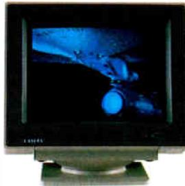
**TM5155 Specifications:** • CGA/EGA/VGA/PGC Compatibility • Input: DB9-pin (TTL) & DB15-pin (Analog) • Hor. Scanning freq.: 15.5-40kHz • Max. Resolution: 800 x 600 • Bandwidth: 40MHz • Size: 15"W x 15"D x 13.5"H • Weight: 35lbs. • One-Year Warranty
