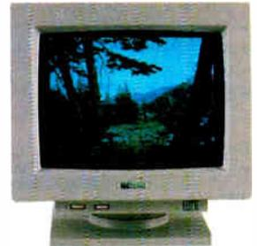
**QC1478 Specifications:** • VGA Compatibility • Non-glare, tinted display, unlimited color capability • Input: DB15-pin High Density connector (Analog) • Scanning freq.: 31.5Khz • Resolution: 720 x 480 (max.) • Bandwidth: 30MHz • Size: 14.17"W x 14.84"D x 14.25"H • Weight: 26 lbs. • One-Year Warranty
