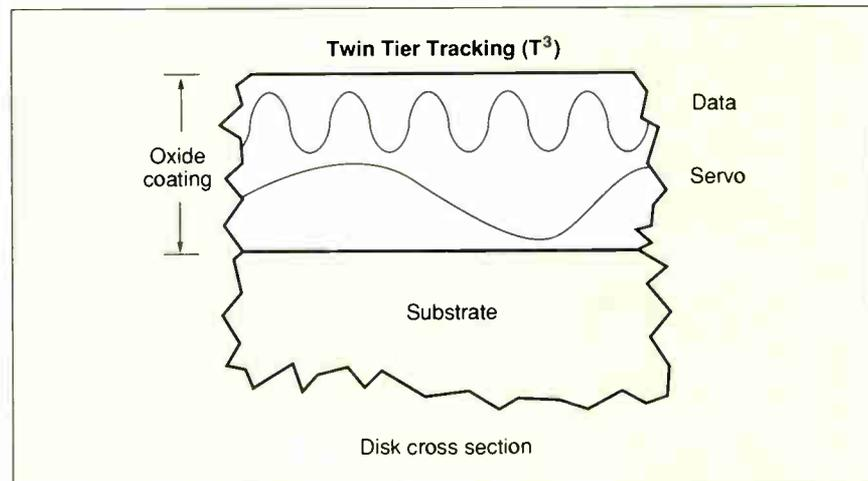
**Figure 4:** Brier's T<sup>3</sup> (Twin Tier Tracking) Servo System uses two layers of magnetic information. The deeper layer is permanent and provides the tracking information.
