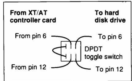
**Figure 1:** Switch-wiring diagram for write-protecting a hard disk drive.
