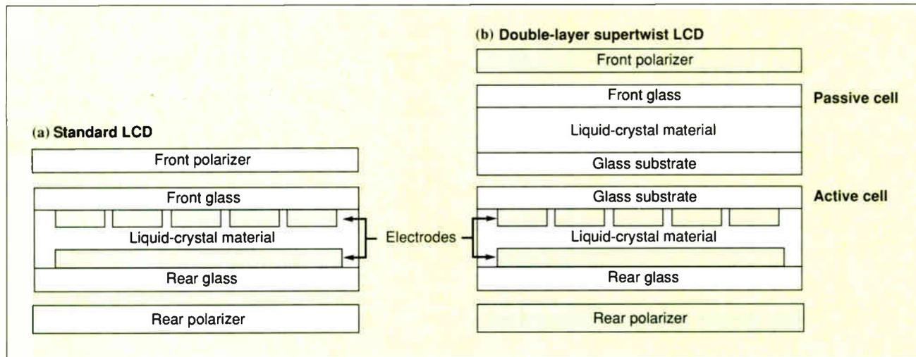
**Figure 1:** The major difference between the standard LCD (a) and the double-layer supertwist (DST) display (b) is the addition of a passive liquid-crystal layer in front of the active LCD layer. The additional layer reduces color distortion.
