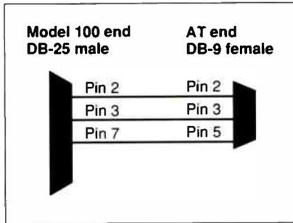
Figure 2: Diagram for a PC AT-to-Model 100 cable.
