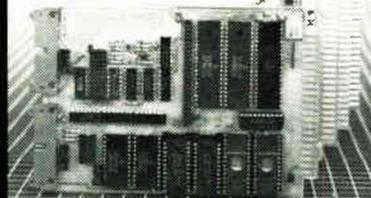
6809 MPU, 2 serial ports, 4 parallel ports, RAM, EPROM, real-time clock, watchdog timer, 44-pin 4.5" x 6.5" PCB
