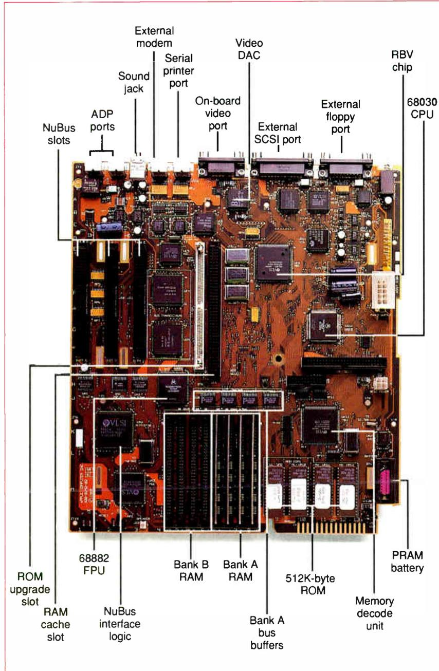
**Photo 4:** The Mac IIci motherboard. The various application-specific ICs reduce the board's component count and thus improve its reliability.
