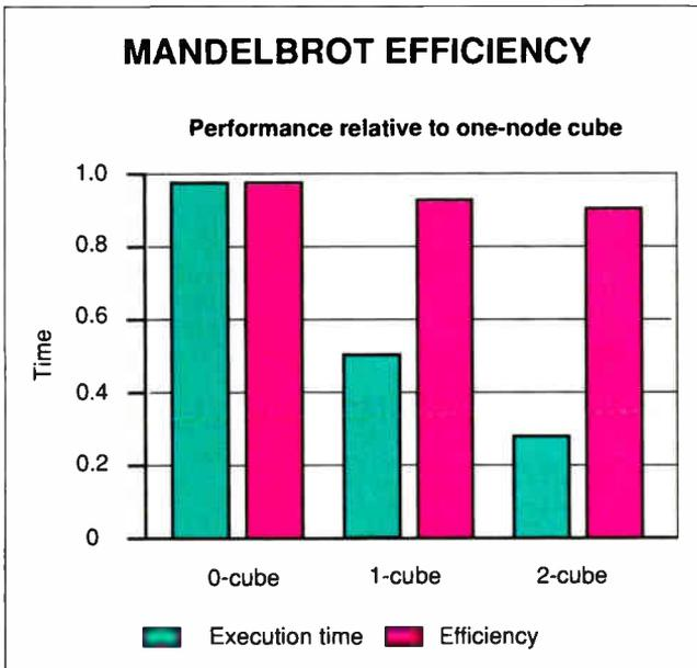
**Figure 4:** Efficiency versus execution time of a 0-, 1-, and 2-cube Mac-Cube, which translates to one, two, and four Macs, respectively. Because the communication overhead also increases as nodes are added, the efficiency declines slightly. For example, adding three more processors to a single-processor node (for a total of four) reduces execution time to a little more than one-fourth of the single processor's time.
