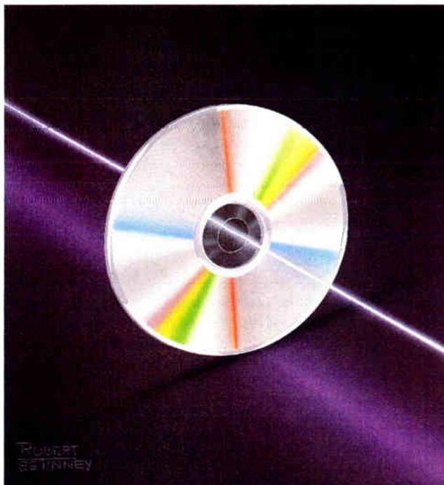
primary advantage is storage density: You can get a lot more information on an optical disk than on a comparably sized magnetic disk. Due to the precision with which a laser can be focused, recording tracks on an optical disk are much closer together than tracks on a magnetic disk. Also, the amount of space needed to record an optical bit is much smaller than that used by magnetic media.
