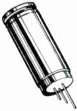
A low power collimator pen containing a MOVPE grown gain guided GaAlAs laser. This collimator pen delivers a maximum CW output power of 2.5 mW at 25 °C.
