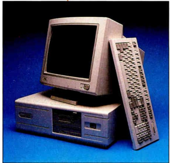
For additional memory, you must use an expansion board, which fits into a special 32-bit expansion slot. This board has room for seven 2-megabyte memory modules (at a rather hefty \$1299 each), bringing the total memory capacity up to 16 megabytes.
