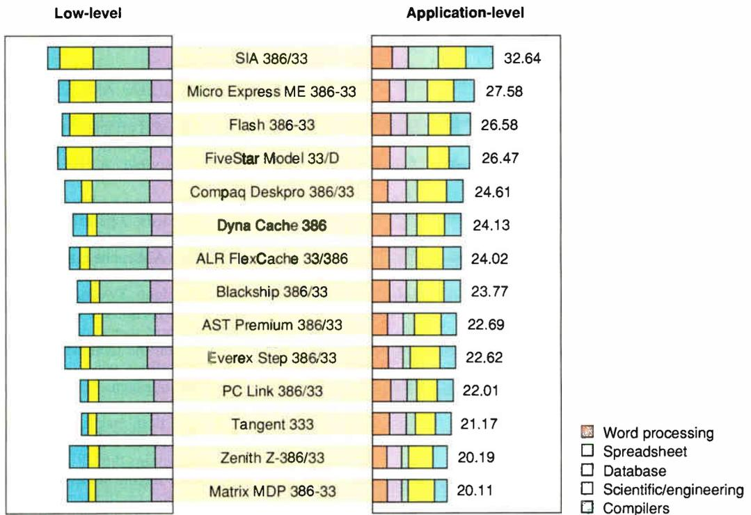
Figure 1: The systems that used the Distributed Processing Technology disk-caching controller took the top four spots on our cumulative application indexes, followed by the Compaq Deskpro. Installing a hardware disk cache in any of the other 33-MHz PCs would dramatically increase their scores, although expensively and sacrificing some hard disk capacity.
