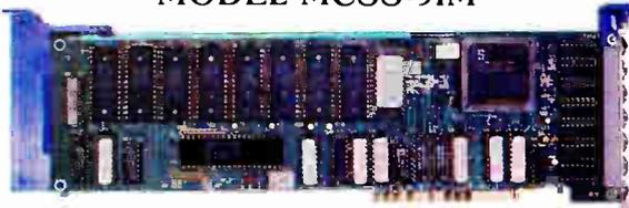
The **MCSS-9IM** is GTEK's newest intelligent card for the Micro-Channel. The **MCSS-9IM** provides 9 channels and comes with 32K of **Dynamemory** that can be upgraded to 1 Megabyte. Call for details on the **MCSS-8TX** a Micro-Channel version of the **PCSS-8TX**.
