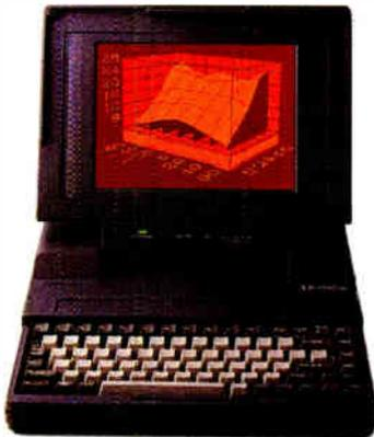
*T3100: 12MHz 80286, internal IBM slot, 20MB hard disk, gas plasma display, 1MB RAM expands to 5MB, 1.44MB 3 1/2" diskette drive.*
