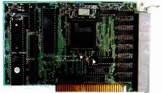
The **PCSS-8I** is GTEK's most popular intelligent serial I/O card. It provides 8 channels for PC/XT/AT/PS2-286 and is DOS Compatible. The **PCSS-8I** has 32K of **Dynamemory**, user upgradeable to 128K bytes.
