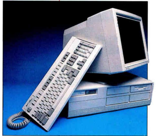
3180E ESDI hard disk drive, 3 megabytes of 80-/100-ns system RAM, 16K bytes of 15-ns SRAM for the cache, and a 200-W power supply. It also came paired with the Zenith ZCM-1490 Flat Technology 14-inch analog color monitor. The system comes with MS-DOS 3.3 Plus and Windows/386. The total price of this system is \$13,197.
