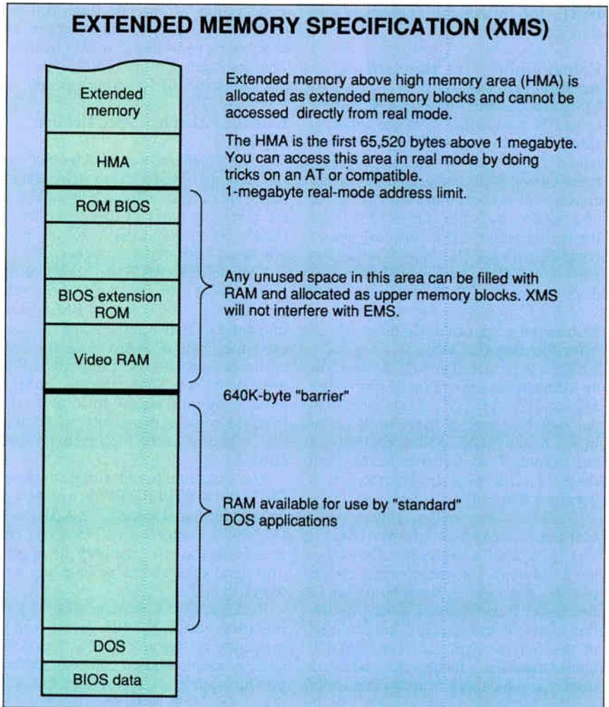
**Figure 2:** Extended memory is the area above the 1-megabyte mark on an 80286- or 80386-based PC; it's simply a linear extension of the RAM below 1 megabyte.
