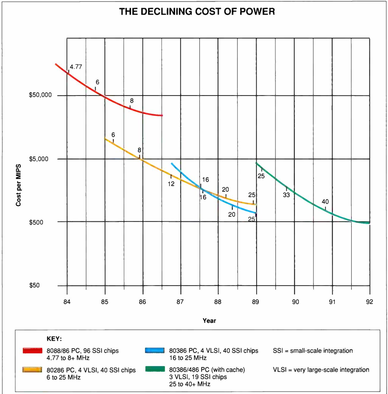
**Figure 1:** These curves represent processing power (in MHz and chip technology) and a PC time line. Succeeding generations of faster and more-complex microprocessors have married with ever-higher levels of integration to produce lower computing costs per MIPS.
