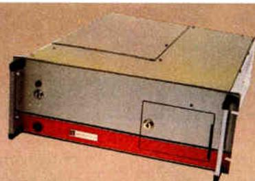
Rack mounted, rugged, 10 slot passive backplane, with 12.5 MHz 80286 CPU
