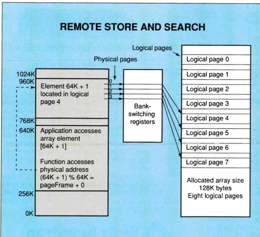
**Figure 2: A conventional memory access for element  $(64\text{K bytes} / \text{sizeof(element)} + 1)$  would have an address that points outside the physical window.**
