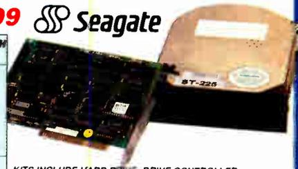
KITS INCLUDE HARD DRIVE, DRIVE CONTROLLER, CABLES AND JDR'S DETAILED INSTRUCTION MANUAL
