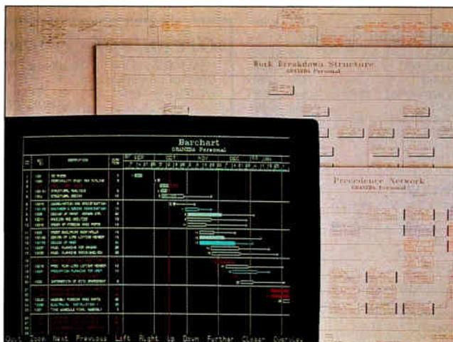
*The four types of drawings that Graneda can create include precedence network, arrow network, bar charts, and work breakdown structures.*
