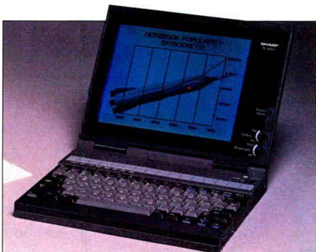
*Sharp's PC-6220 is a lightweight and low-cost notebook AT that comes complete with VGA graphics and a 2-hour battery.*
