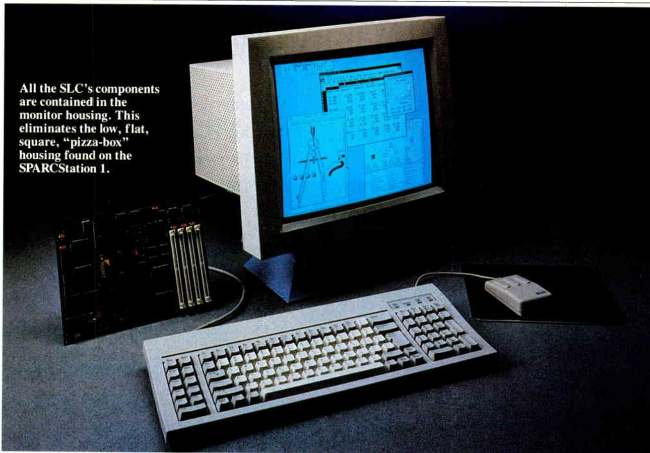
All the SLC's components are contained in the monitor housing. This eliminates the low, flat, square, "pizza-box" housing found on the SPARCStation 1.
