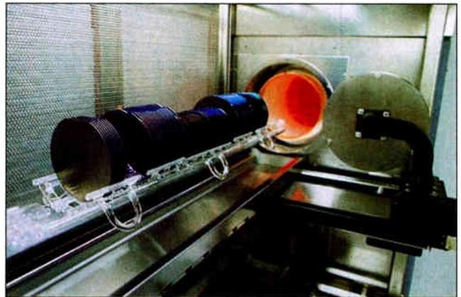
**Photo 2:** Research at the Austin, Texas, semiconductor consortium, SEMATECH, centers around ways to efficiently fabricate chips. Here, wafers are being prepared for loading into a furnace chamber.
