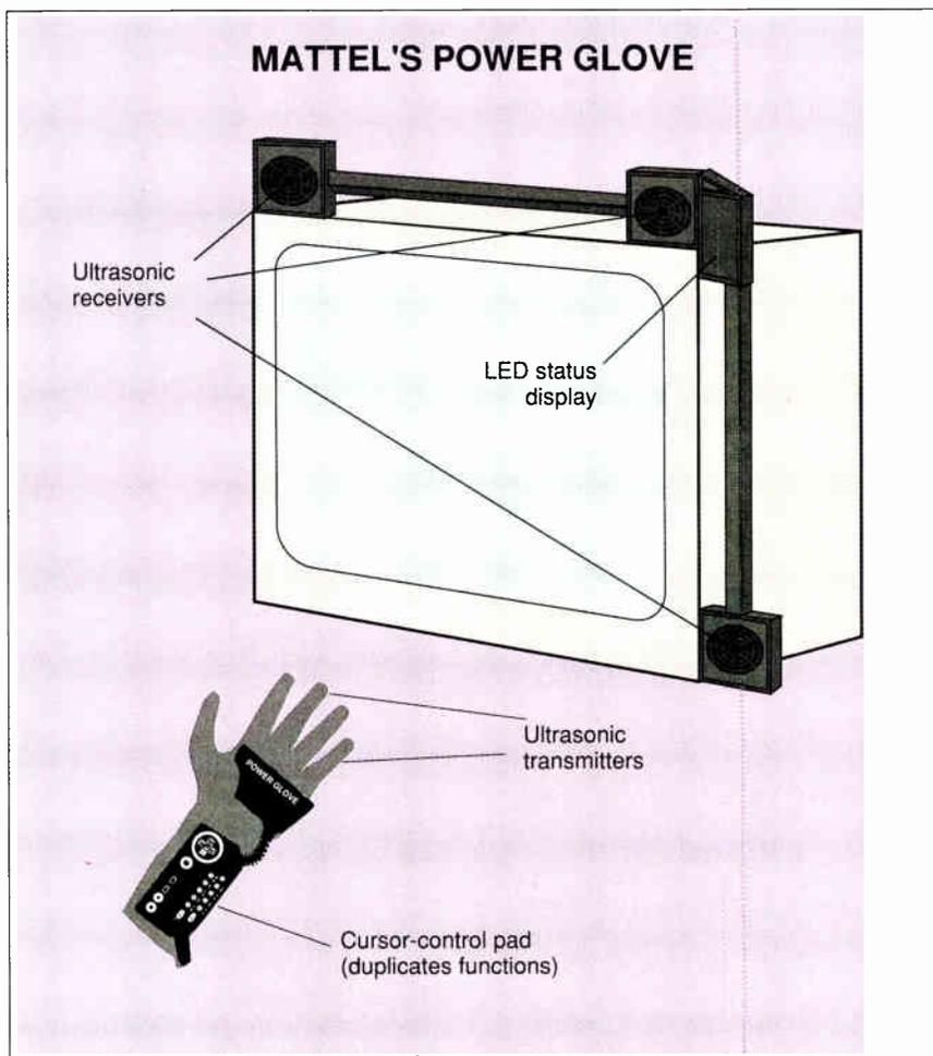
Figure 4: The Power Glove uses two ultrasonic transmitters and three receivers to triangulate the position and orientation of the hand. The cursor keypad duplicates the sensory functions and allows for somewhat more precise input.
