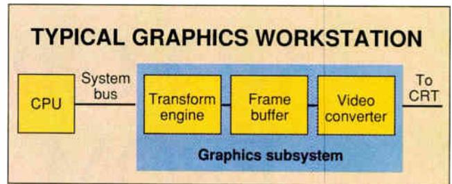
Figure 1: When dealing with a 3-D model, the system's main CPU passes the information about the object to the transform engine (in the graphics subsystem). This specialized floating-point processor converts the information into the 2-D screen image, which is stored in the frame buffer. The video converter reads the frame buffer to create video scan information.
