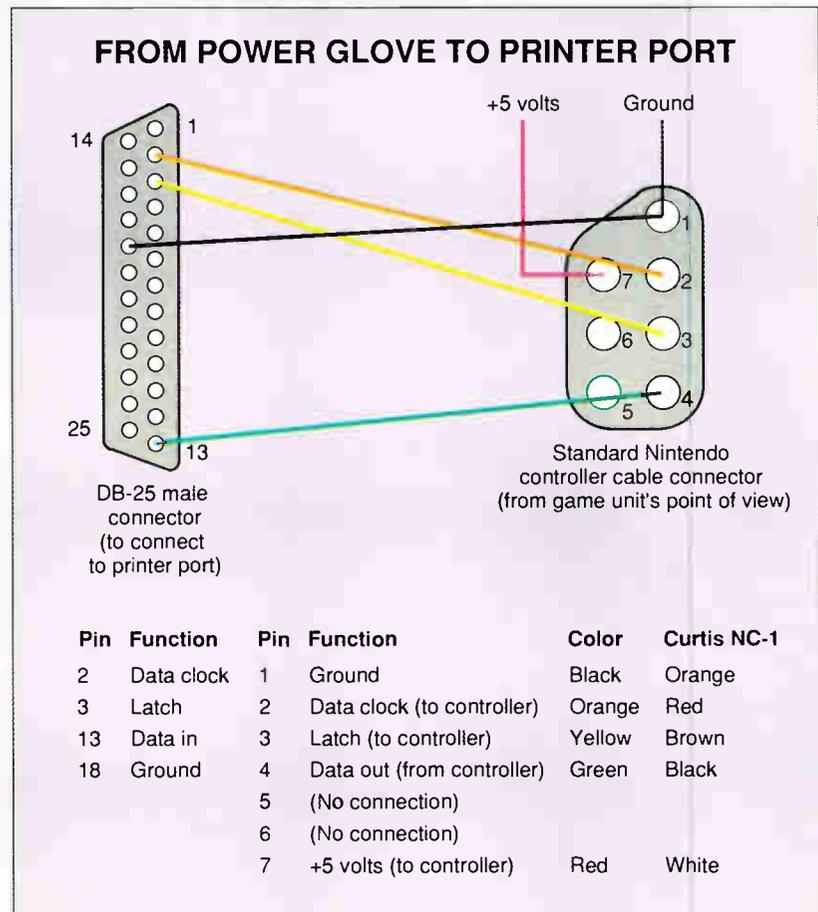
**Figure B:** This diagram details the wiring necessary to connect the Power Glove to a standard PC-compatible printer port. The colors shown are for the Mattel unit. They may vary from unit to unit, so be sure to verify them. If you choose to use the Curtis NC-1 Super Extendo cable, go by the colors listed for it.
