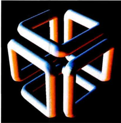
**Photo 1:** As rendered here, the Silicon Graphics logo contains roughly 1400 polygons. With solid surfaces, remote and local lighting, calculations of spectral characteristics of surface, and full color rendering, this object can rotate and move in real time. The animation is smooth and convincingly real.
