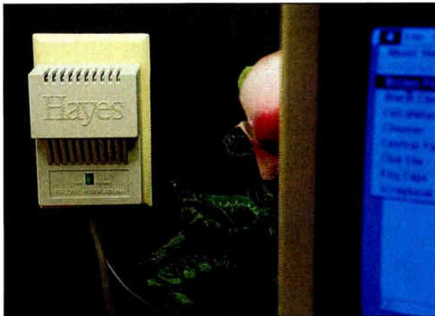
The Hayes Personal Modem 2400plus is a 2400-bps modem in an AC adapter.
