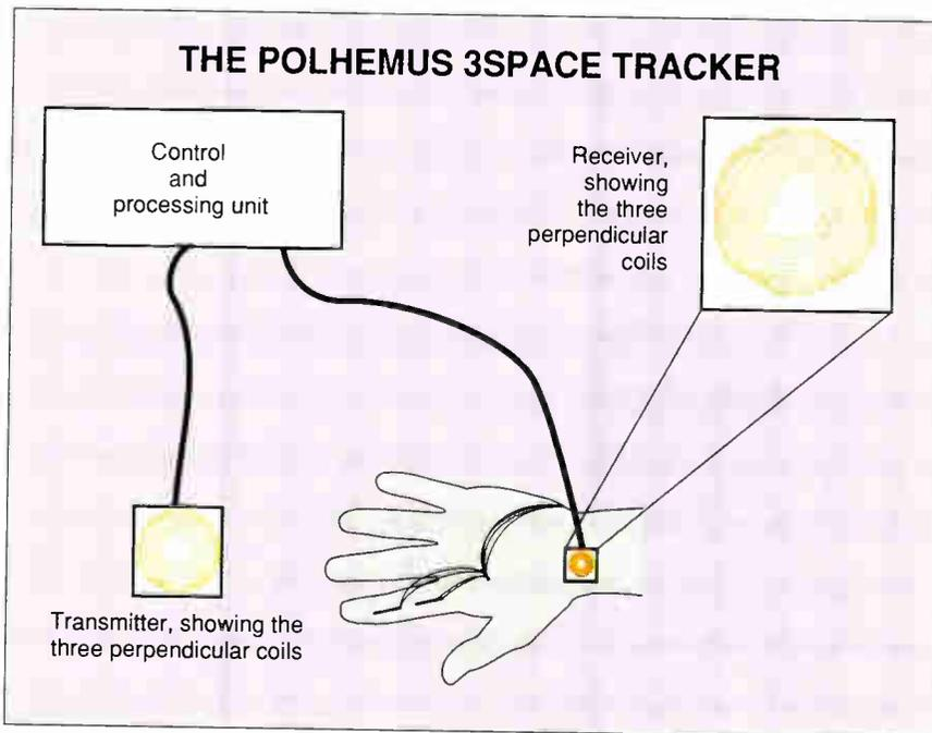
**Figure 2:** Designed to report the relative location of the user's hand in space, the Polhemus 3Space Tracker consists of a small cube mounted on the hand, and a slightly larger transmitter that rests on a stationary stand nearby. The cutaway views show the three perpendicular coils in both the transmitter and the receiver.
