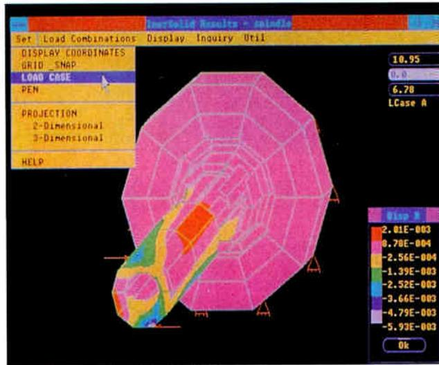
*InerSolid, the stress-analysis module of Inertia, shows the results of analysis on a spindle.*
