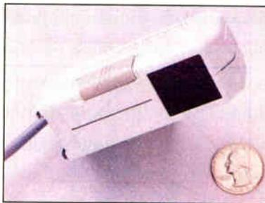
**Photo A:** *The Private Eye computer monitor is more useful than it may first appear. It lets you view important data while simultaneously working on tasks, and it provides the ultimate in portability.*
