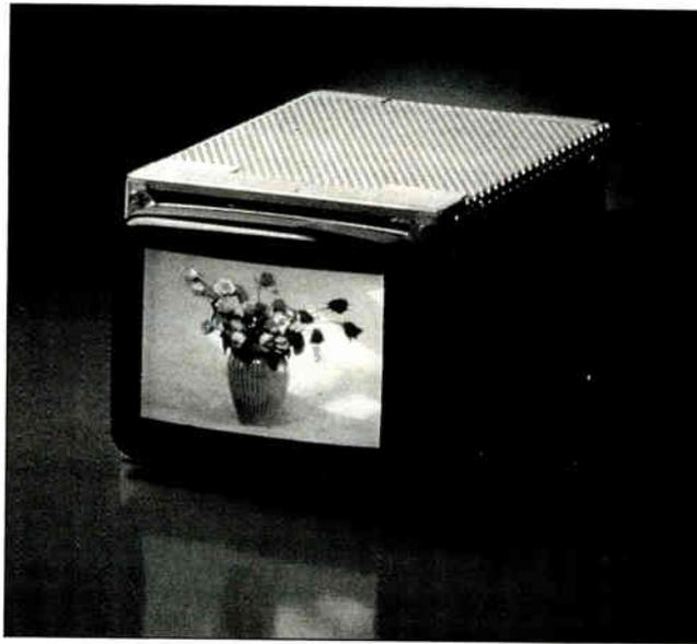
*The Color Pix.L monitor includes a self-compensating 85- to 264-V power supply, making it compatible with any voltage input in the world.*
