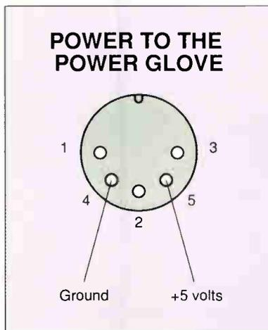
**Figure A:** To connect a Power Glove to your PC compatible, you need a 5-V power source. Pins 4 and 5 of a standard five-pin keyboard connector provide 5 V to the keyboard and can also be used to power the Power Glove.
