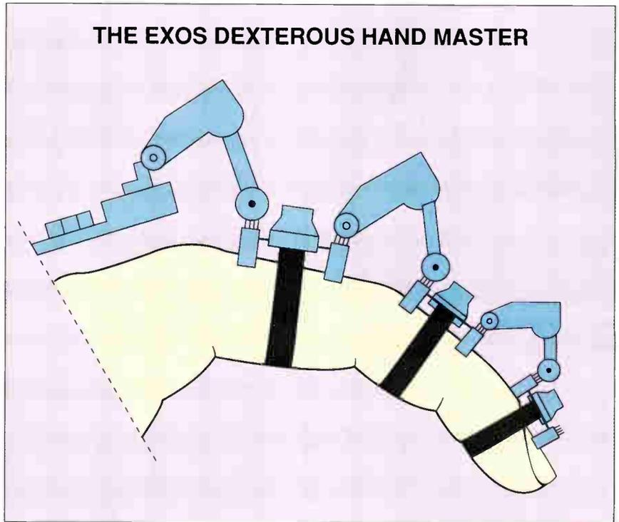
**Figure 3:** The Hand Master consists of an exoskeletal arrangement of sensors. The sensors are held over each finger joint by lightweight pads and Velcro straps. Each sensor houses both a Hall-effect magnetic pickup and a magnet.
