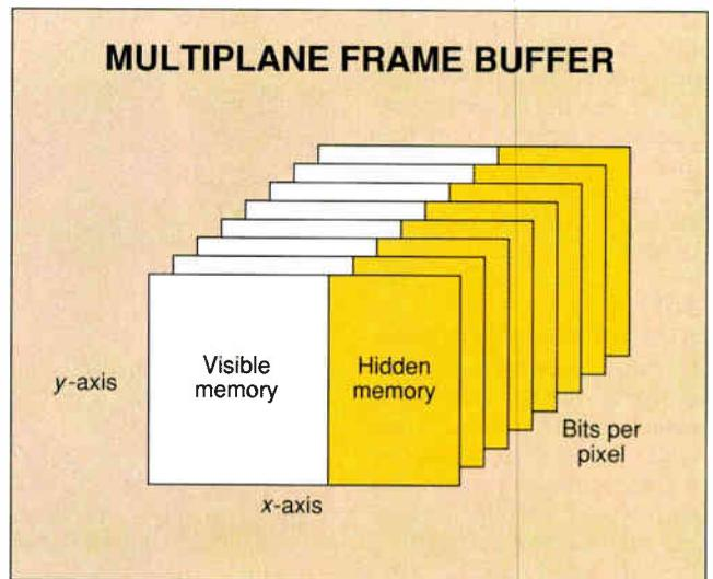
Figure 2: A graphical display with a single plane allows only monochrome images. Increasing the screen depth allows more colors, double-buffering for animation, z-buffering for 3-D rendering, alpha buffering for transparency, or antialiasing. The system shown here has 8 bits per pixel, which provides 2<sup>8</sup> options (256 color choices), and a portion of nondisplayable (hidden) screen memory, which can be used for fast generation of bit-mapped text, texture mapping, and pattern tiling.
