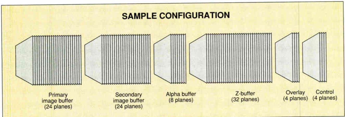
**Figure 3:** A frame buffer can have many bit planes and require a vast amount of memory. This configuration has a total of 96 bit planes. Assuming a screen resolution of 1280 by 1024 pixels, this represents 125,829,120 bits, or nearly 16 million bytes.
