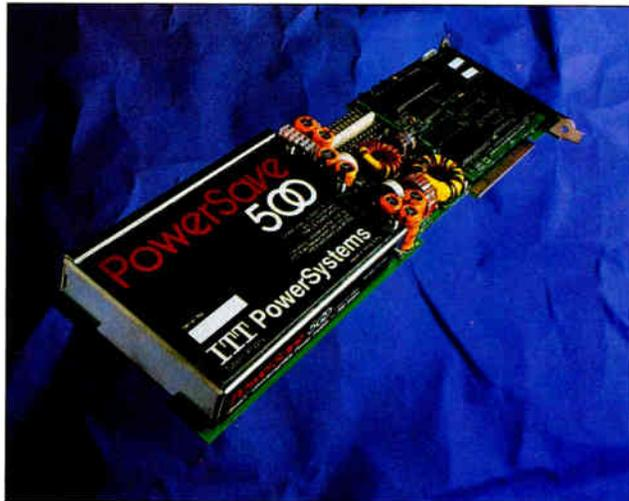
*ITT PowerSystems' VIP PowerSave 500 is a backup power supply with software for saving your work and automatically shutting down your system.*
