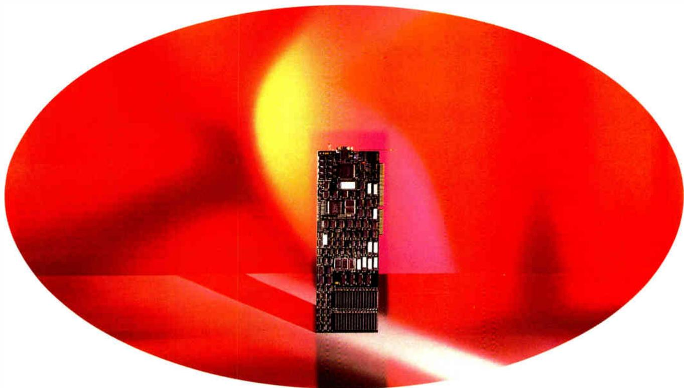
*The MultiSync Graphics Engine Board. Uses 50MHz TMS 34010 graphics processor to accelerate software applications as much as 900%.*
