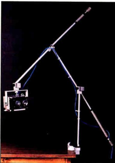
**Photo B:** *The CCSV, a stereoscopic viewer fixed on a counterbalanced kinematic linkage, lets you easily enter and leave the virtual world.*
