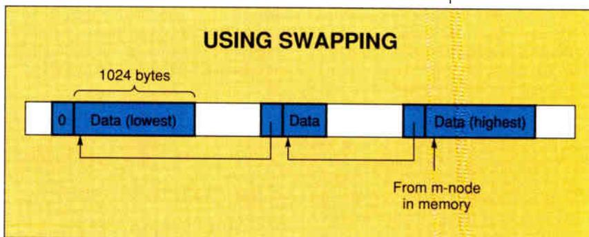
**Figure 4:** The swap file is divided into records of 1K + 2 bytes. The first 2 bytes serve as links in a backward-pointing chain. Data swapped out of the heap is chopped into 1K-byte pieces when written to the swap file. Note that the head of the chain actually begins with the record storing the data to be loaded highest in memory.
