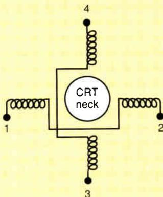
Horizontal control is applied to pins 1 and 2
