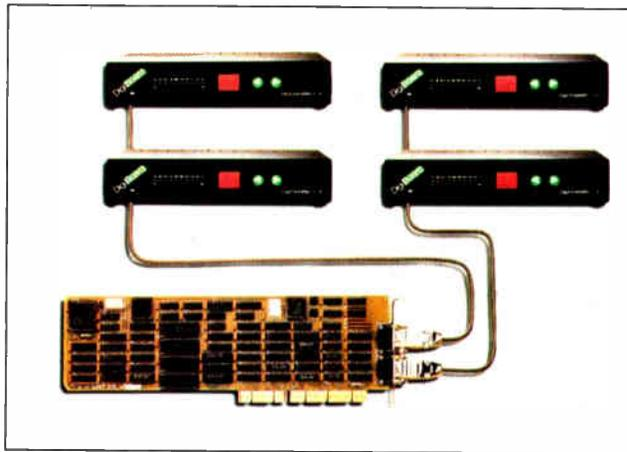
*The DigiChannel MC C/X System, with one board and one C/CON-16 box, lets your PS/2 inexpensively support 16 Unix users; with four boxes, you can support 64 users.*
