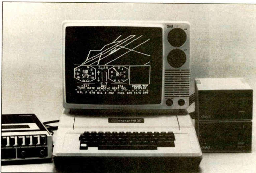
△ The Apple II used a 6502 and offered 16K bytes of RAM (expandable to 48K), 16K bytes of ROM, a keyboard, cassette interface, eight-slot motherboard, game paddles, and a color-capable graphics/text display, for \$1298.
