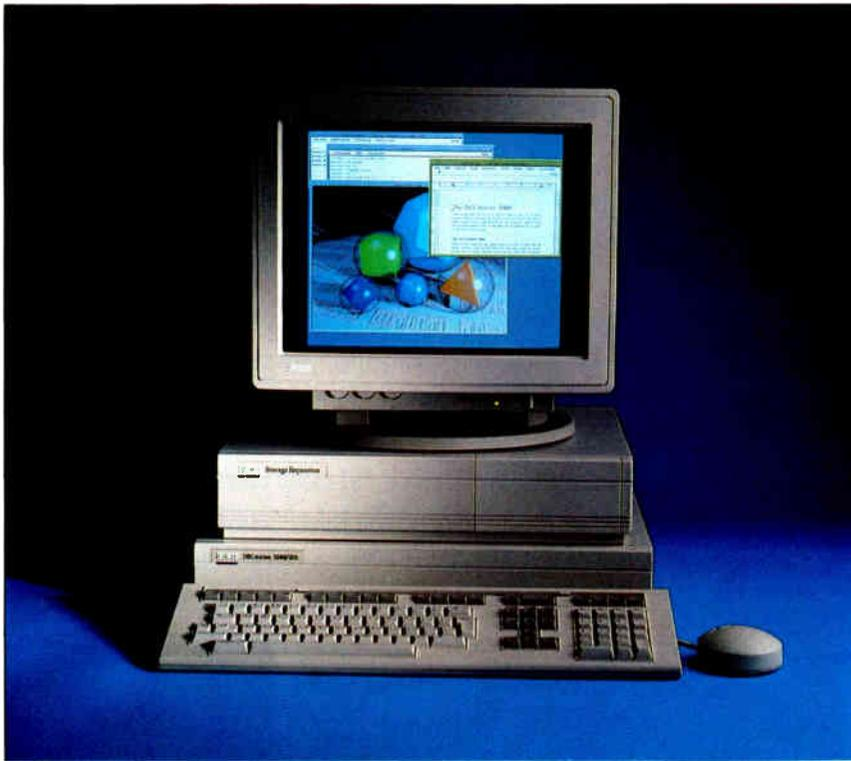
*The DECstation 5000 packs some serious performance into a compact box. The expansion cabinet atop the main unit holds the hard disk drive.*
