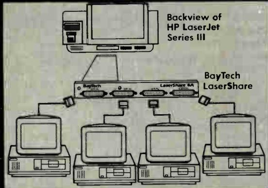
LaserShare is an expansion card that allows four users to connect to one laser printer, including the new HP LaserJet Series III. LaserShare simply plugs into the I/O slot of your laser printer, giving each computer access as if it were directly connected.
