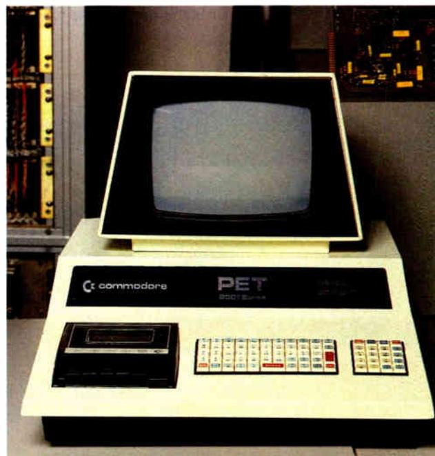
Commodore Business Machines unveils the **Commodore PET** (Personal Electronic Transactor) at the West Coast Computer Faire in April. The 6502-based machine cost \$595 assembled and included 4K bytes of RAM, 14K bytes of ROM, keyboard, display, built-in cassette tape drive, and 8K Microsoft BASIC.
