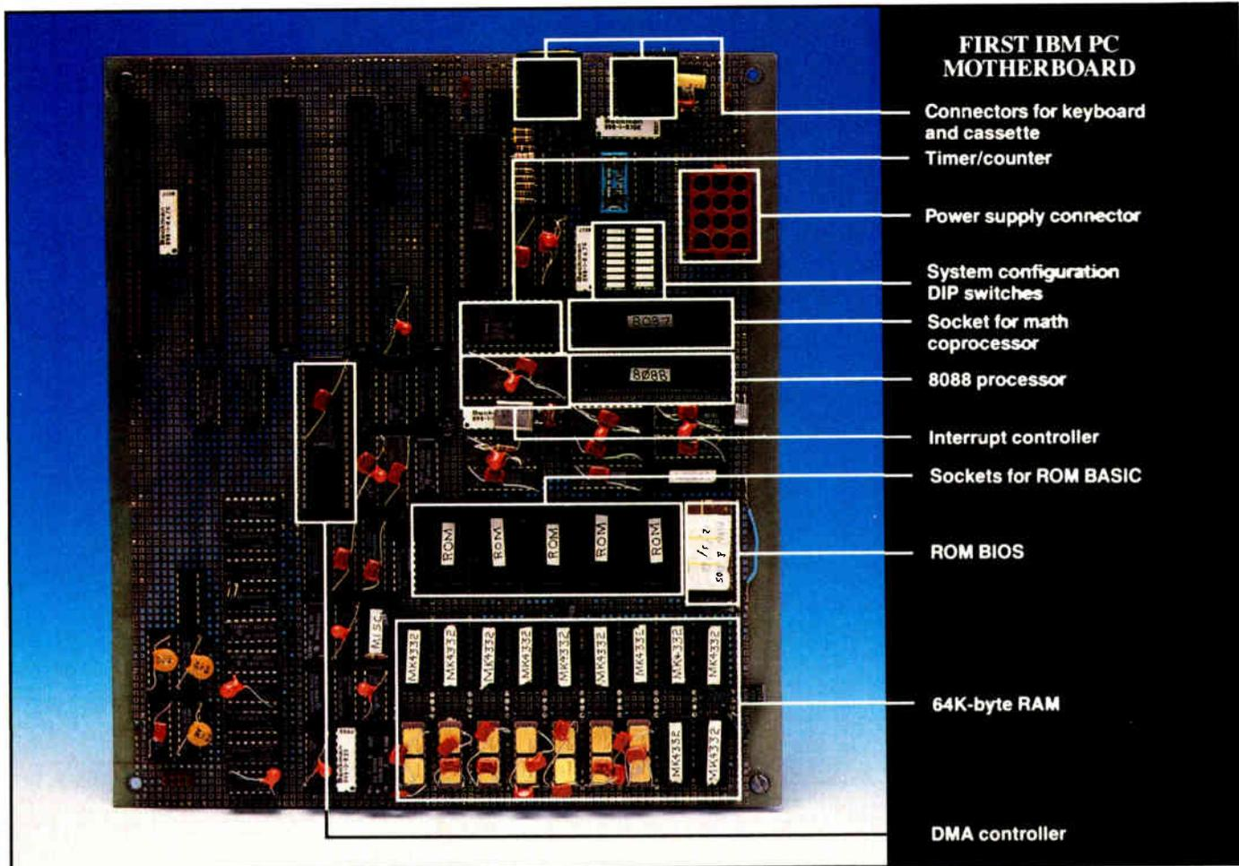
numeric coprocessor. The 8087 gave the 8088 a fast partner for floating-point calculations. But since the 8087 wasn't yet available when the PC was announced, we simply left an empty socket on the board and didn't disclose a use for it.
