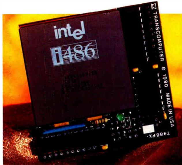
*CPU modules from TransComputer and Feith Systems can add 486 performance to your 386-based system.*
