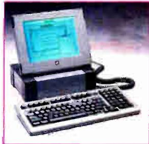
Optional paper white VGA LCD display with back-lit super twist technology.
