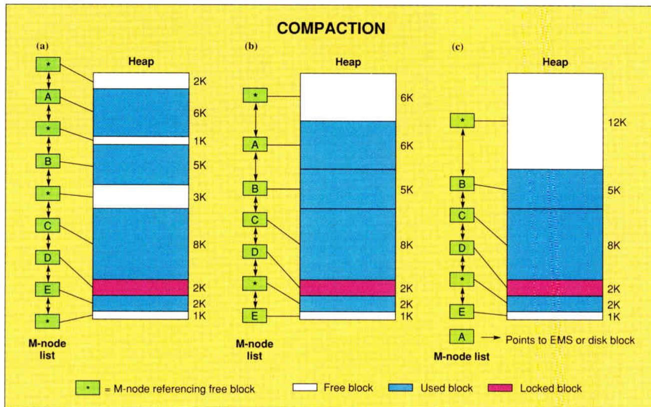
**Figure 1:** Swapping memory out of the heap begins when a memory request comes in. (a) The request is for 8K bytes, and no free blocks of 8K bytes exist. (b) The memory manager compacts the heap, freeing a block of 6K bytes. Not good enough, so (c) the manager swaps a 6K-byte block out to EMS memory or disk. A 12K-byte block is now available, and the 8K-byte request is granted.
