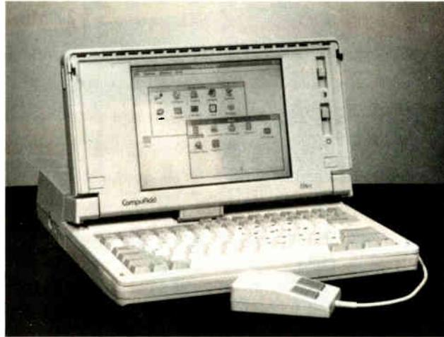
*The CompuAdd 316SL uses 12-V and nickel-cadmium batteries and ships with power-management software. The 316SL weighs 11½ pounds.*
