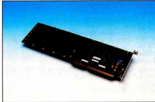
*Sixty-four Intel Flash chips make up the Flashdisk's memory. Similar to EEPROMs, the CMOS chips can be electrically erased and reprogrammed 10,000 times.*
