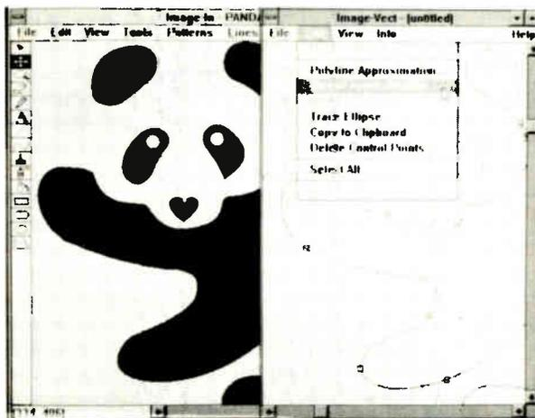
*The Image-In Vect module can convert bit-mapped images to vector images of any size. You can then export files to AutoCAD in DXF format.*
