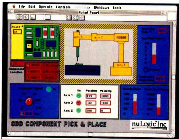
*As LabView 2 controls a pick-and-place machine for odd-shaped components, it displays at right information on insertion force, number of boards completed per hour, and total insertions while letting you control the conveyor speed in the lower left window.*
