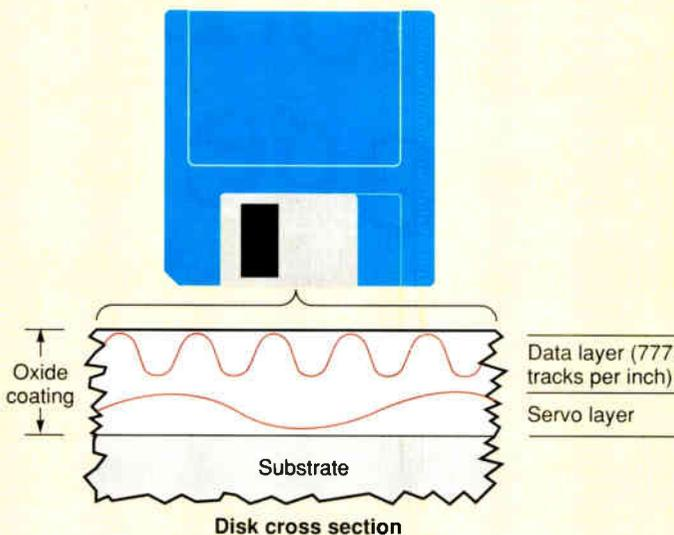
The oxide coating on the Stor/Mor's floppy media is divided into two layers. The bottom, or servo, layer contains an embedded homing signal that guides read/write heads. Accurate head positioning in part allows the drive to densely pack data in the upper layer into 777 tracks per inch.
