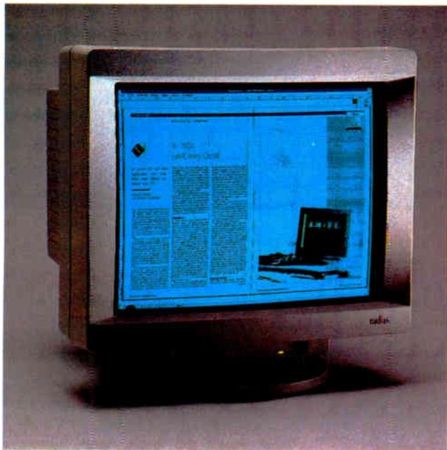
*Radius's 21-inch monitor includes a controller-based VGA chip and supports either PCs or Macs.*
