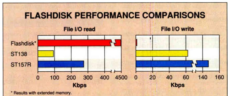
*Flashdisk showed markedly different results when performing file I/O reads and writes under the BYTE DOS Benchmarks (version 2.0). Here, the BYTE Lab compares performance against the Seagate ST138 and ST157R hard disk drives. All tests were conducted with a 6-MHz AT clone; higher numbers indicate better performance.*
