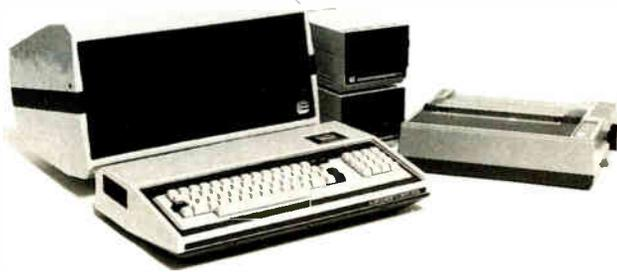
△ The Exidy Sorcerer sold for \$895 and included a Z80; 8K bytes of RAM; 12K bytes of ROM; a keyboard; and serial, parallel, and cassette interfaces. Its major innovations were the use of plug-in ROM cartridges for software and user-definable characters.
