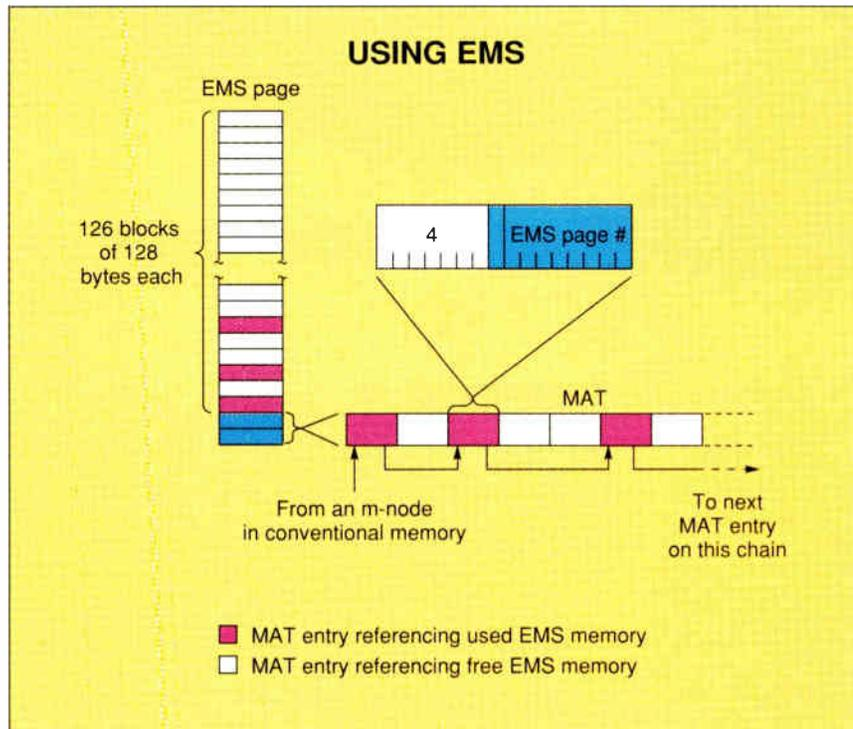
**Figure 3:** Each 16K-byte EMS page is divided into 128 blocks of 128 bytes each. In this figure, a chunk of heap memory has been swapped to EMS memory, and its data occupies EMS blocks 2, 4, and 7 on this EMS page. The MAT entries form a chain, linking the pieces of the data. Each MAT entry carries the EMS page number and block offset of the next entry in the chain, so MAT entry chains can stretch across several EMS pages.
