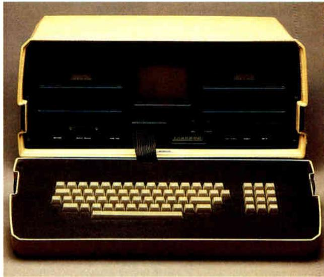
△ Adam Osborne, publisher of microprocessor books, unveils the \$1795 Osborne 1 Portable. It includes a Z80, a 5-inch display, 64K bytes of RAM, a keyboard and keypad, two serial interfaces, two 5¼-inch floppy disk drives and bundled software.
