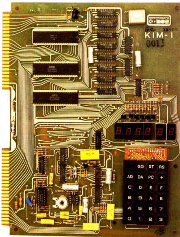
MOS Technology announces the KIM-1, a \$245 assembled single-board computer based on the 6502, with 1K bytes of RAM, LED readout, cassette and serial interfaces, and a 2K-byte ROM monitor. BYTE's write-up says that the KIM-1 "will prove attractive to readers who are not inclined to fondle hardware extensively."
