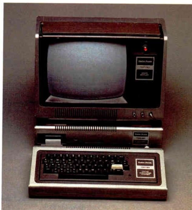
▷ The TRS-80 (TRS stood for Tandy Radio Shack) used a Z80 and had 4K bytes of RAM and 4K bytes of ROM (including BASIC), a keyboard, display, and cassette interface. Tandy spent only \$150,000 to develop the system, including design, tooling, and software. Reportedly, only a few thousand were made so that if it flopped, the systems could be used to track inventory in Radio Shack stores.
