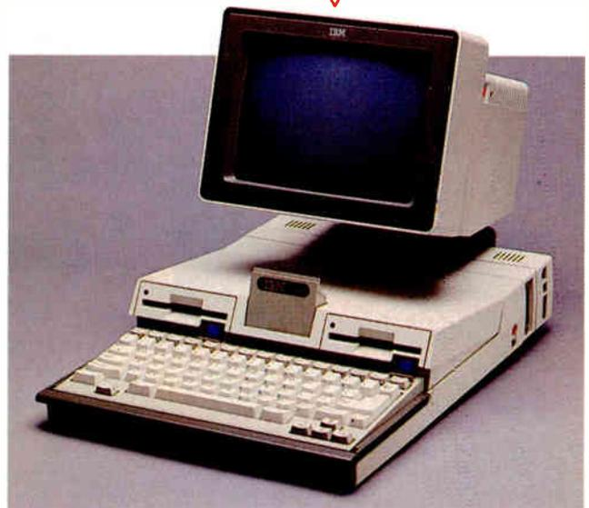
IBM introduces the PC Convertible, a 12- to 16-pound battery-powered laptop for \$2000, which becomes its second unsuccessful portable.
