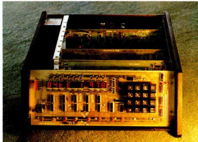
Heathkit introduces the **H-8** microcomputer kit based on an 8080 processor with an octal front-panel keypad.
