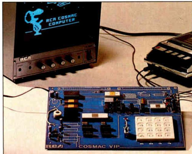
△ **RCA introduces the 1802 microprocessor.** It is later used in the RCA COSMAC VIP system, which was developed by Joseph Weisbecker from a design he pioneered five years before called FRED. The COSMAC included 2K bytes of RAM, 512 bytes of ROM, a hexadecimal keypad, and interfaces for video, cassette, and audio. RCA later exited the computer business.
