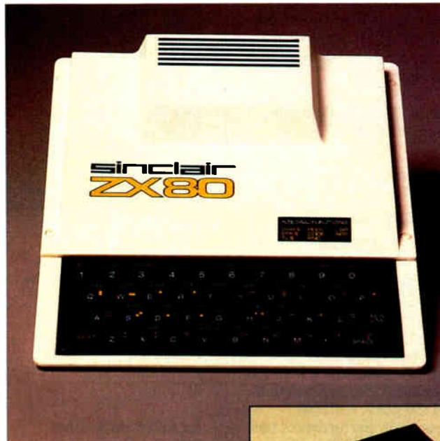
◁ The Sinclair Research ZX80 was the first microcomputer to cost less than \$200. Based on a Z80 with 1K bytes of RAM and 4K bytes of integer BASIC in ROM, it had a membrane keyboard and was the brainchild of English genius Clive Sinclair. The successor ZX81 (inset) was later sold by Timex and dropped to less than \$100 before Timex exited the market.
