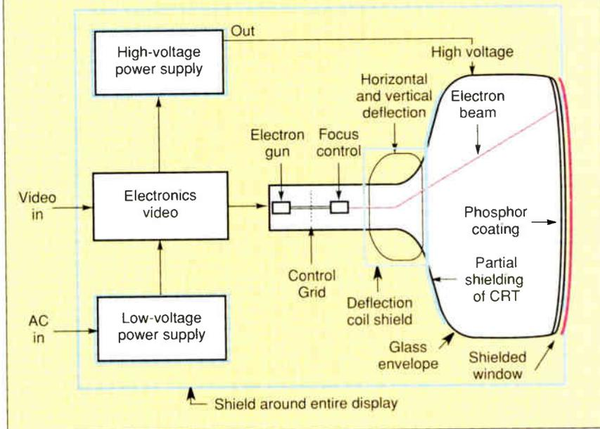
**Figure 2:** The face of the CRT is shielded with a well-grounded EMI window. The CRT glass envelope, deflection coils, power supplies, and the terminal itself are shielded with metals that have good ferromagnetic properties and good conductivity, such as iron and nickel.
