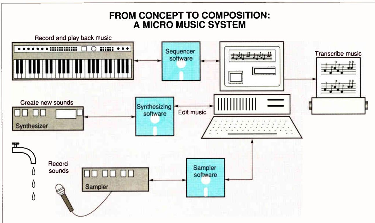
*The versatility of the personal computer and its graphics screen make it an ideal front end for any electronic music system. Software that performs sequencing, synthesis, sampling, and notation have made it possible to have an entire studio in a box.*
