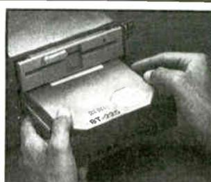
You install the 1.2 meg, 5¼" floppy disk drive, learning disk drive operation and adjustment. Later, you improve your data storage capacity dramatically by installing this powerful 20 meg hard drive.
