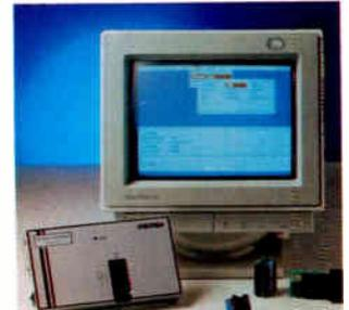
**T**he Logic Universal Programmer for programmable logic devices works with PLDs from all manufacturers, according to Xeltek. The Programmer offers an interface that combines pull-down menus, windows, and a command line.
