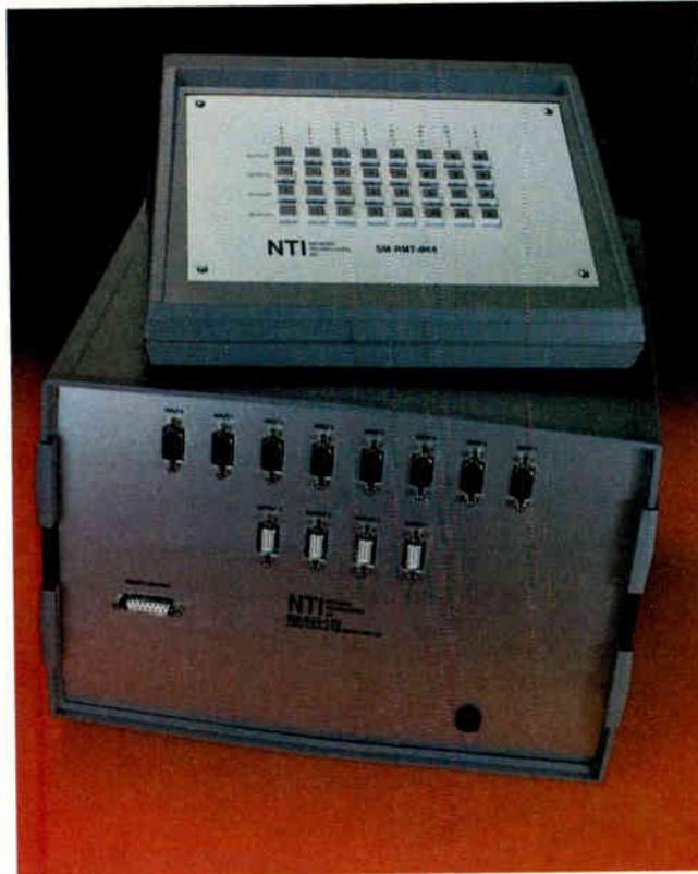
*You can remotely control up to four VGA displays from eight systems with Network Technologies' matrix switch (bottom) and remote-control unit (top).*
