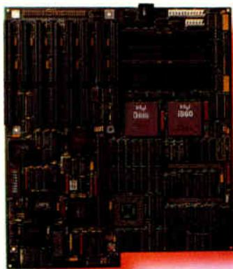
buffer card for ultra high-performance workstation graphics. **For UNIX Workstations, Too.** The 4860 board makes a great foundation for high-performance RISC workstations that run advanced UNIX applications. Many workstation vendors are choosing the i860 processor as a standardized vehicle for CAD and simulation systems, and the 4860 is perfectly compatible with these applications.
