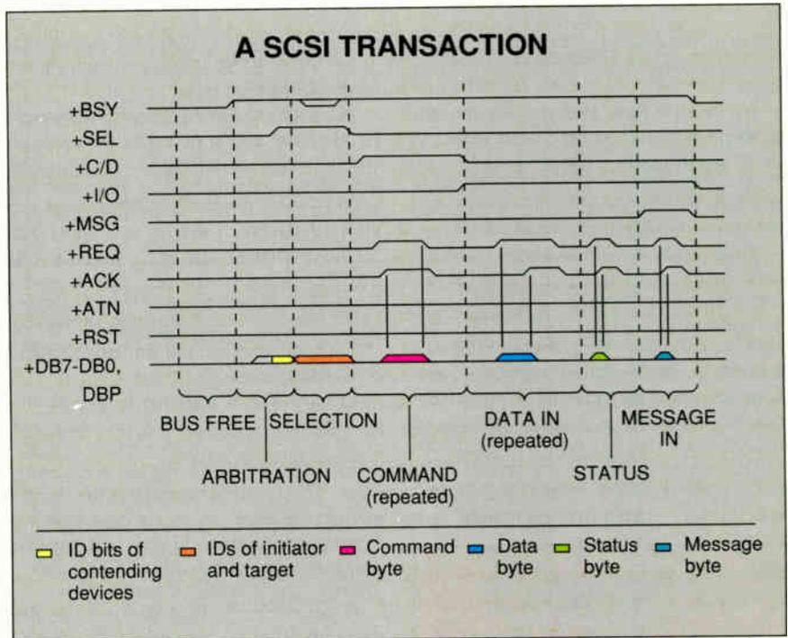
**Figure 2: SCSI bus timing.** During a transaction, the signals and phases can occur in the sequence shown. The ARBITRATION phase, which was optional in the original SCSI standard, is now mandatory in the new SCSI-2 standard described in the text. The target may disconnect during a lengthy operation, freeing the bus for other devices. The device reconnects later by use of a RESELECTION phase (not shown).
