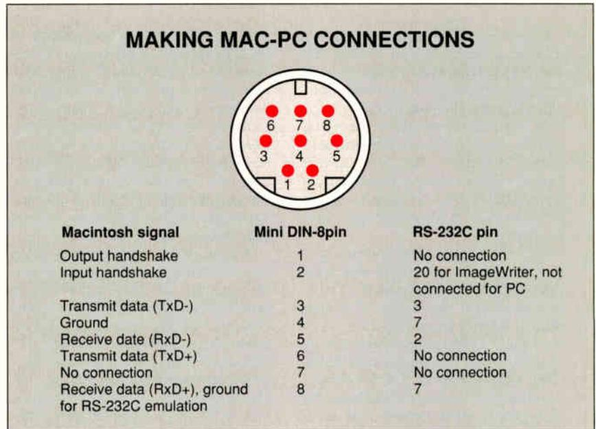
**Figure 1:** The schematic for a null modem cable to connect the serial ports of a Macintosh and an IBM PC. You can order an ImageWriter II extension cable and cut it in half to obtain the male DIN-8 connector. The DB-25 connector is available from most electronics stores.
