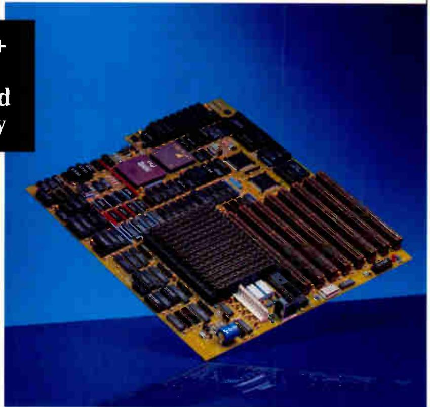
**Solid.** The 80486-33 EISA features 8 expansion slots with 6 EISA bus master slots, all of which allow for seamless integration of 16-bit and 8-bit AT/ISA I/O cards. Additionally, you'll have no more worries when your memory needs intensify. The 80486-33 EISA provides over ten various memory capacity choices from 1 to 64MB on-board! These memory configurations utilize 256K, 1MB or 4MB SIMM memory concurrently.
