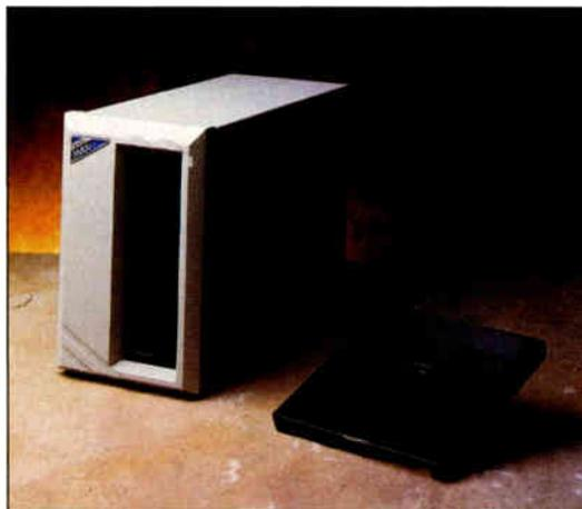
Removable hard disk drives are another option. These devices are like standard hard disk drives, but they come in two parts: a docking section installed in the computer, and a separate disk pack (see photo 1). You can unplug the disk portion from the docking section and plug it into another computer.
