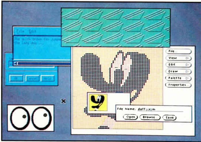
As can be seen above, the usefulness of having no window manager is debatable, but by no means impossible. Having no window manager active would most probably occur when only one X Client is being run on an X Server.
