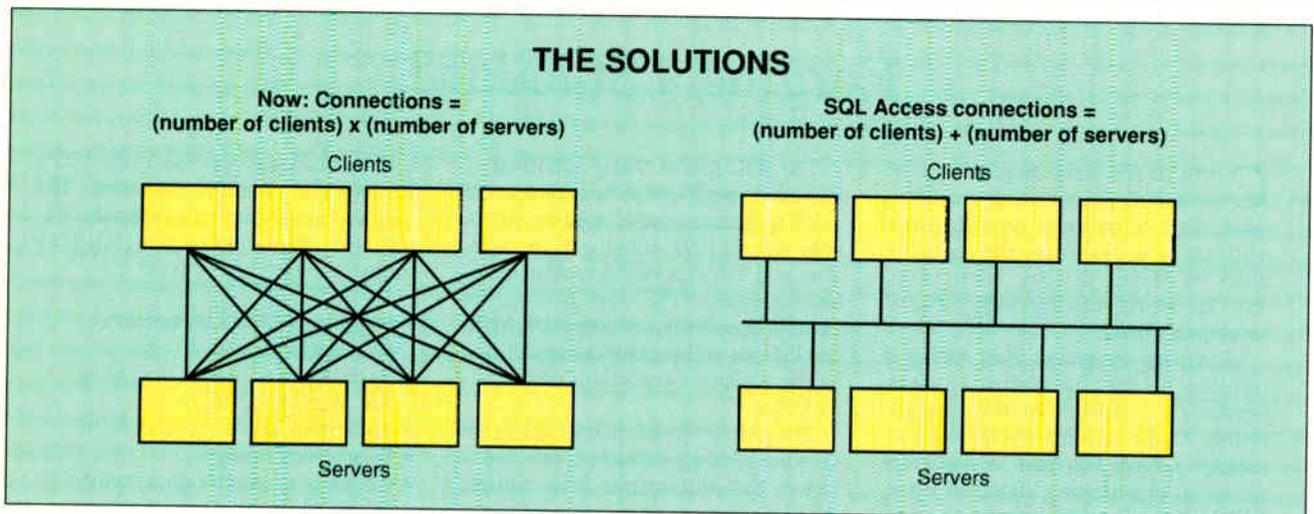
**Figure 2:** Without a SQL standard, a separate gateway has to be written for each client and server in use. The SQL Access Group technical specification, when adopted by the industry, will enable SQL software interoperability, as well as portability of SQL applications.
