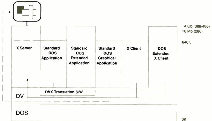
DESQview is loaded on top of DOS, the first program booted into the computer. Multitasking within DESQview can be several program partitions. In the case of DESQview/X, one contains an X Server.
