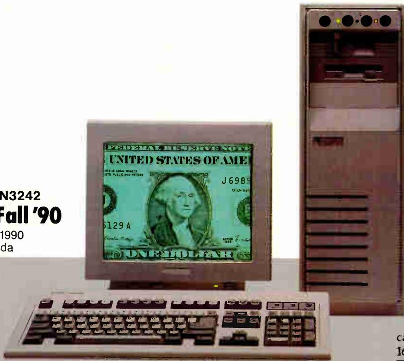
DTK 386 systems deliver superior performance at prices that are hard to beat. **33MHz Cache.** Take our KEEN-3300 Series for example. Its innovative high speed writeback cache memory and 80386-33 microprocessor combine to deliver zero wait state performance and a MIPS rating of 8.2.
