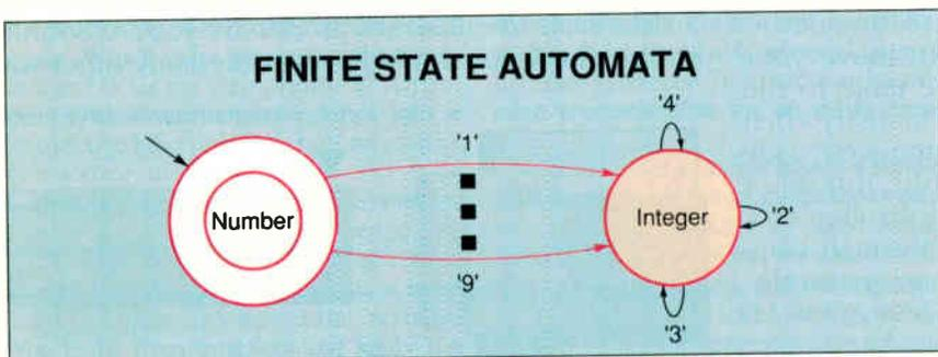
**Figure 1c:** The state-transition diagram describes how finite-state automata can change. The machine starts in a known state, parses an input condition, consults the transition diagram (or table), and determines which state to engage next.
