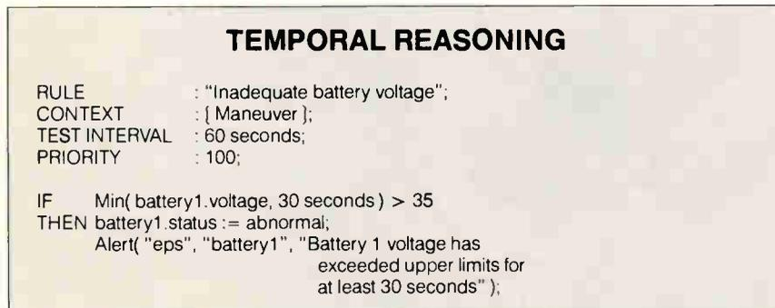
**Figure 4:** With the capacity to remember the past, a real-time expert system can then build rules that take advantage of this feature. This rule checks the recent voltage values to see if the battery is in an abnormal state.
