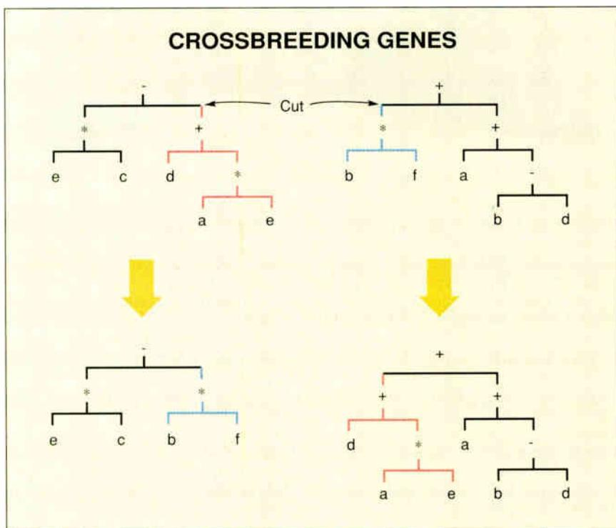
**Figure 2:** To "breed" two possible solutions and come up with a still better solution, you can perform "crossover breeding." Here, two solutions (top) are cut at the points indicated, and the subtrees below those points are swapped, resulting in two new solutions (bottom). Note that one of the new genes is the correct solution shown in figure 1.
