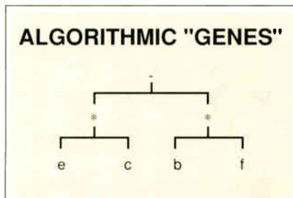
**Figure 1:** To solve the two simultaneous equations  $ax + by = c$  and  $dx + ey = f$  (where  $x$  and  $y$  are unknowns and  $a, b, c, d, e,$  and  $f$  are constants), you can set up a binary tree with the constants as "leaves" in the tree, and mathematical operations at the branches. Solving for  $x$  gives  $x = (ec - bf) / (ae - bd)$ . If you assume that  $ae - bd = 1$ , then  $(ec - bf)$  is the correct answer. This tree shows how this "gene" is represented in the computer.
