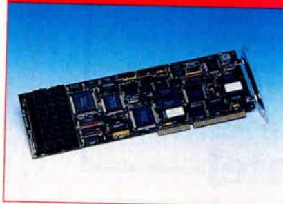
Based on its price alone, CompuAdd's HardCache/ESDI is instantly attractive. At \$895 in its tested 4-MB configuration, the HardCache costs less than half the price of comparable ESDI controllers. Although its performance lagged behind the others in this select group, the HardCache significantly improved performance over that of a standard controller.
