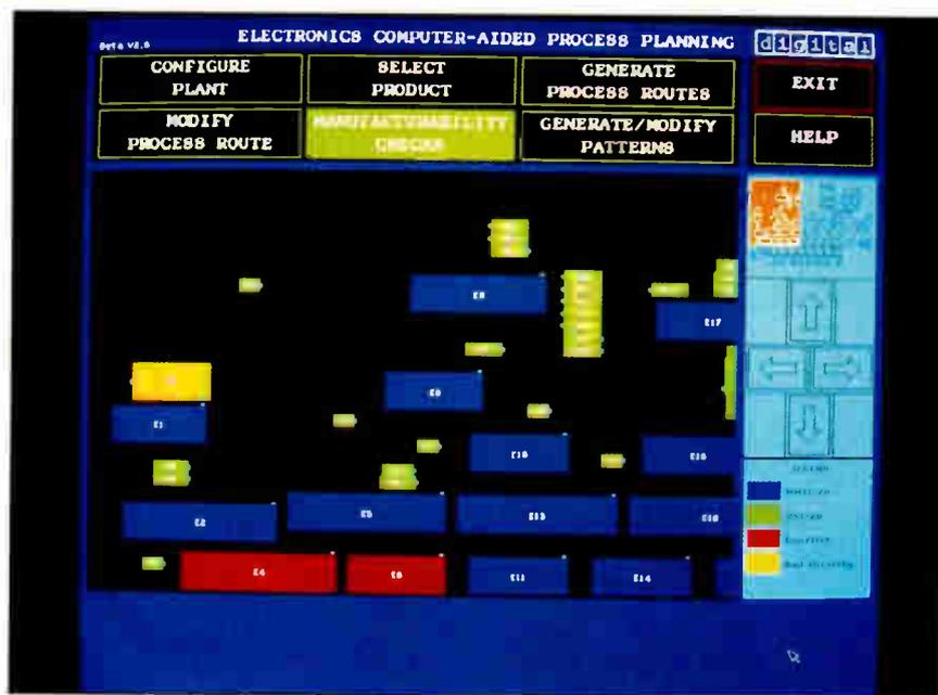
**Photo 2:** A graphical display of the printed circuit board with its components color-coded according to the machine that will be used to assemble them. Components that exceed manufacturing constraints are highlighted: spacing-rule violations are shown in red; polarity-rule violations are shown in yellow. (Photo courtesy of DEC)
