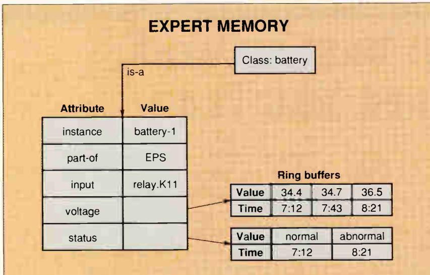
**Figure 3:** To function in a real-time environment, an expert system must be able to remember historical data. The figure shows how ring buffers let a frame-representation system remember information about battery voltage and status.
