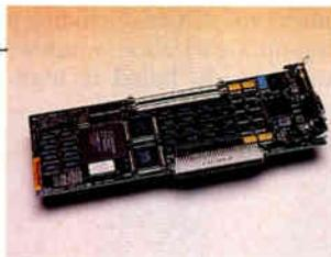
from the Mac's CPU. The board's buffers store and manipulate bit-mapped images without the penalty of moving chunks of data from main memory to the display board. Both are a potent combination that allows high-end Macs to be versatile graphics workstations for scientific, engineering, and photo-imaging work.
