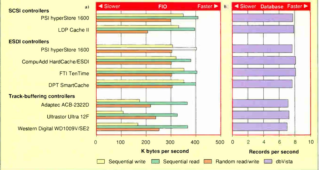
**Figure 2: Performance under NetWare 386 version 3.10.** Performance of all the boards was similar on all tests (a,b). Our four-user LAN simulation apparently did not push NetWare past its own cache; in small networks, even heavy random disk access may not show a measurable benefit from a caching controller.
