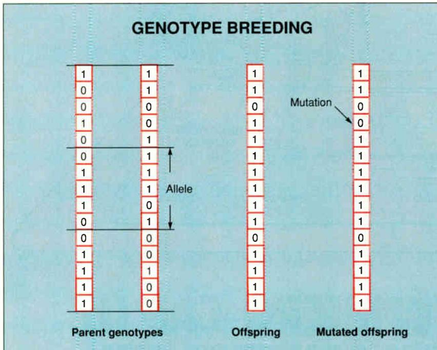
**Figure 2:** The parent genotypes are bred together, producing an offspring that inherits a random contribution of alleles from both. The offspring's genotype is then subjected to a mutation, where some bits in the genotype are "flipped" to account for this random, natural occurrence. The mutation rate is usually much rarer than depicted here (about 1 bit per thousand is typical).
