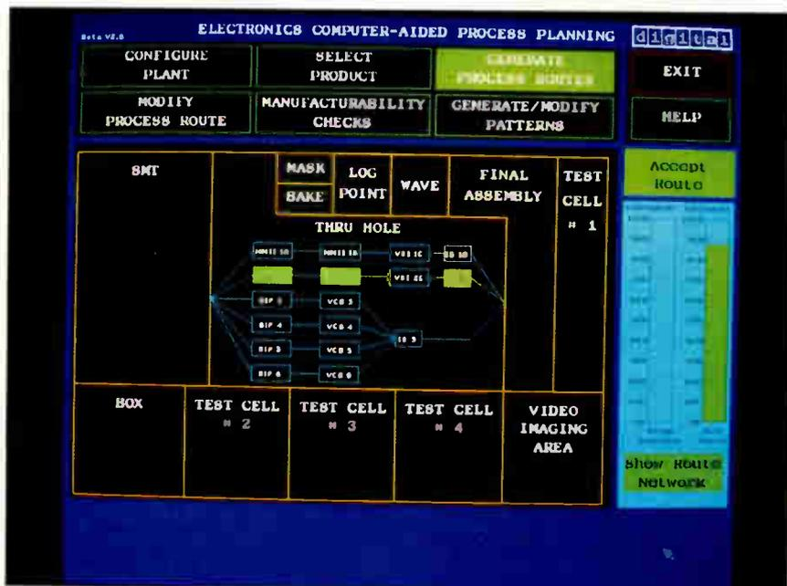
**Photo 1:** All the feasible process routes for a printed circuit board shown on a layout of the factory floor. The recommended route highlights the selected machines. Note in the "thermometers" on the right that the recommended route has an 85 percent automatic assembly with no setup required. (Photo courtesy of DEC)
