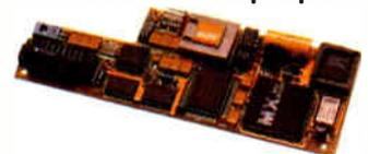
The MaxFax 9624LT-T is Macronix's new integrated fax/modem for Toshiba laptop and notebook computers. The 9600-bps fax and Hayes-compatible 2400-bps modem card fits into the dedicated internal modem slot on most Toshiba laptops.
