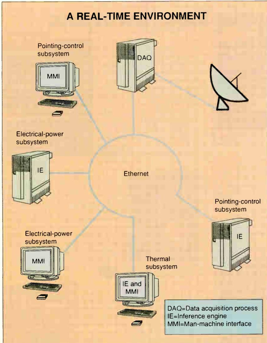
**Figure 1:** By distributing different functions to different processors, a knowledge-based system cuts down the load on any one processor, making the system faster and more responsive. In the example, the inference engine, data acquisition, and man-machine interface processes reside on different processors.
