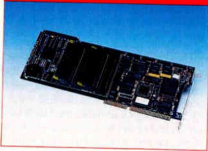
Like many other caching controllers, TenTime from FTI acts less like a controller and more like a dedicated coprocessor board. It has a 68070 CPU that executes a proprietary real-time, multi-threaded operating system. The operating system supports error correction and intelligent cache management (the details of which the people at FTI were understandably reluctant to reveal).
