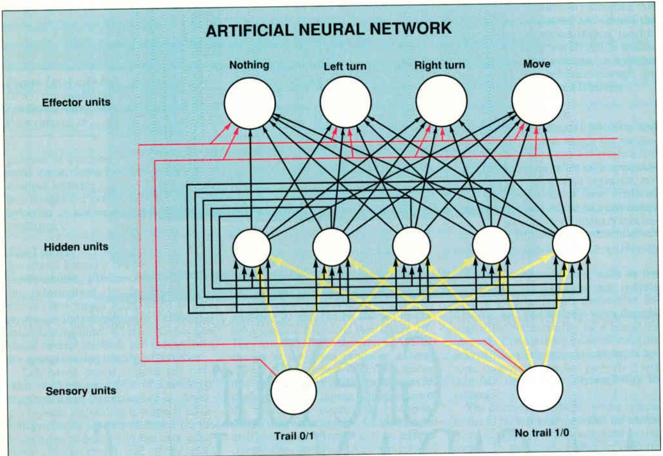
**Figure 1b:** The artificial neural network may be used as knowledge representation for certain forms of artificial life. The sensory units act as input discriminators, the hidden units provide connection and feedback, and the effector units generate output conditions. (Figure courtesy of David R. Jefferson)
