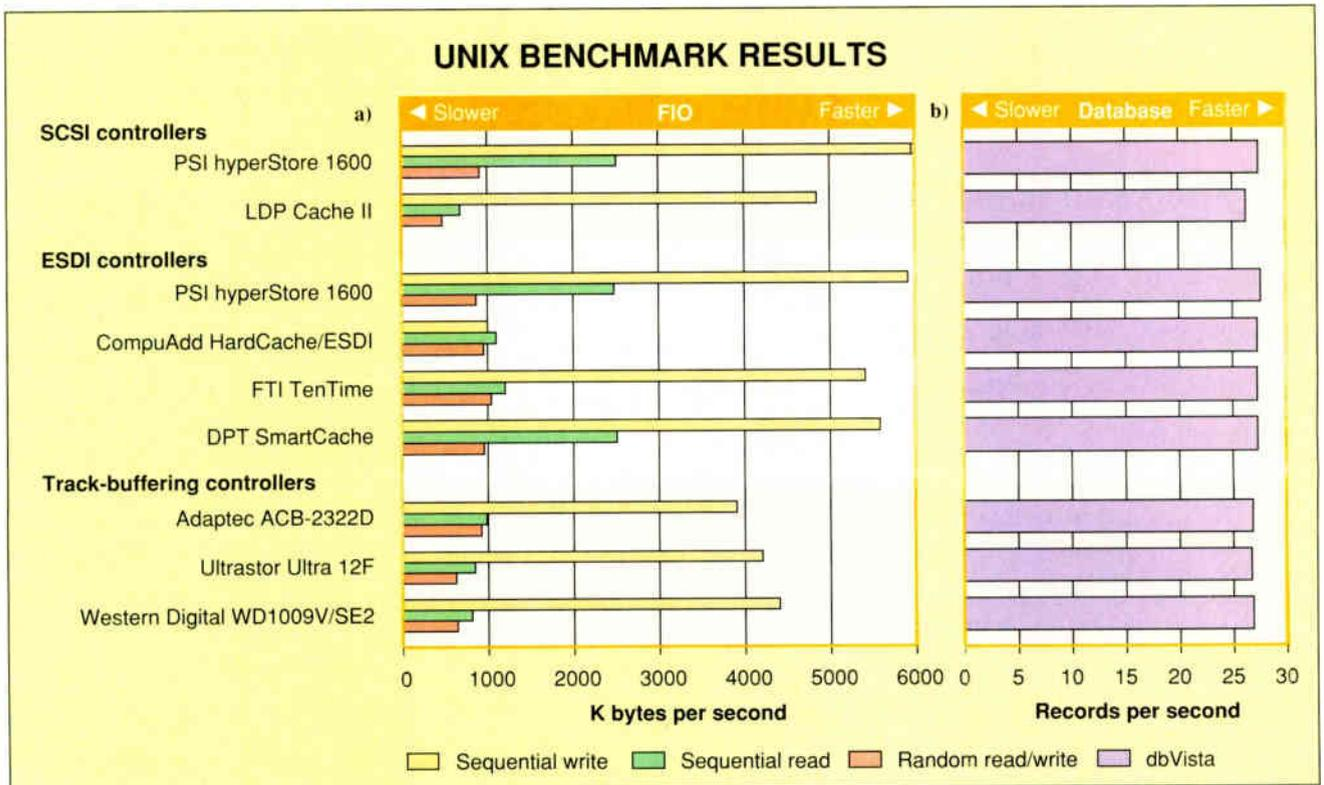
**Figure 3:** Results of our benchmarks under SCO Unix. (a) Notice that the hyperStore 1600 continues to perform well. Also note that Unix's write-buffering scheme favors write operations over read operations. (b) SCO Unix's own buffers were able to handle most of the dbVista throughput (even the track-buffering controllers did well), so the results are tightly grouped. The hyperStore 1600 barely edges past the competition.
