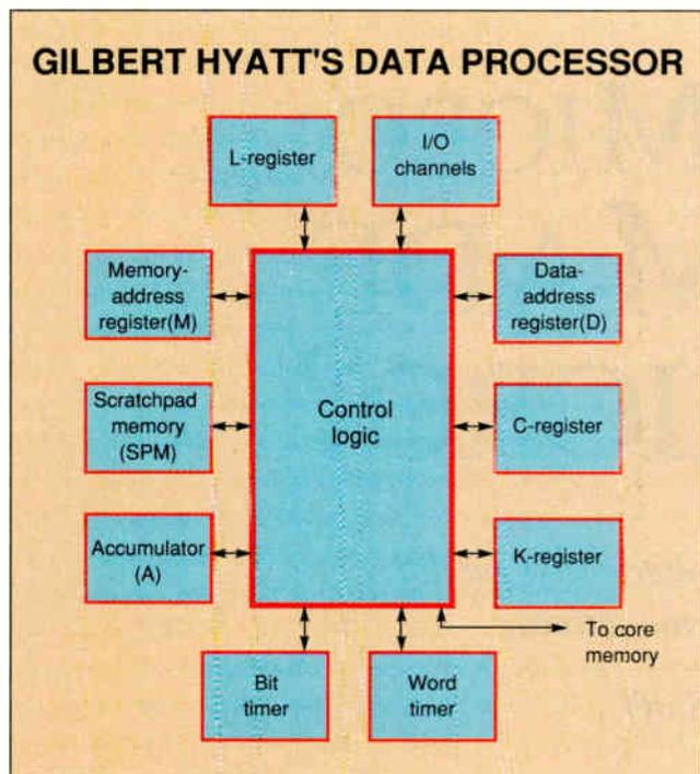
*This block diagram, from the patent granted Gilbert Hyatt, shows the components of his data processor. The basic timing functions derive from bit and word timers. Basic arithmetic happens in the A register. The C, K, and L registers handle instructions and control. The M register is used to address main memory. The SPM registers provide intermediate storage independent of the main memory. The I/O channels move data to and from registers.*
