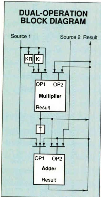
**Figure 2a:** The multiplier and adder can receive inputs from registers, their own outputs, or each other's outputs. They can be wired 62 different ways to create special-purpose instructions, such as "multiply-accumulate."
