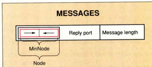
**Figure 3:** The Amiga operating system uses "messages" to pass information from task to task, as the basis for I/O requests, and as the medium of transfer for Intuition's mouse and window events. A message incorporates a node and therefore inherits all its properties and functions.
