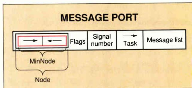
**Figure 4:** A message is transmitted to a message port, which contains a list of incoming messages to be serviced, in priority order. Like messages, message ports incorporate a node and therefore inherit all the properties and functions of a node.
