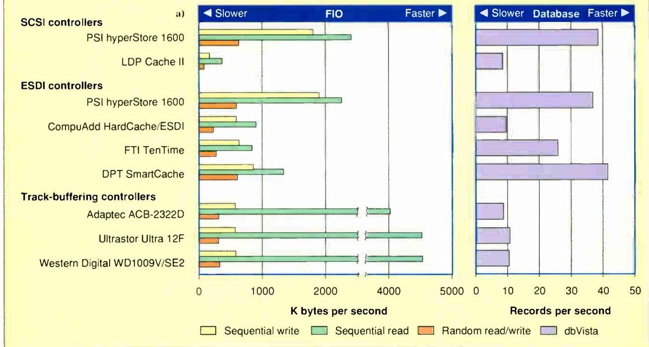
**Figure 1: DOS benchmark performance.** PSI's hyperStore 1600 clearly demonstrated superiority on sequential operations (a), while DPT's SmartCache edged it out on our random tests. (b) In our dbVista benchmark, the performance of CompuAdd's HardCache/ESDI suffered because of its write-through design.
