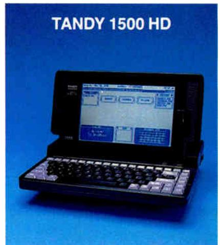
**T**andy's 1500 HD isn't the fastest XT-class machine, but it has several notable features, and Tandy's many retail outlets make servicing easier. Tandy powers the machine with a 10-MHz V20 processor. The basic system, at \$1999, includes 640K bytes of RAM, a 20-MB
