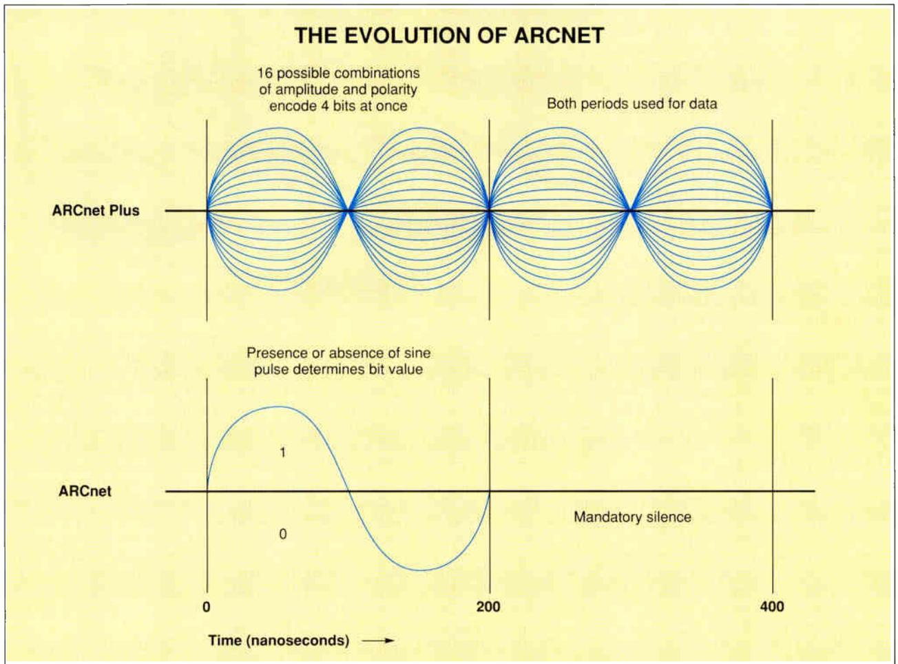
The original 2.5-Mbps ARCnet signals bit values by determining the presence or absence of a sine pulse. Here, ARCnet signals a "1" bit by sending a 200-ns pulse, followed by a silence of equal length. The 20-Mbps ARCnet Plus specification makes more efficient use of the bandwidth by using both periods for data and by using amplitude modulation to encode 4 bits into every pulse. ARCnet Plus also sends a calibration pattern once for every 8 bytes, further reducing overhead.
