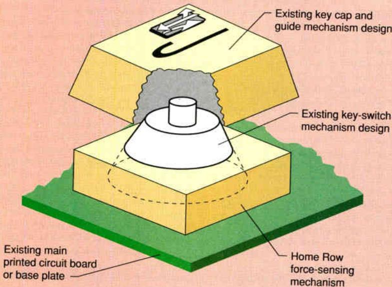
*This pointer-in-a-keyboard uses no real estate and costs nearly nothing. The Home Row is a joystick embedded in the J key; when another key is toggled, the J key rocks on its base, moving the screen cursor. Key Tronic is manufacturing OEM keyboards with this feature under the name "KeyMouse."*
