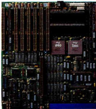
By adapting Intel's APX (Attached Processor Executive) software to our 4860 MotherBoard, we've created a way to exploit the power of the i860 to give you *practical* multiprocessing. In fact, i860/APX provides a base for entirely new applications made possible by the advent of the i860 RISC processor.
