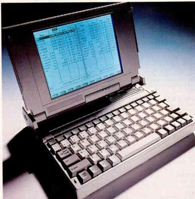
battery, and if there's a problem, it flashes red. There's the usual audible beep when the battery starts to run low. You can charge the battery when the system is on if you put it into suspend mode.
