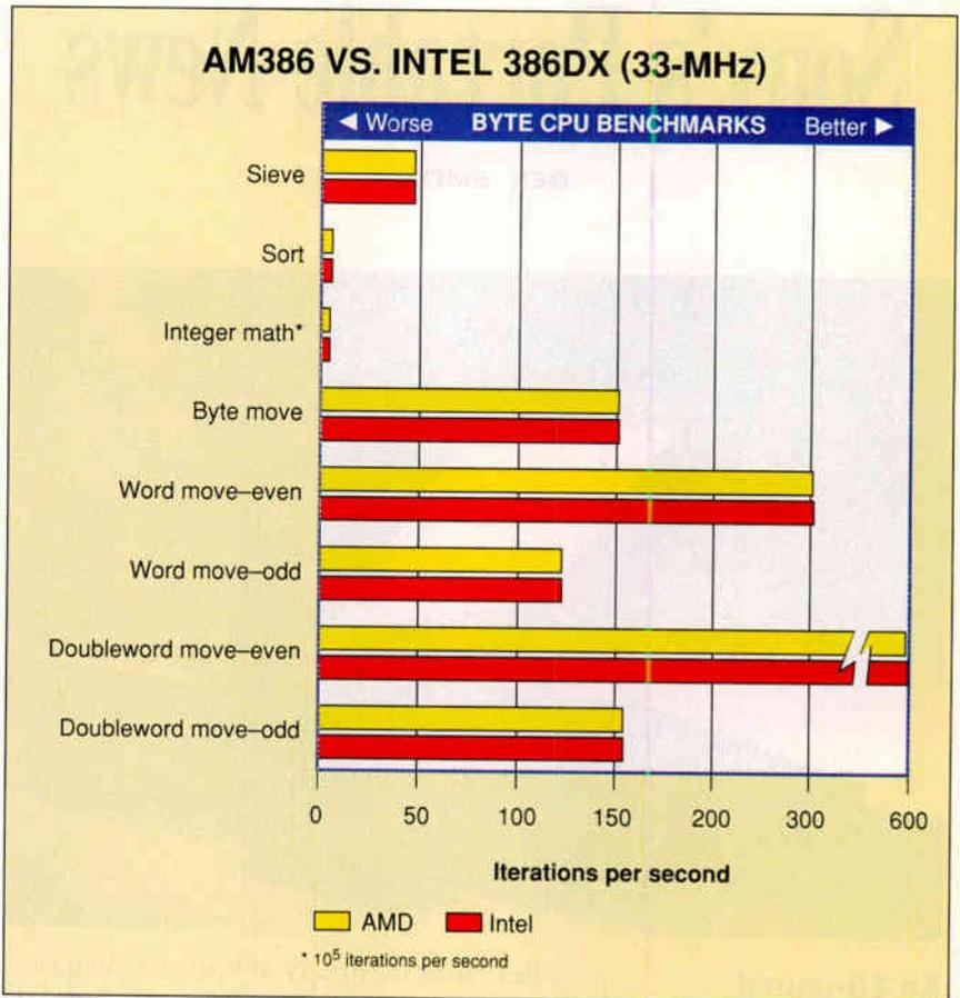
*The AMD Am386 and Intel 386 processors are, for all practical purposes, identical in performance. (The occasional differences are too small to matter.) All units are iterations per second except integer math, which is 10<sup>5</sup> iterations per second.*
