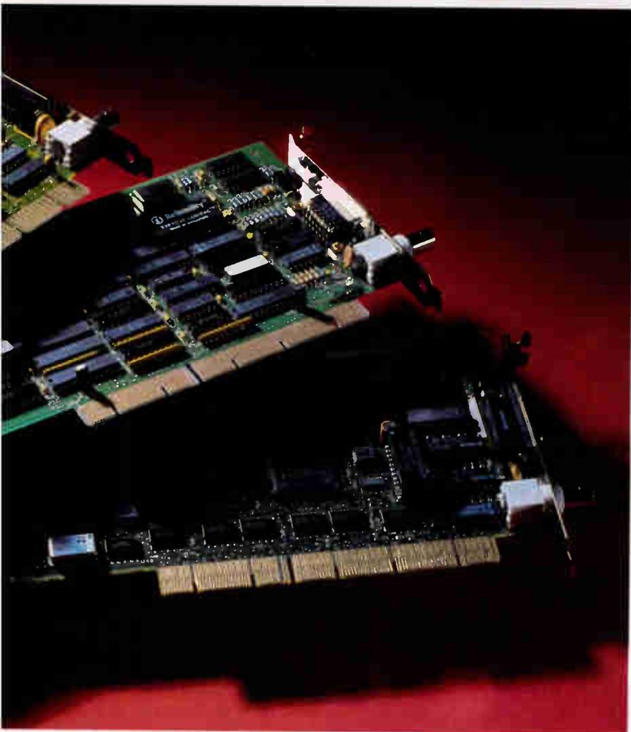
*The Mylex LNE390 (left) offers the most flexibility. You can configure it for DMA, I/O-mapped, or memory-mapped operation. The Racal-InterLan ES3210 (center) communicates via shared memory. Novell/Anthem's bus-mastering NE3200 (right) is the only adapter with an on-board coprocessor.*
