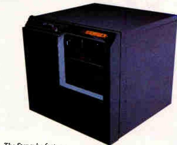
*The Stepcube features tool-less device installation through its access panels.*
