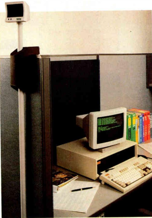
*Instead of requiring you to run cables through your office, InfraLAN relies on an infrared base unit that supports up to four computers and two optical nodes for sending and receiving signals from other base units. Optical range lists at 80 feet.*
