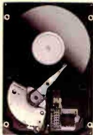
The T2000SX has a 40MB hard disk with 19 msec access time.
