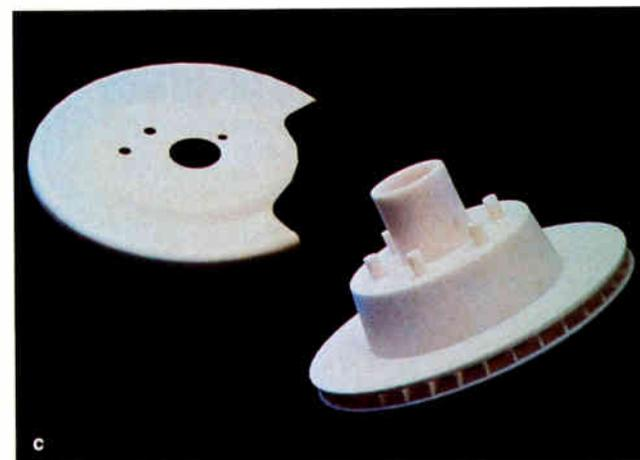
**Photo 1:** Selective laser sintering, a process developed by DTM, starts with a surface model CAD design (a). A laser then “welds” together particles of wax or plastic (b) to create a single cross section of the model. The system builds layer upon layer to create a model, which is used to make the finished object—in this case, a gear (c).
