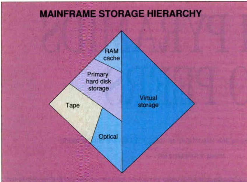
**Figure 1:** The classic centralized-mainframe storage hierarchy covers a variety of capabilities: backup; disk space management and grooming; archive and tape library management; and audit trails, accounting, and usage-trend analysis.
