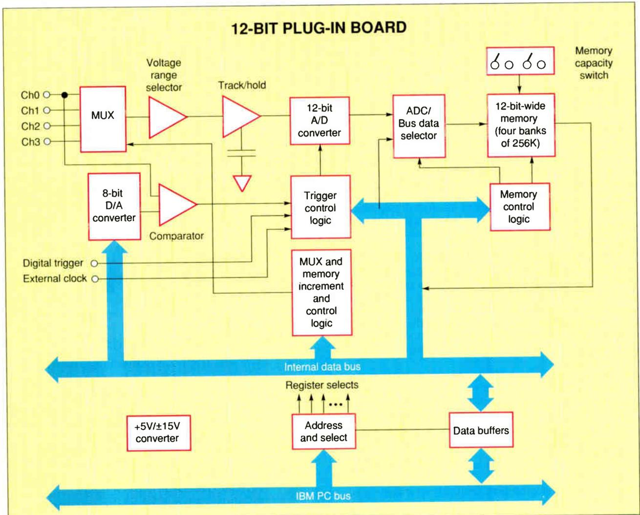
**Figure 2:** The block diagram of a 12-bit data acquisition board for IBM PC compatibles. This is a plug-in board with four measurement input channels and a sampling rate of 1 million samples per second. (Courtesy of Keithley Metrabyte)
