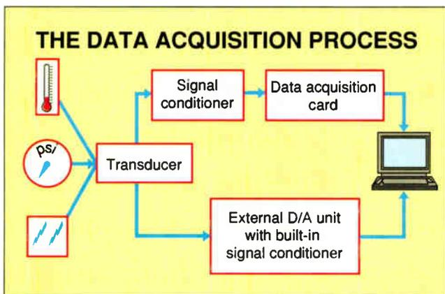
**Figure 1:** Data acquisition involves measuring some physical phenomena, such as temperature, pressure, or voltage (left), using sensors or transducers. The captured signals must then be conditioned, either by a separate unit (top) or by one built into a stand-alone data acquisition unit (bottom). The signal is then converted to digital form, and the data is manipulated and displayed on a computer equipped with data acquisition software.
