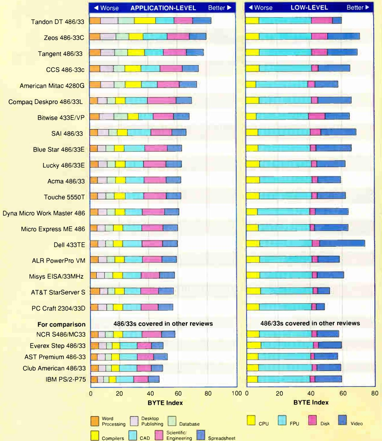
The BYTE DOS benchmark test results, ranked by cumulative application index score, show the Tandon DT 486/33 in the top spot. This results from its large disk cache and hides a relatively poor showing in the low-level video tests. For each index score, an 8-MHz IBM AT = 1.
