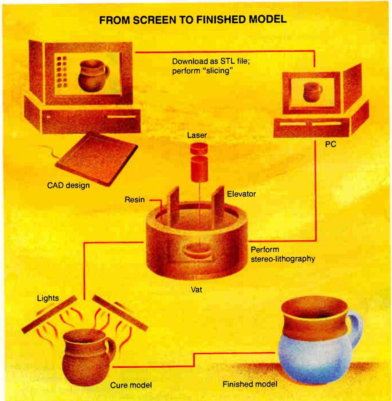
*Rapid automated prototyping, a technology that is now available on microcomputers and workstations, lets you build prototypes from solid-model CAD drawings—just as you use a printer to create 2-D printouts of screen images.*
