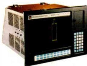
**Mission Critical Workstation 1448:** Combines a CRT and CPU into one rugged NEMA-4 system with 9 option slots and 2 drive bays. A complete 386SX system from \$7395.
