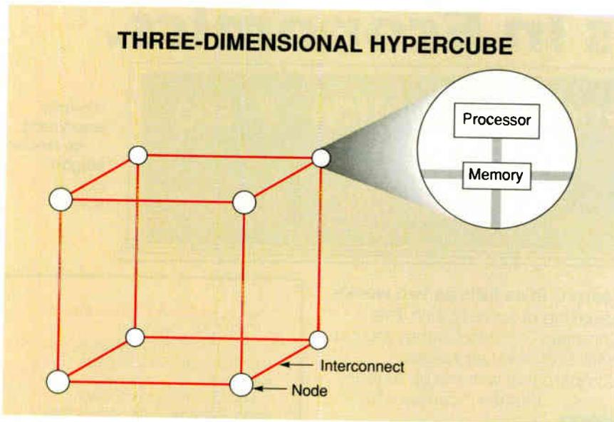
**Figure 3:** A three-dimensional hypercube has the logical structure of a cube, with each node containing a processor, local memory, and connections to three other nodes (see inset). The edges of the cube represent the interconnections. The longest transmission path between any two processors—the communications diameter—need involve only three processors (excluding the sender but including the receiver).
