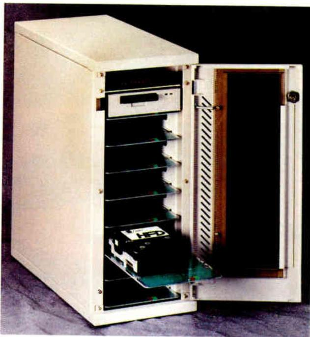
*With the Legacy HFD storage subsystem and complementary RAID software, you can store up to eight backup devices and replace a failed drive without downtime.*
