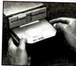
You install the 1.2 meg, 5-1/4" floppy disk drive, learning disk drive operation and adjustment. Later, you dramatically improve your computer's data storage capacity by installing this powerful 20 meg hard drive.
