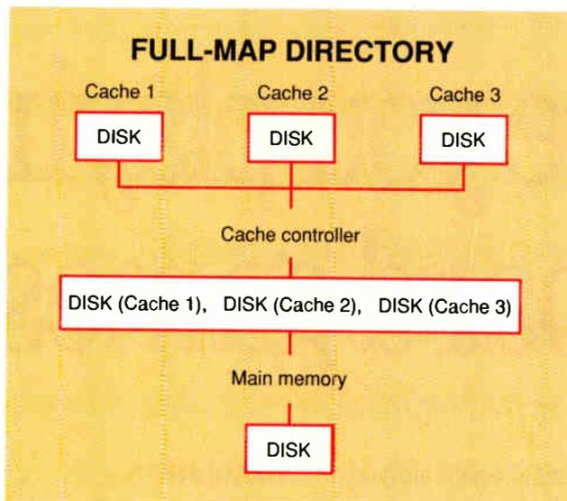
**Figure 1:** In a full-map directory, every cached block has a record and a pointer in the cache controller. The record includes status flags that indicate whether you can write to the block and whether it is a valid block. The costs for a centralized cache directory are primarily memory overhead, more controller processing demands, and communications bottlenecking.
