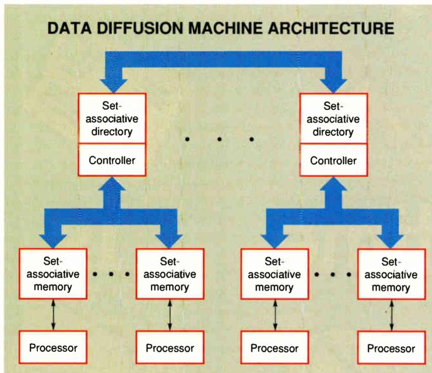
**Figure 7:** The Data Diffusion Machine uses the original GigaMax tree architecture but divides the shared memory among the processors. More important, it turns to virtually, rather than physically, addressed memory, using set-associative memory and directories.
