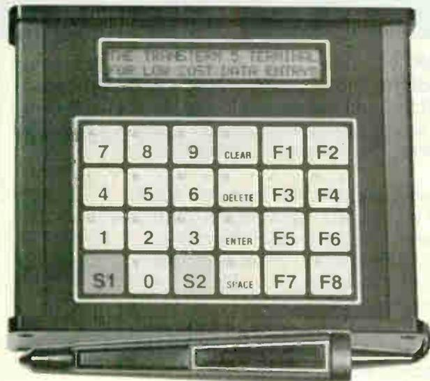
The TransTerm 5 is a work station data entry/display terminal for on-line shop floor data collection into PC/AT based systems. The unit is one of a family of such terminals which feature LC displays for operator prompting and data entry via a membrane keyboard or an optional barcode wand (Code 39). A multi terminal polling controller (up to 250 stations) and a dBASE III+ compatible software package are also available. System costs below \$300.00 per station. Call for info.
