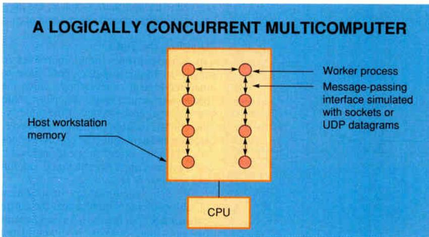
**Figure 2:** Developing a multicomputer system that runs on  $n$  processors requires that you first create a logically concurrent description and cast it into a process-structure graph. Here, an eight-process system is organized as a line of processes. The processes are debugged in a single address space using message passing. This verifies that the system will not deadlock when ported to the multicomputer.
