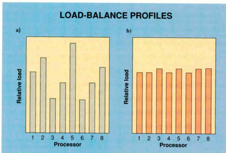
**Figure 4:** (a) A strong load imbalance will produce a poor increase in performance when performed on a multicomputer. (b) By contrast, a near-perfect load balance will produce linear improvements in performance. (Note that the y axis elements are not labeled because specific numbers are not being shown.)
