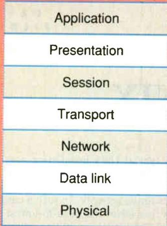
*The seven layers of the OSI model for networks are designed to make the specification endure many changes in technology.*
