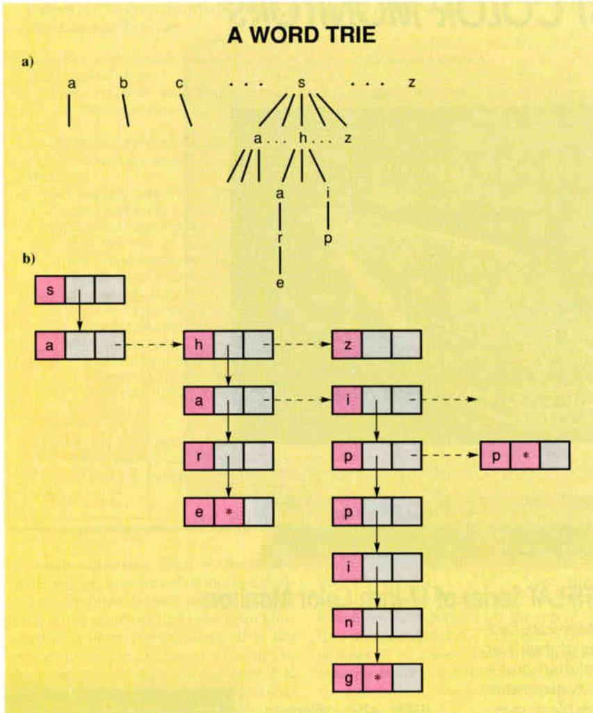
**Figure 2:** (a) A trie—26 trees, one for each letter of the alphabet, and each node containing a single letter. The path from the root defines a word. Each node that represents an indexed word contains a pointer to a list of file numbers. (b) The pointer structure of the trie. (The asterisks stand for pointers to a list of file numbers; the empty boxes could be pointers to other nodes; the dashed lines indicate the omission of a few nodes for clarity.)
