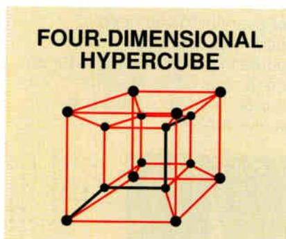
**Figure 4:** A four-dimensional hypercube has the logical structure of a tesseract. It has 16 processors, each with connections to four other processors. The communications diameter is 4.
