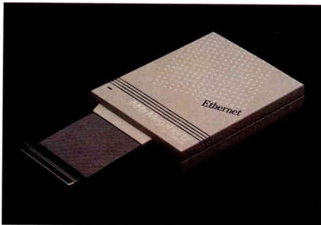
The external laptop Ethernet adapter connects to the Toshiba's 100-pin bus-expansion connector.
