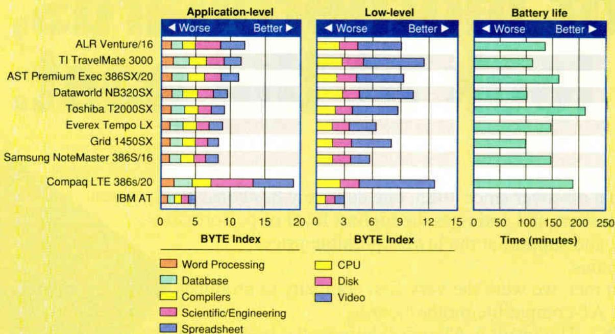
Notebook benchmark results aren't directly comparable with the standard system benchmarks. The battery-life test results are in minutes. For all other benchmarks, the results are indexed and show relative performance; for each index, an 8-MHz IBM AT running MS-DOS 3.30 = 1.
