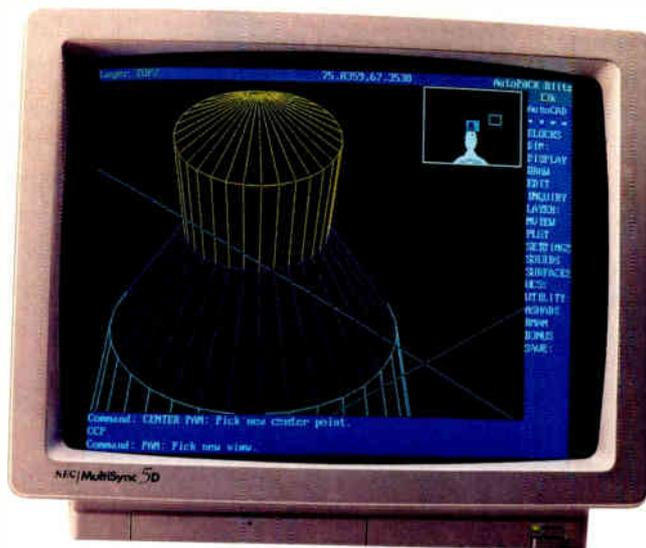
*On a normal VGA display, this CAD drawing would appear jagged. But AutoPack Blitz, which uses Edsun Labs' technology, displays the drawing at a virtual 2048- by 2048-pixel resolution.*
