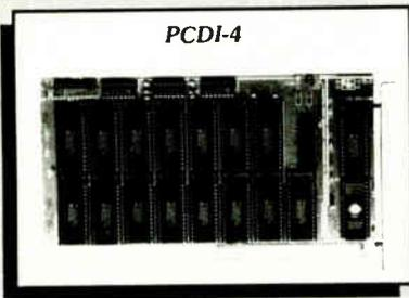
How would you like disk access times measured in the nanoseconds instead of milliseconds? Performance like this is possible with GTEK's newest product, a *solid state disk emulator*. The **PCDI-4** can hold up to 4 Megabytes of non-volatile memory which DOS can access as a disk drive. On board BIOS provides the driver, just plug it in and go! It can even be used as the boot disk. This rugged solid state disk is perfect for harsh environments where a hard disk just won't do!
