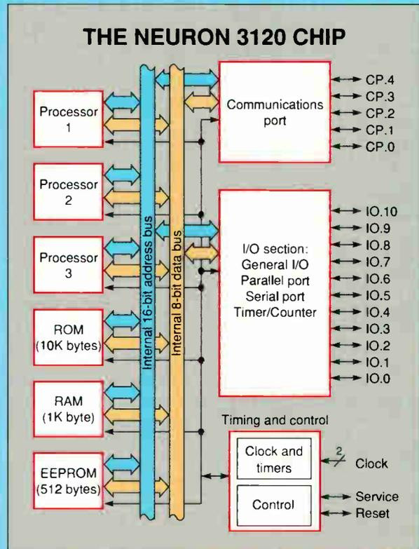
*The first member of the Neuron chip family is the 3120 chip. The 3120 contains three processors: two dedicated to LONTalk (the network protocol used by Neurons) and one designed to be used by the chip's application program.*
