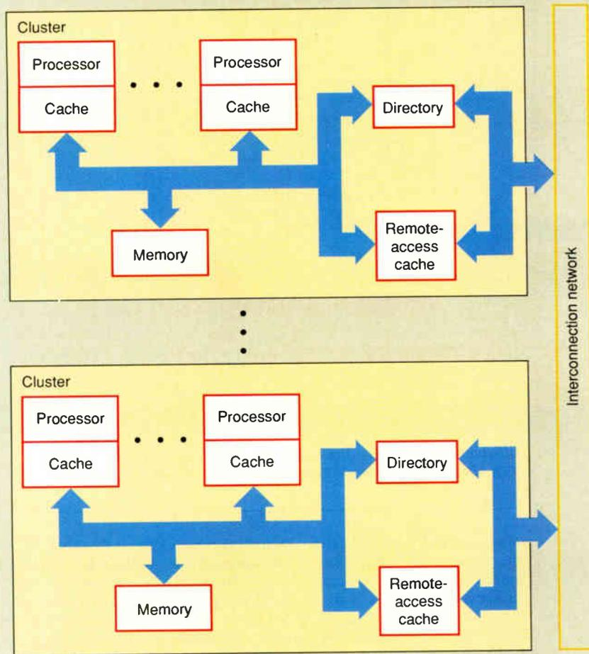
**Figure 4: DASH uses a simple two-level hierarchy, with a bus connecting processors and their caches with each other, local memory, and a second-level cache and directory.**
