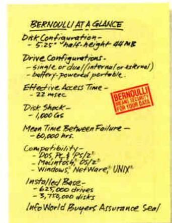
You don't have to pamper a Bernoulli. Its patented design flies a flexible disk precisely under the read/write head. Should your system encounter a bump, air impurity, or power loss, the disk simply falls away. The result? Hard-disk performance without the risks.
