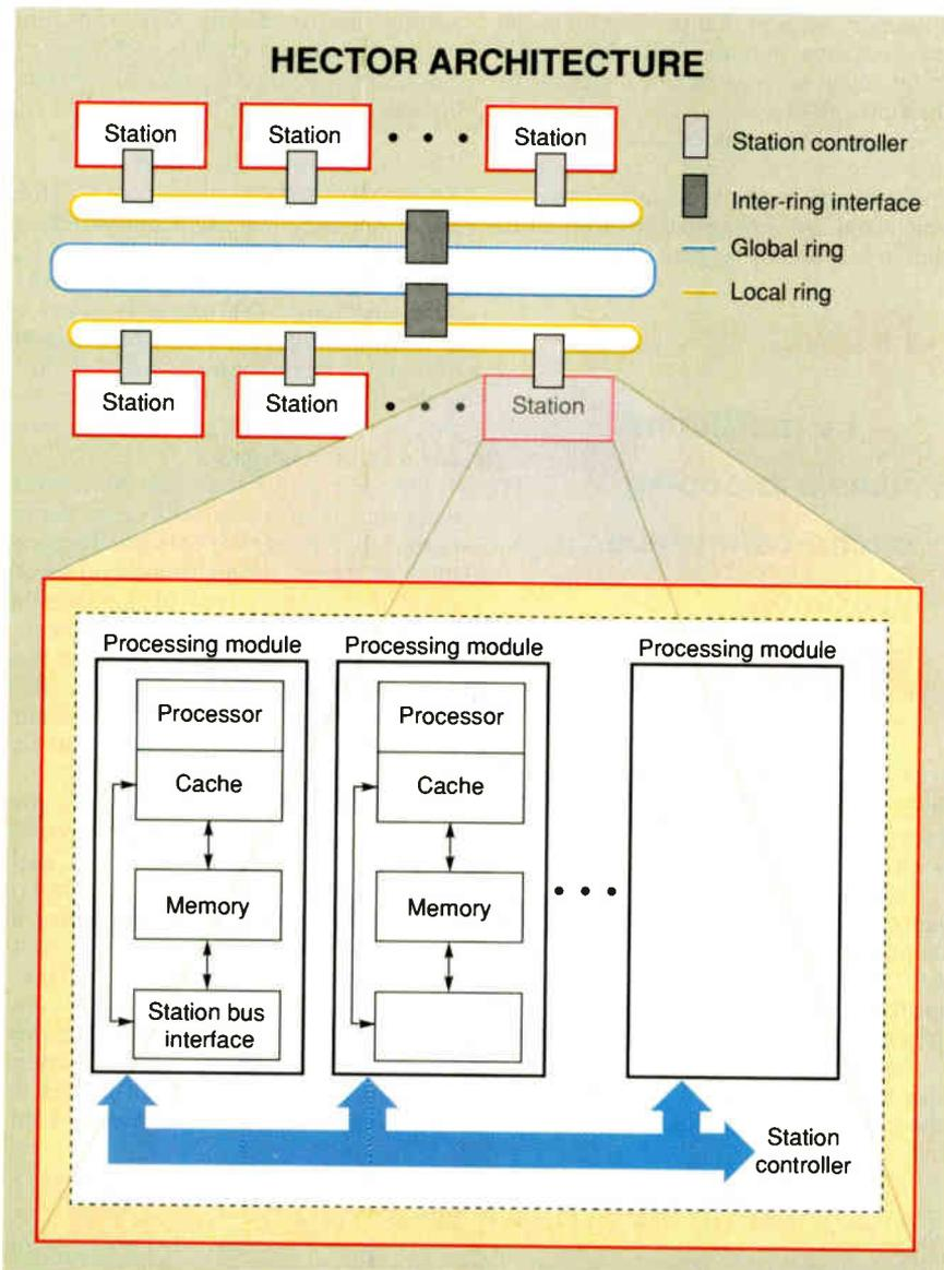
**Figure 3:** Hector opts for a hierarchical arrangement in which the top two levels use rings for the interconnections. The processing node (see inset) includes an interface to the station bus and, typically, a processor, cache, and local memory as well.
