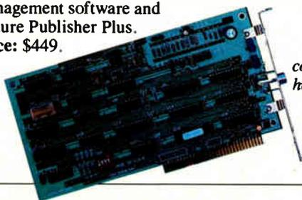
*The VIP 640C's color-enhancement hardware produces real-time display of a video image on any standard VGA monitor.*
