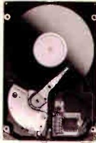
The T2000SX has a 40MB hard disk with 19 msec access time.
