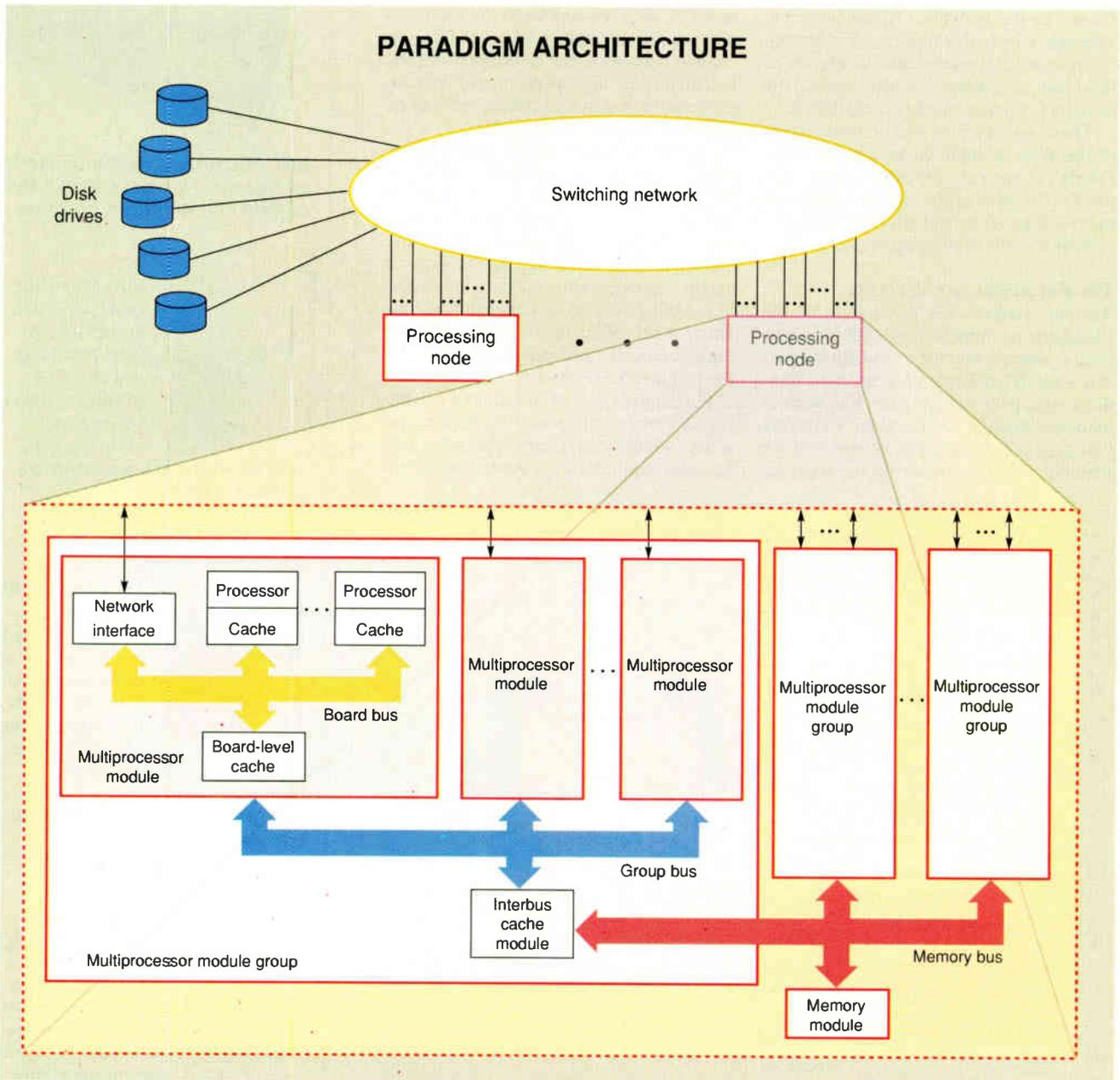
**Figure 5:** In Paradigm, high-level groups of processors, called nodes (see inset), are linked to a switching network. The links, however, are not central nodal links; instead, they connect multiprocessor module groups—the second level down in the hierarchy—to the network, eliminating some bus traffic.
