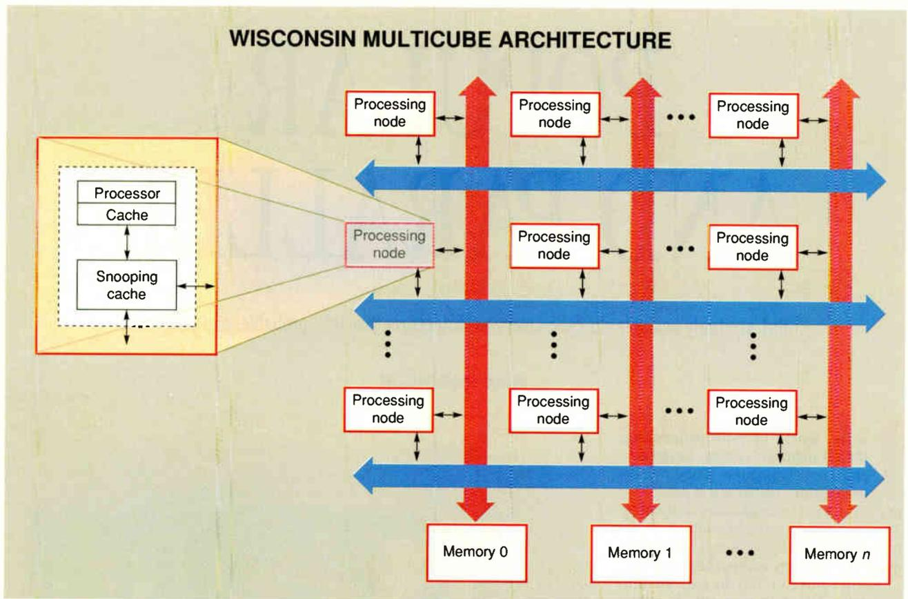
**Figure 1:** The Wisconsin multicube is a special case of a multicube architecture in which a grid of buses interconnects a highly scalable number of processors. A node (see inset) consists of a high-performance microprocessor (which would probably have its own cache); a separate, conventional cache; and a snooping cache connected to the node's row and column buses.
