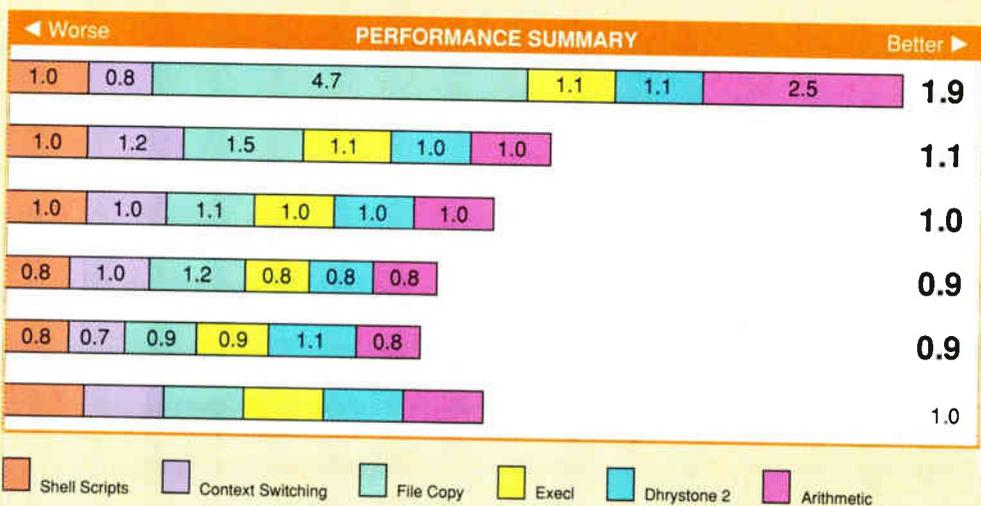
The Solbourne S4000 was a standout in the BYTE benchmark test results due to its performance in the Arithmetic and File Copy tests. For more details on the tests, see the text box "BYTE Updates Unix Benchmarks" at right.
