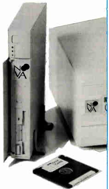
*Base unit supplied with: One Meg Ram, HD/FD Ctrlr, 1.44 Floppy, Monographics, One parallel, Two serial ports, reset 80-250V power supply, 82 keyboard, full one year warranty.*
