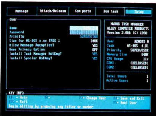
**A**DOS-based multiuser operating system, 386/MultiWare gives remote users a virtual 8086 session on a 386 host. When combined with 386/MultiNode, it provides each session with access to any NetWare LAN. 386/MultiWare allows remote users or attached terminals to share the resources of a single 386 PC. Remote users have access to host memory (including EMS memory) and disk drives. 386/MultiWare coexists with DOS and is very easy to install.
