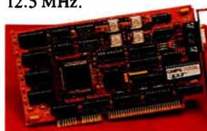
The card's Ultra VGA driver increases the usual 16 or 256 colors on a monitor to 742,813, with near-photographic quality, according to the company. It has a 60-Hz refresh rate and 512 KB of video RAM. Software drivers include Super VGA for Windows 3.0 and Ultra VGA for Windows 3.0 and Autodesk applications.
