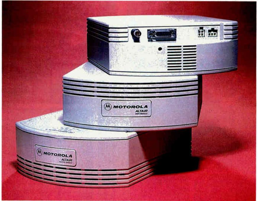
*The Altair system. Shown here are the Control Module (CM) and two User Modules (UM). The grillwork hides a special six-sector microwave antenna. The back panel has connections for power, thin and thick Ethernet, and, on the CM, a special RS-232 cable for UM security registration. Installation can be as simple as placing the unit on your desk and connecting the Ethernet cable.*
