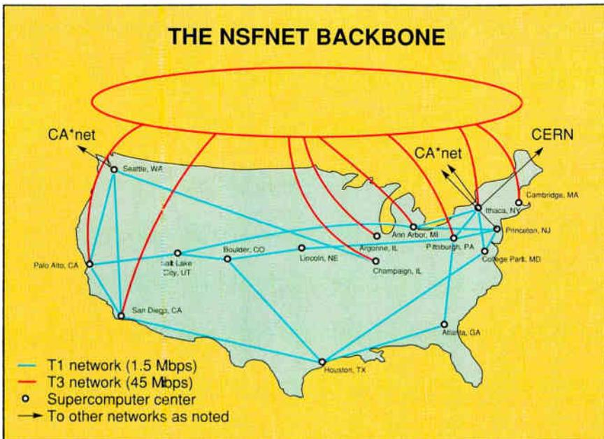
**Figure 1:** With T1 links between 16 supercomputing centers and a T3 cloud in place, the NSFnet backbone and the associated Internet serve most research and educational institutions in the U.S. (Courtesy of Merit Network, Inc.)
