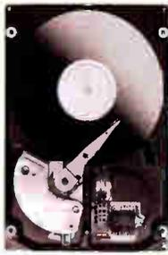
The T2000SX has a 60MB hard disk with 19 msec access time.
