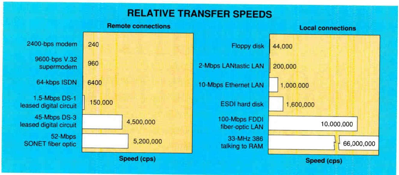
**Figure 1:** When you compare the transfer rates of modems, disk drives, and even high-speed fiber-optic lines with the internal speed of a 33-MHz 386, you can see how far telecommunications still has to go to clear the bandwidth bottleneck: If the 33-MHz bar were drawn without a break, it would be about 10 inches long. (The numbers shown are approximate theoretical raw speeds in characters per second. The scale shown is roughly 1 inch = 6,600,000 cps.)
