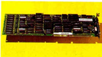
**P**C-Slave/286 cards are single-board computers; each PC-Slave/286 has a 12-MHz 286 CPU with 1 MB of RAM and built-in CGA. These cards do not support extended or expanded memory applications. The PC-Slave/286 cards sell for \$1195 each. With supporting software, a four-user package comes to \$4929. Unlike Cubix and J&L Information Systems, Alloy doesn't offer a 386SX processor board.
