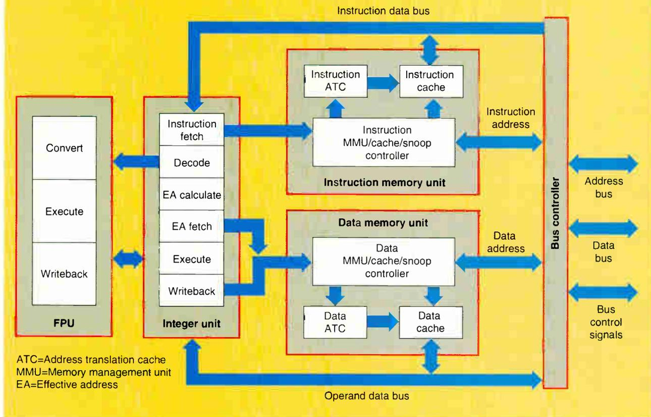
Figure 1: The caches, floating-point processor, and MMU are built onto the 68040. (Source: Motorola, Inc.)
