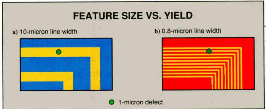
**Figure 2:** Whether a wafer defect constitutes a flaw in a chip depends on the feature size. A chip with 10-micron metallization line width will be essentially unaffected by a 1-micron open-circuit flaw (a), whereas the same defect will kill a chip with denser circuitry (b).
