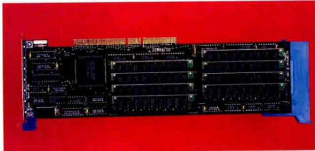
*The self-configuring OS/RAM32plus provides up to 128 MB of extended and expanded memory in one slot.*
