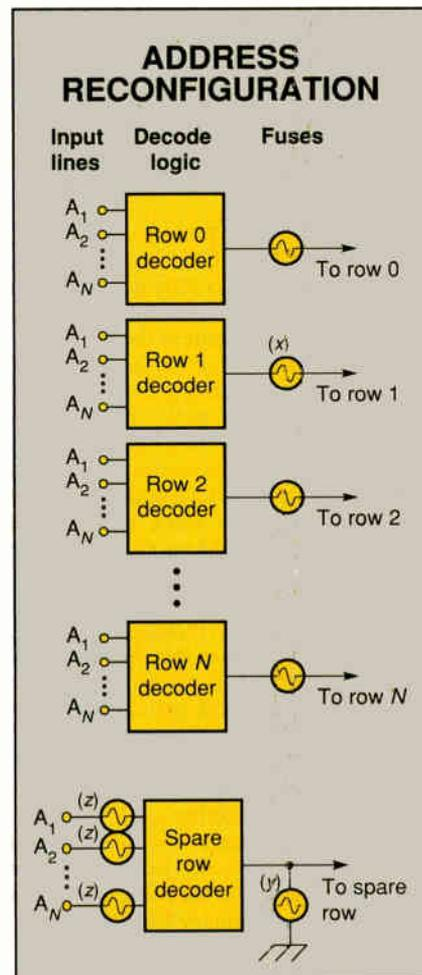
**Figure 3:** This arrangement of fuses for reconfiguring memory has the advantage of not affecting the memory's speed. Breaking one of the main array output fuses (x) will disable that line. Breaking one of the spare output fuses (y) will enable that line by removing a short circuit to ground. The fuses on the input of the spare line decoder (z) can be broken selectively to program the spare line so that it responds to the address of the line that was disabled.
