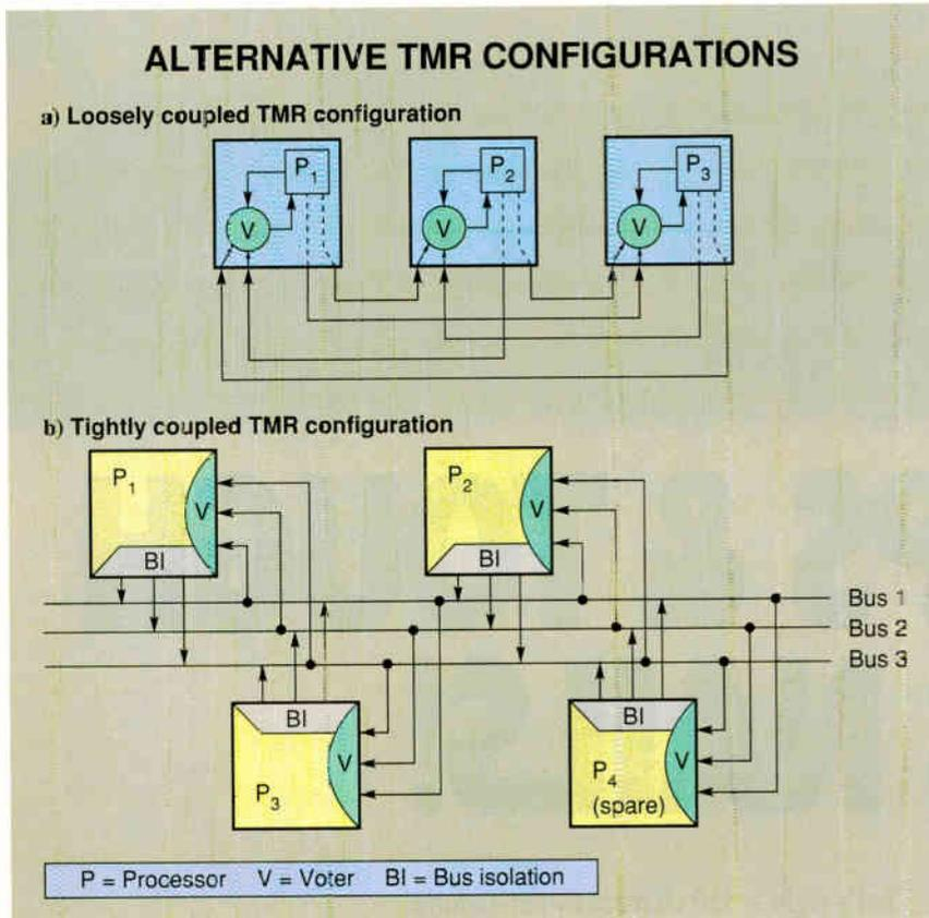
**Figure 2:** (a) In a loosely coupled TMR configuration, software performs the voting. (b) In a tightly coupled TMR configuration, processors are each assigned to drive one bus through their bus-isolation logic and read all three buses via their input voters.
