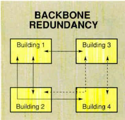
**Figure 1:** Providing increased fault tolerance is often a matter of redeploying network assets or making modest investments in equipment. Here, the backbone between the four buildings can be made completely redundant by adding two links (dotted lines).
