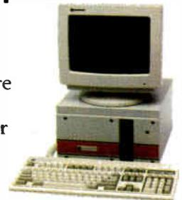
*Mission Critical Benchtop 2003: With 10 option slots and 2 drive bays the 2003 makes desktop computing possible in extreme environments. A complete 386SX system from \$3950 without monitor.*
