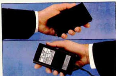
TOP: Rechargeable Ni-Cad battery weighs 1.05 lbs.
