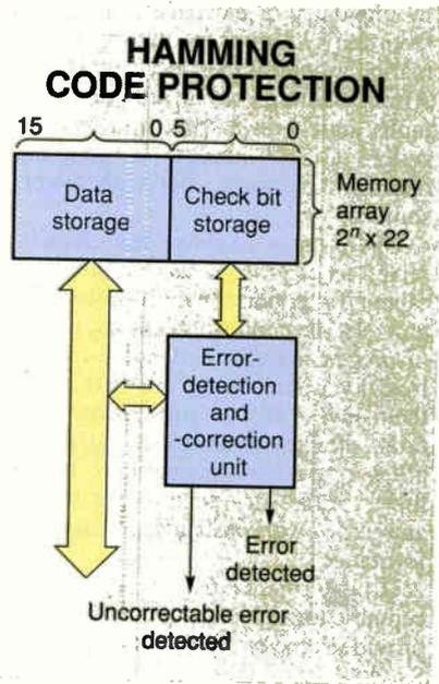
Figure 4: A 16-bit memory array protected by a Hamming code. Six check bits enable single-error correction and double-error detection.
