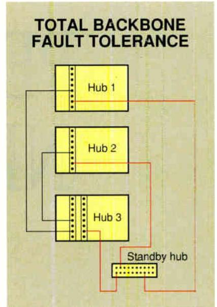
**Figure 2:** Making a backbone truly fault tolerant requires redundant hubs as well as redundant cabling. The standby hub ensures that the link between any two primary hubs will not be lost if the third hub goes down.
