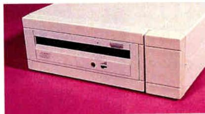
The Toshiba TXM-3201A1 was a leader in many of the benchmark tests. However, it was also the most feature-poor of the drives. It has a standard SCSI adapter and came bundled with a Future Domain TMC-840 card, which allows you to configure among four base addresses and two interrupts and set the time-out delay. I also ran the drive under the TMC-845 card with the Hitachi drivers. I noticed a slight performance improvement with that combination.
