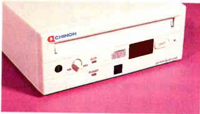
What the Chinon CDC-431 lacks in speed, it almost makes up for in features. Despite a rated access time of 350 ms, the Chinon gains the dubious honor of running dead last in most of the benchmark results.
