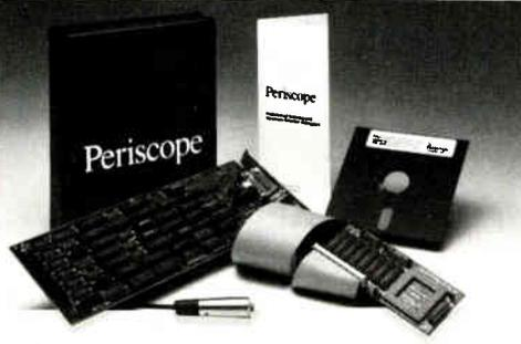
Real-time Periscope Model IV, shown with new 33MHz board and 486 pod.
