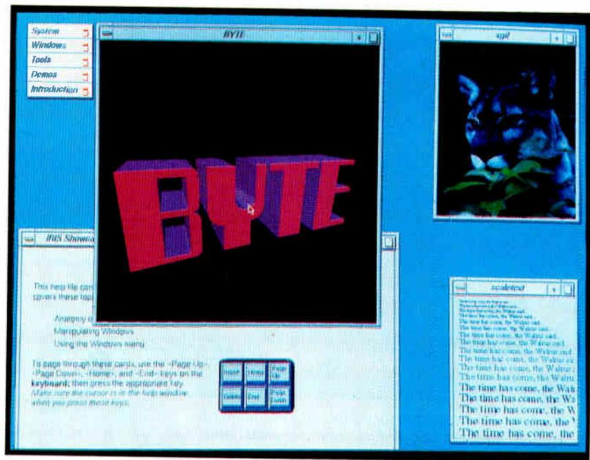
The BYTE logo is written using the standard SGI Graphics Library. Gouraud shading generates 24-bit-color requests that are approximated by hardware dithering to 8-bit color. The xgif file is a standard X Window System application showing the quality achieved with standard 8-bit color. The "scale test" box is displaying the results of PostScript code.
