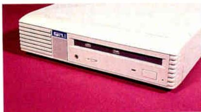
Peripheral Land's drive is a Sony CDU-541-1 mounted in an enclosure designed to fit beneath the chassis of a Mac SE. PLI's Macintosh orientation is evident in the manual (which avoided the subject of PC installation), in the omission of both a device driver and MSCDEX, and in a
