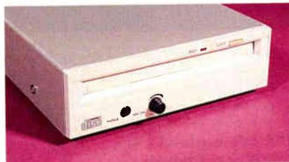
Although the Texel DM-5021 placed in the middle of the benchmarks, it does support continuous reads, and the test animation displayed smoothly. Missing from the drive were RCA jacks and an emergency-eject mechanism.
