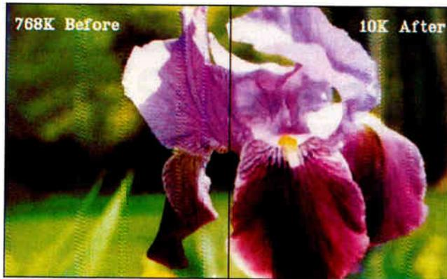
*Iterated's P.OEM compression technology uses fractal transforms to compress images. The uncompressed image at left consumes 768K bytes. The compressed image at right consumes 10K bytes.*
