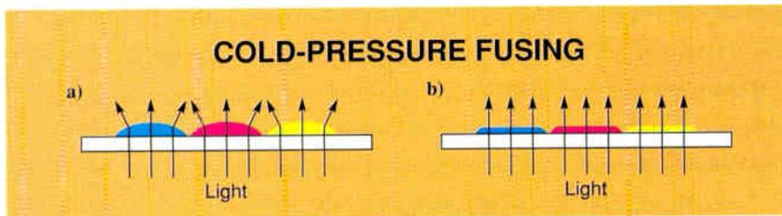
**Figure 3:** (a) Without fusing, solid-ink droplets from phase-change ink-jet printers remain rounded on the surface. On an overhead transparency, this shape diffracts light away from the projector, resulting in a black-and-white projected image. (b) With fusing, the ink droplets are flattened, and the light proceeds normally to the projector, resulting in good-quality overhead transparencies.
