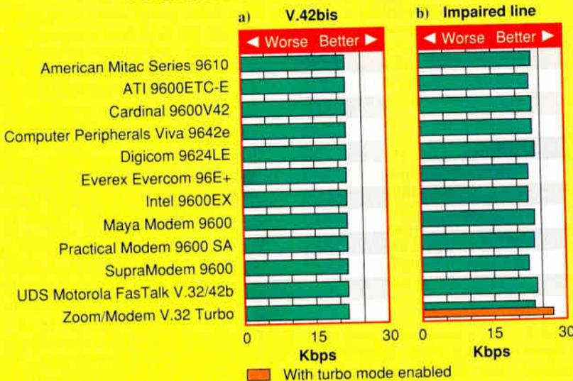
Effective throughput is measured under various conditions. (a) Each modem performed equally well when connected to a Hayes Ultra V-Series modem using V.42bis compression. (b) The UDS Motorola FasTalk V.32/42b proved to be slightly faster than the other entries using a V.32 connection over impaired lines. However, the Zoom/Modem V.32 Turbo's turbo (12,000-bps) connection gave it the highest overall throughput when two Zoom/Modems were connected.
