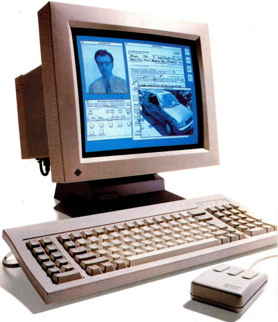
*The new \$4,995 SPARCstation ELC gives you more than twice the power of our previous entry-level monochrome workstation: 20.3 SPECmarks from a single 33-MHz chip that performs both integer and floating-point calculations. Load it with up to 64 MB of memory, and up to 5.2 GB of external storage.*
