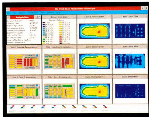
*The Circuit Board Thermometer for Windows shows a completed circuit-board thermal analysis. The program supports multiple viewing of data.*
