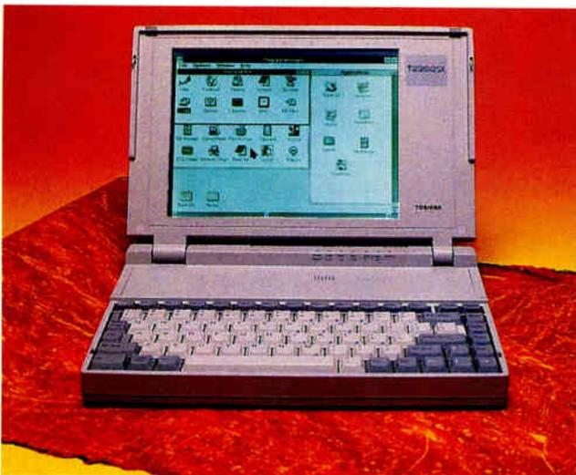
**T**he Toshiba T2200SX notebook computer is a refreshing addition to the notebook computer industry, not because of any astounding technical innovation, but because of important refinements. I looked at a "commercial sample" of Toshiba's new system and was impressed by the combination of technology and attention to detail that it represents.
