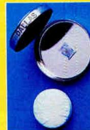
DS199 Touch Memory comes in a steel container called a MicroCan that has a peel-and-stick adhesive backing. The metal housing serves as the
