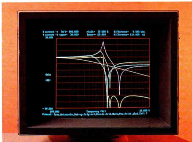
*AFD-Plus 3.0 lets you explore multiple design alternatives, create complex filter prototypes, and revise existing active-filter designs.*
