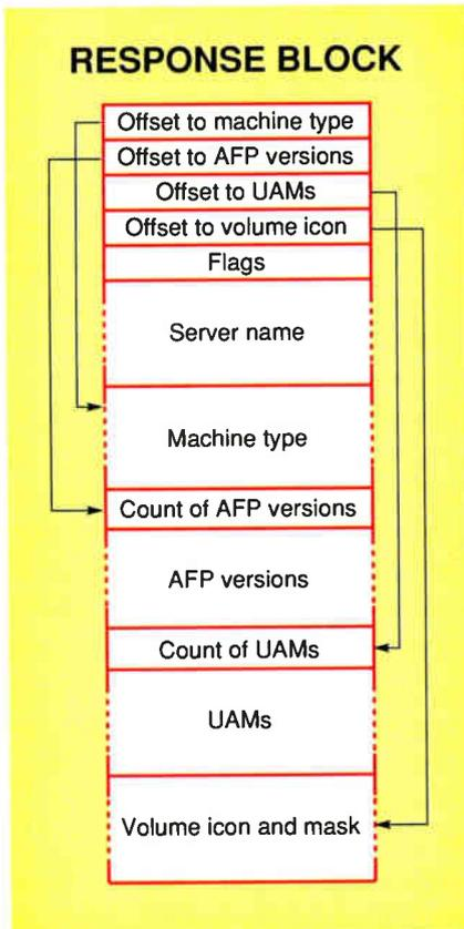
**Figure 2:** The format of the response to an `FPGetSrvrInfo` command. All offsets are 16-bit values, while the counts are 8-bit values. The flags value is also a 16-bit word, the low 2 bits of which are significant: Bit 1 set indicates that the server supports the `FPCopyFile` command, and bit 0 set indicates that the server supports `FPChangePassword`.
