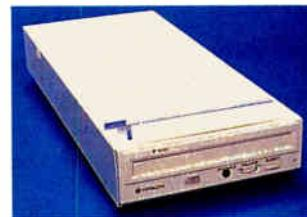
cleaning. The TCDR-6000 can daisy-chain as many as eight drives on a single interface card. The unit uses a High Sierra/ISO-9660 CD and has a double-door cartridge compartment. **Price:** \$805. **Contact:** Todd Enterprises, Inc., 224-49 67th Ave., Bay-side, NY 11364, (800) 445-8633 or (718) 343-1040; fax (718) 343-9180. **Circle 1280 on Inquiry Card.**
