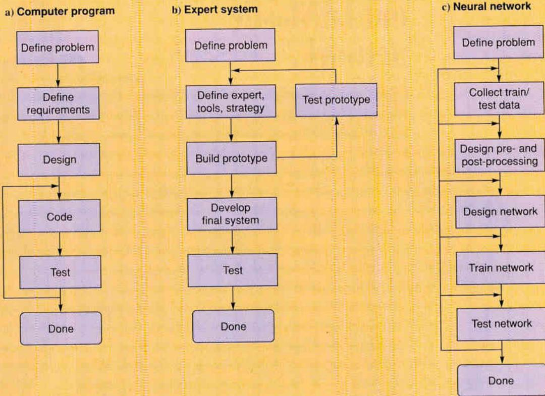
**Figure 2:** You develop computer programs, rule-based expert systems, and neural networks using quite different procedures. Rule-based development generally follows a rapid prototyping model. In a neural-network application, you spend more effort collecting data and determining the correct preprocessing technique.
