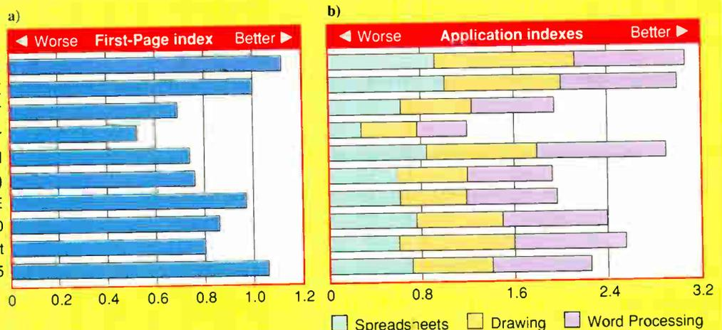
*From click to klunk: (a) The first-page index tracks printer performance on a single text page. We started timing when the printer first received PostScript commands and stopped timing when the page fell into the output tray. Expect this type of performance for memos and simple business correspondence.*
