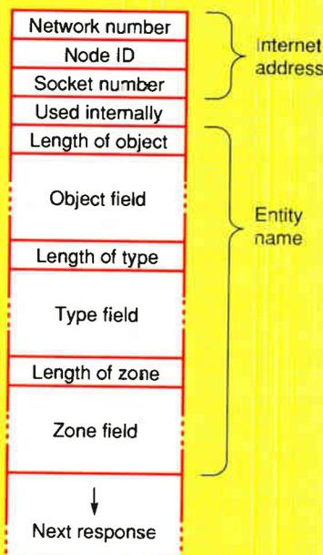
**Figure 1:** The format of a single-response entry from the NBP `LookUpName` command. Each item in the internet address portion is a byte, except for the network number, which is a 16-bit value. Note that the elements of the entity name are counted strings.
