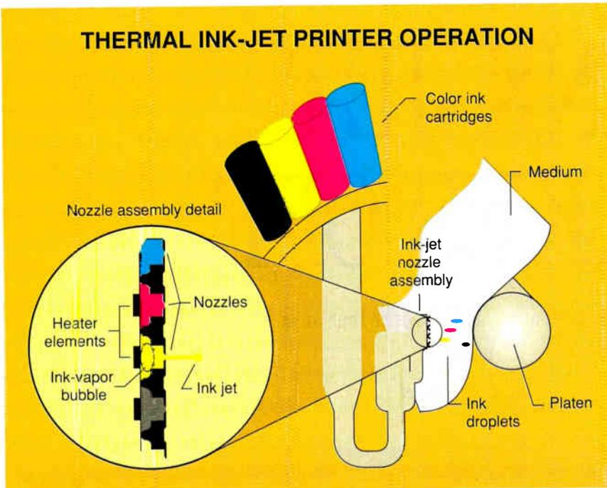
**Figure 1:** Thermal ink-jet printers, the so-called bubble jets, work by heating a drop of ink until it forms a vapor bubble. The bubble forces the ink out of the nozzle and onto the paper.
