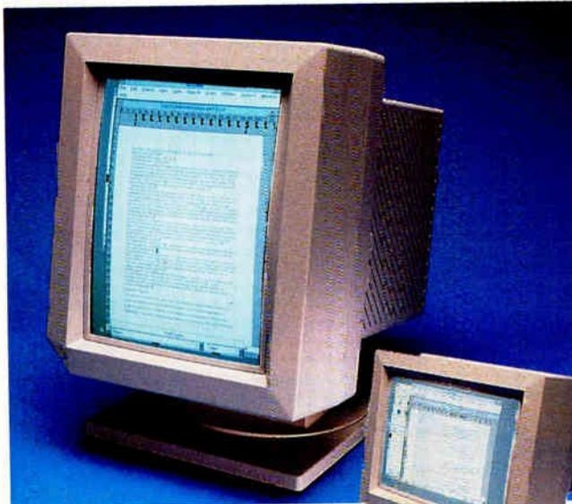
It doesn't take long for a Windows 3.0 user to realize that your garden-variety VGA resolution on a standard-size (i.e., 13- or 14-inch) monitor just won't cut it for serious use. A resolution of 640 by 480 pixels on a small screen offers little more than a small peek at a piece of a desktop.
