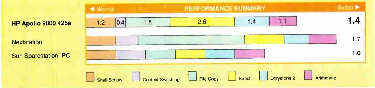
The graph above summarizes the results of BYTE's Unix benchmarks (version 3). We index the results to show relative performance; for all tests, a Sun Sparcstation IPC=1. The cumulative index is formed by summing the indexed performance results for the individual tests. The tests show relative performance for running a shell script with eight concurrent scripts running, pipe-based context switching, file copy throughput (in 5 seconds),
