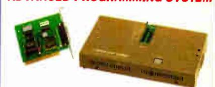
A NEW UNIVERSAL PROGRAMMING SYSTEM FROM MODULAR CIRCUIT TECHNOLOGY. USES APPROPRIATE ADAPTORS (OPTIONAL) TO PROGRAM MULTIPLE DIP DEVICES AS WELL AS PLCC AND PGA PACKAGED DEVICES.
