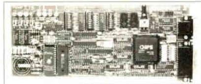
On-board switches, LEDs, and digital displays allow complete control over testing in systems lacking video or disk (ideal for motherboard or system burn-in).
