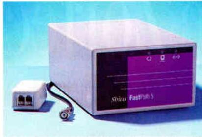
**Photo 1:** Shiva's FastPath 5 LocalTalk-to-Ethernet gateway supports AppleTalk Phase 1 and 2, TCP/IP, and DECnet Level 1 protocols. Rather than implementing an NFS gateway within the FastPath, Shiva bundles a copy of InterCon's NFS/Share NFS client, which runs on each Mac.
