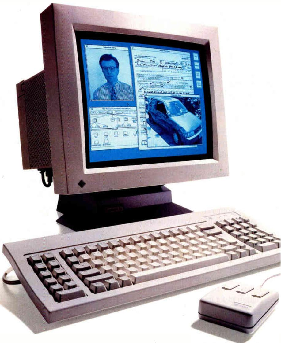
*The new \$4,995 SPARCstation ELC gives you more than twice the power of our previous entry-level monochrome workstation: 20.3 SPECmarks from a single 33-MHz chip that performs both integer and floating-point calculations. Load it with up to 64 MB of memory, and up to 5.2 GB of external storage.*
