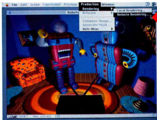
**Ray Dream's Designer** is a solid modeling-cum-ray-tracing application. It has the ability to hand off the computationally expensive ray-tracing portions of a job to other networked Macs. It does this by using System 7.0's built-in file sharing and Apple event mechanisms.
