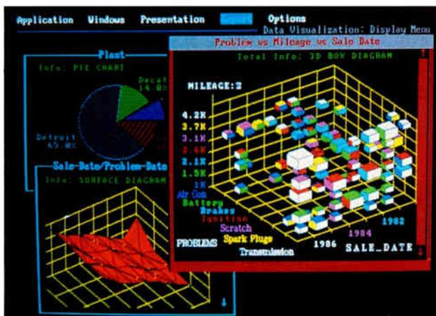
The Database Visualization Tool automatically displays database files in 2-D and 3-D graphics using numeric and nonnumeric data.
