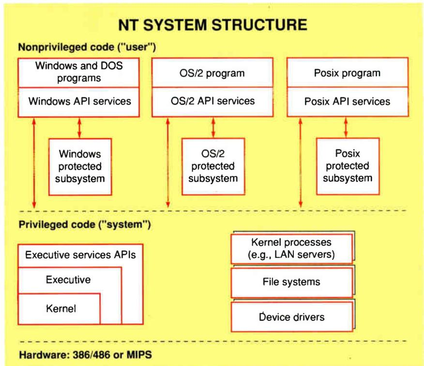
*The ambitious layout of Microsoft's New Technology (NT) portable system software, designed to run on both Intel 80x86 and Mips Computer Systems RISC processors. The microkernel approach allows the basic functions of the operating system to be isolated in the Executive kernel, which Microsoft says will take up only 50 kilobytes of memory.*
