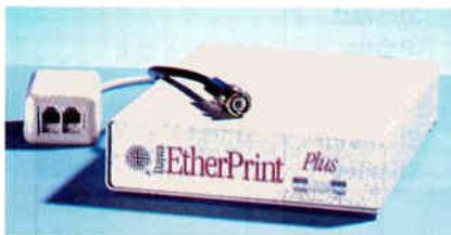
Photo 2: Dayna's EtherPrint Plus links Ethernet-bound Macs to printers on LocalTalk.
