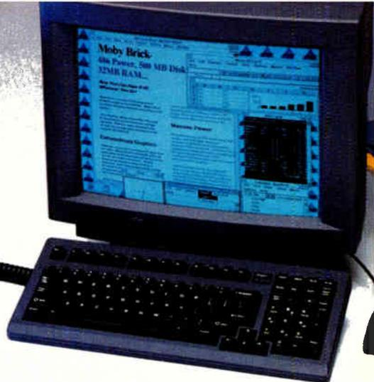
**33MHz 486, 510MB Hard Disk, 32MB RAM, 1024 x 768 VGA, only 8.7 lbs.**
