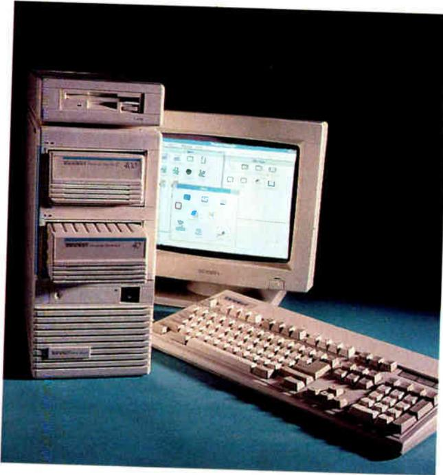
actly to your needs. Need a more powerful processor? Plug in a new card. A larger hard drive? Plug in a new Pac. You can even add a second dock for an additional Pac. Even the floppy drives are modular. If you need a second one, it snaps on atop the PacII's case.
