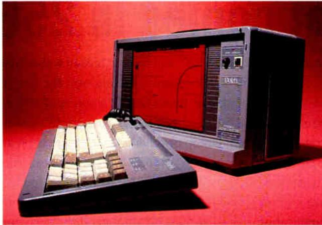
The 486-50E comes standard with a Conner Peripherals 200-MB SCSI hard drive and a 3½-inch 1.44-MB floppy drive. There's no room to add further storage, but you can buy the machine with a larger hard drive. I found the 200-MB drive and the 4-MB caching controller to be an effective combination.
