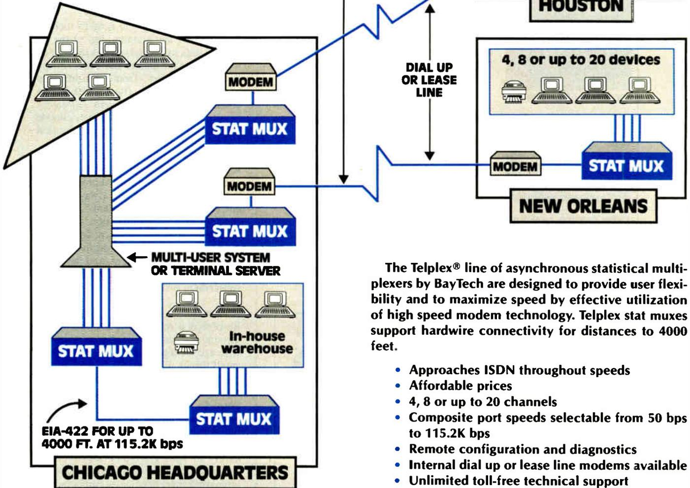
The Telplex® line of asynchronous statistical multiplexers by BayTech are designed to provide user flexibility and to maximize speed by effective utilization of high speed modem technology. Telplex stat muxes support hardwire connectivity for distances to 4000 feet.
