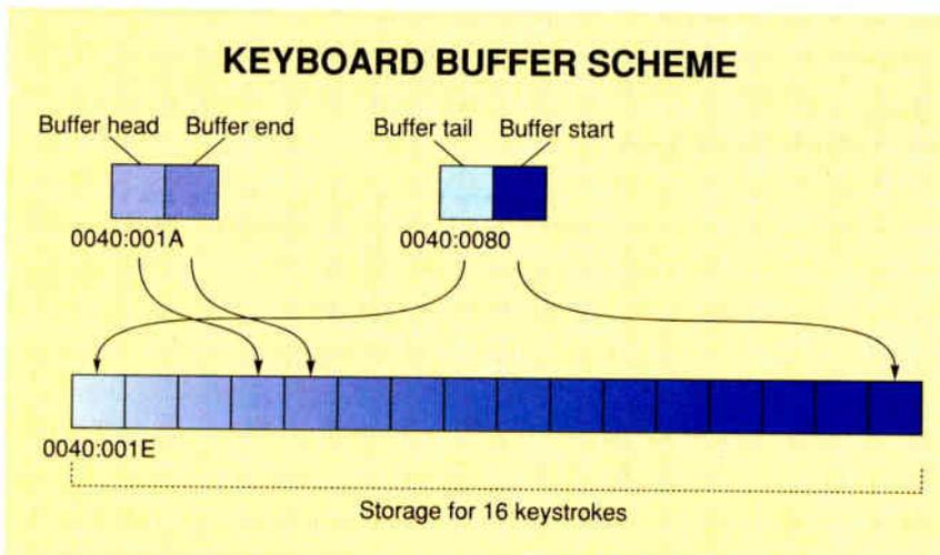
**Figure 2:** The keyboard buffer has storage for 16 keystrokes, two pointers to the head and tail of a circular buffer, and two more pointers that determine the physical buffer boundaries. The ROM BIOS normally handles the buffer stuffing as part of the keyboard hardware interrupt, but you need to do it yourself if you're running on an old machine. Newer BIOSes have function calls to place data in the buffer.
