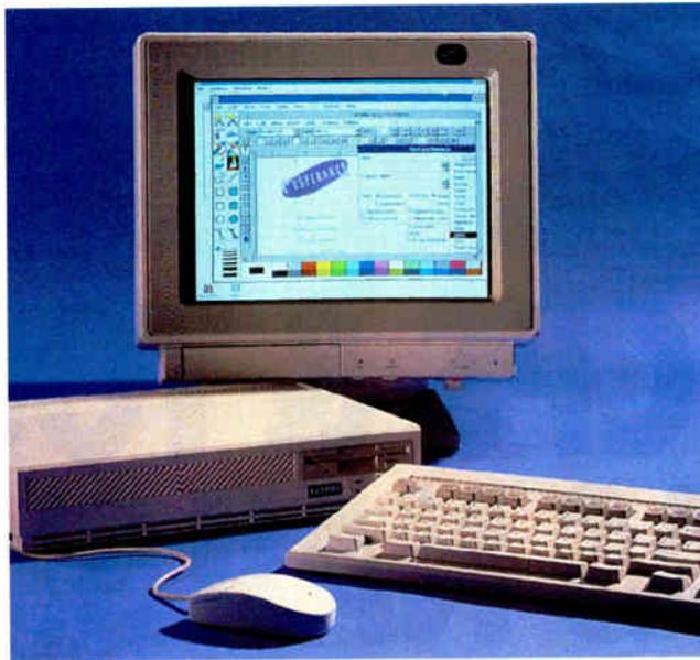
top-of-the-line model. It includes 32 MB of RAM, a 3½-inch 426-MB SCSI hard drive, an 8514/A graphics card with integrated VGA and support for 1024- by 768-pixel noninterlaced resolution, 1 MB of video RAM, and a 15-inch Super VGA color monitor.
