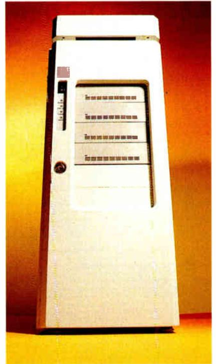
**T**angent has added a formidable competitor to the file-server market with its 486-based Multi-Server. The processor runs at 33 MHz and takes advantage of a standard 256-KB SRAM cache. Although the Multi-Server can use only a single CPU, it addresses the I/O bottleneck issue elegantly with the powerful combination of EISA bus mastering and a SCSI-2 interface. The unit we received carried 16 MB of memory, four 165-MB SCSI drives, two SCSI controllers, and a price tag of \$14,500.
