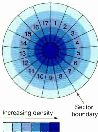
**Figure A:** Typical hard disks have used variable-density recording, which writes data at a constant rate to a disk rotating at a constant angular velocity. Variable-density recording results in a lower density (and lower storage efficiency) for recorded data on the outer tracks of a disk.
