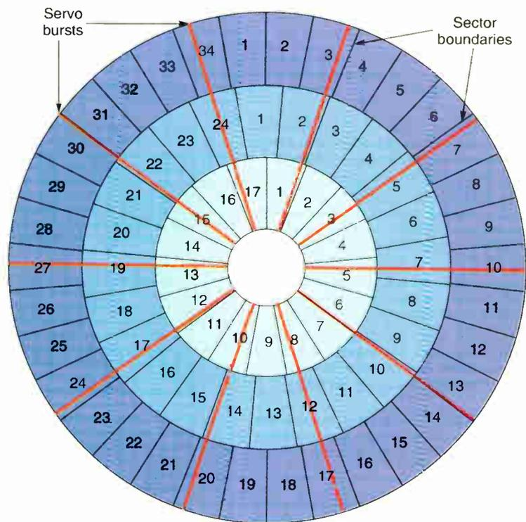
**Figure B:** CDR is a more efficient storage method that is now gaining acceptance. It breaks each disk platter into concentric zones, each with a recording density optimized for it. Because the outer zones are larger in circumference, they can contain more bits. More sectors are recorded in the outer zones than in the inner zones (each sector contains the same number of data bits).
