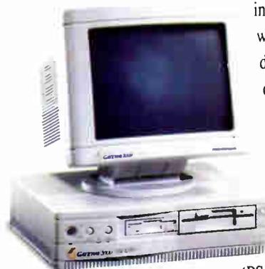
in a small footprint system, we integrated the diskette drive controller, the video chip set and the I/O card on the motherboard, leaving five 16-bit slots open in the standard configuration.
