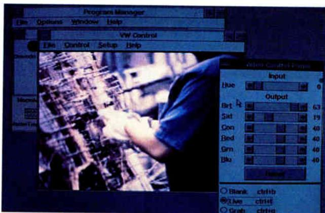
vide access to multiple video sources. On the video-in-a-window side, Bravado does its duty: real-time video in a scalable window, with accompanying audio. It can handle NTSC or PAL signals, and it can save and load "frozen" video and other images to and from disk.
