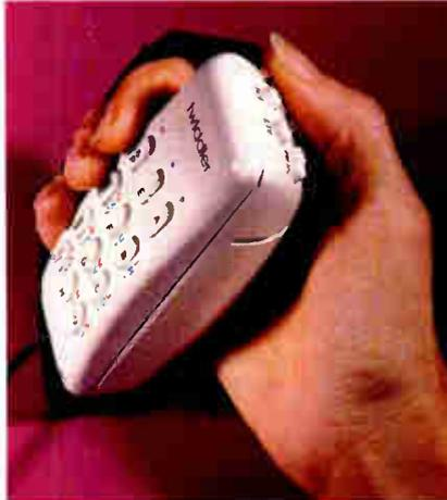
based on an electrolytic tilt sensor that is sealed inside the device. By pressing the mouse button on the top of the unit and pointing with your index finger in the direction you want the device to tilt, you control the cursor on the screen.
