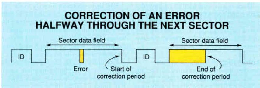
Figure 3: Correctable single-burst errors are typically corrected by the time the disk has rotated halfway through the data sector that follows the sector with the error.
