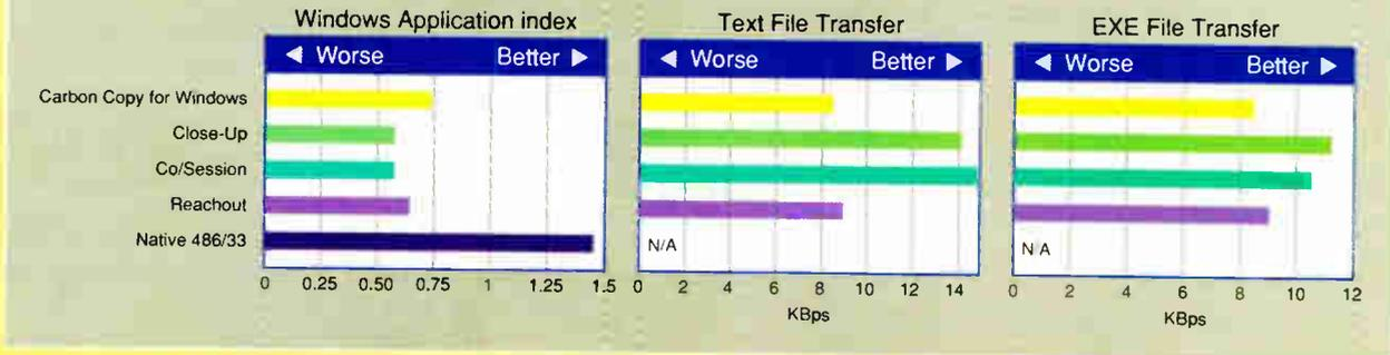
**Figure A:** Carbon Copy for Windows was the fastest at running Windows applications via 9600-bps modem. Close-Up and Co/Session proved to be the best at file transfers. (N/A = not applicable.)
