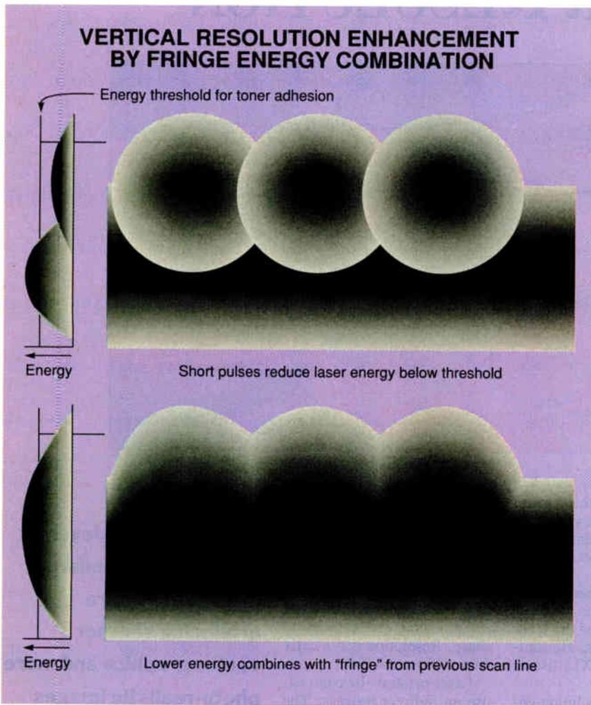
**Figure 1:** A weak pulse of laser light on the upper scan line combines with fringe energy delivered to the lower scan line to fatten the line. The upper part of the diagram shows an ideal situation in which the two scan lines do not interact; the lower part shows the actual, combined effect. (Courtesy of LaserMaster Technologies)
