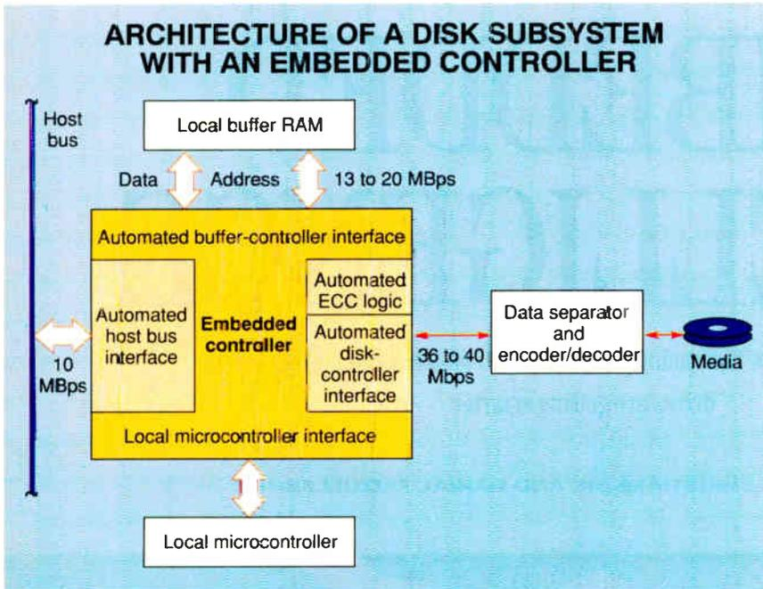
**Figure 1:** The microcontroller is responsible for programming the embedded controller, handling exceptions, and, in single-processor designs, positioning the read/write heads over the desired track and ensuring that they stay aligned. The disk buffer holds data moving between host and disk: it may be DRAM or static RAM.
