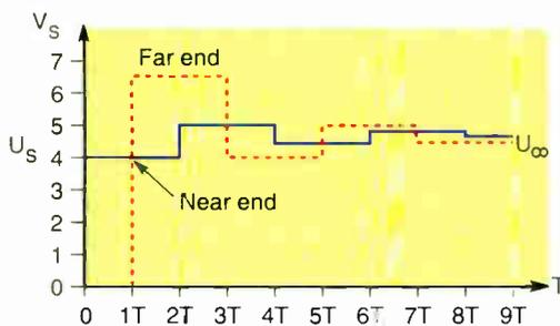
**Figure B:** A logic transition occurs at the near end of a bus at time 0 and arrives at the far end at  $1T$ , with significant overshoot. The overshoot propagates back to the near end and changes the voltage there. The reflections travel up and down, decreasing, until at  $8T$  the bus settles near its final logic level.
