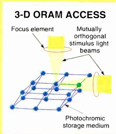
**Figure A:** 3-D ORAMs record information through the excitation of a photochromic chemical dopant. To read a bit, two photons of 1.03-micrometer wavelength provide the necessary stimulus when they strike a data bit.
