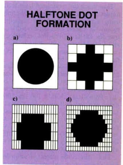
calculate the size of the halftone cell—in this case, 5 by 5 pixels. A 50 percent gray level would fill half of these cells (i.e., 12 or 13).
