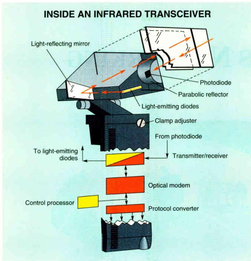
*The components of the Photonics infrared transceiver. The transceiver directs the beam of light to a passive surface, such as the room's ceiling, where the light transmission can be picked up by another transceiver.*
