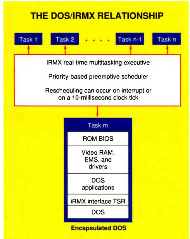
**Figure 2:** DOS runs as an iRMX task like any other in V86 mode. The DOS task contains a normal DOS system complete with drivers, ROM BIOS, and applications. In that same iRMX task, you can initiate Windows just as you would on a dedicated DOS system.
