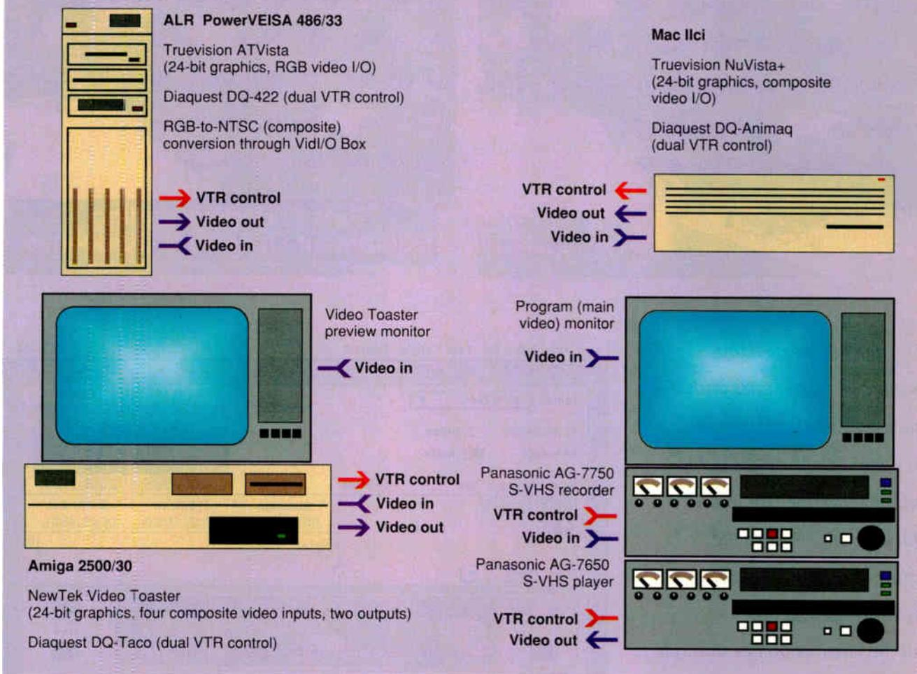
All three systems in the BYTE Multimedia Lab are equipped to handle video I/O. The end of the line is always the video input of the AG-7750 S-VHS VCR. If only the real interconnections were as neat and manageable as in this diagram.
