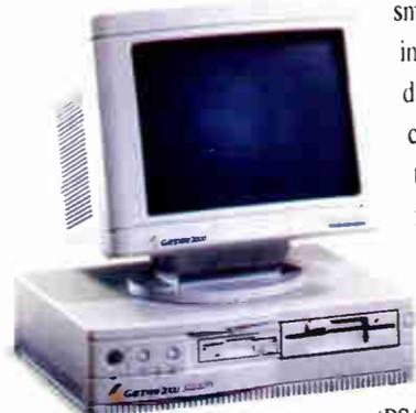
The mini desktop models have a standard mouse port (PS/2 compatible), leaving two serial ports open. RAM on these systems is expandable to 16MB on the motherboard. The Western Digital IDE hard drives feature a 32K read-look-ahead cache buffer. All mini desktop models have Quadtel BIOS and 200 watt power supplies.
