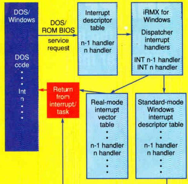
**Figure 4:** Any iRMX task, including DOS/Windows, can initiate hardware interrupts. The system traps DOS/Windows interrupts in Ring 0; reflects them to the appropriate handler, whether real-mode or protected-mode; and then traps the return to route the tasks to the appropriate mode.
