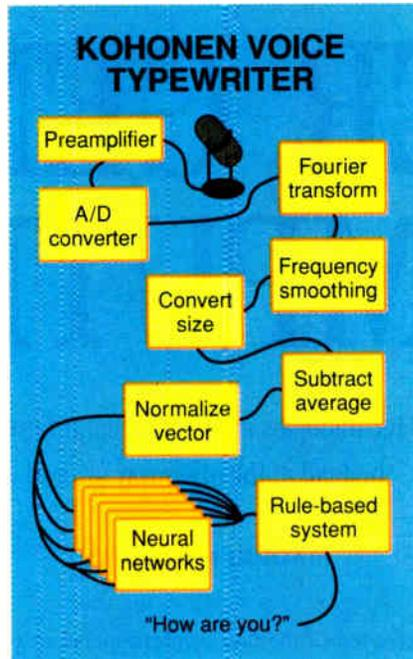
**Figure 1:** *The Kohonen voice typewriter marries conventional digital signal processing with neural networks and rule-based experts to produce an excellent speech-to-text system that responds in about ¼ second with accuracy in the 92 percent to 97 percent range.*
