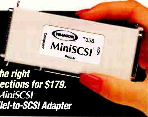
Add a SCSI port to almost any printer port with our pocket-sized, self-contained MiniSCSI. Ideal for laptops, notebooks and systems which can't accommodate a standard SCSI interface, the MiniSCSI also lets you relocate SCSI devices easily.
