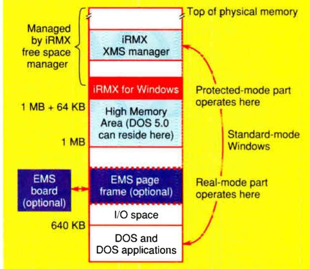
**Figure 3:** How do DOS, Windows, and iRMX share system memory? At first, iRMX has all the extended memory. Then, standard-mode Windows obtains some from an iRMX XMS driver, which functions as a high-memory manager, taking responsibility for its management.
