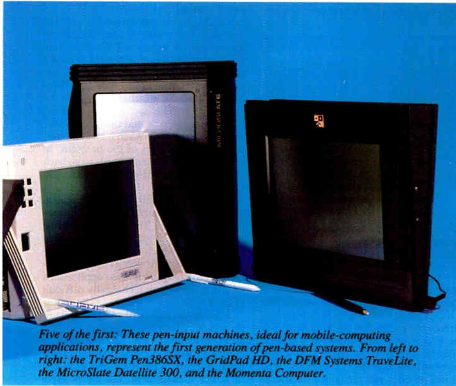
Five of the first: These pen-input machines, ideal for mobile-computing applications, represent the first generation of pen-based systems. From left to right: the TriGem Pen386SX, the GridPad HD, the DFM Systems TraveLite, the MicroSlate Datellite 300, and the Momenta Computer.
