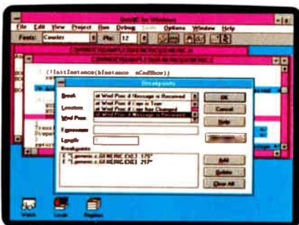
QuickC for Windows supports a wide range of breakpoint types, from breaking at a location to breaking on a Windows procedure when a message is received.
