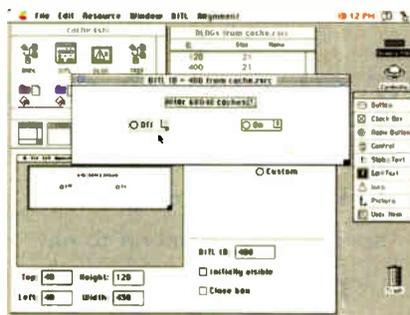
**Screen 2:** The dialog box used to obtain a choice from the user. A mouse-click on either button supplies an item value to the program. All other events are ignored. Note that this dialog box isn't initially visible; the code displays it later.
