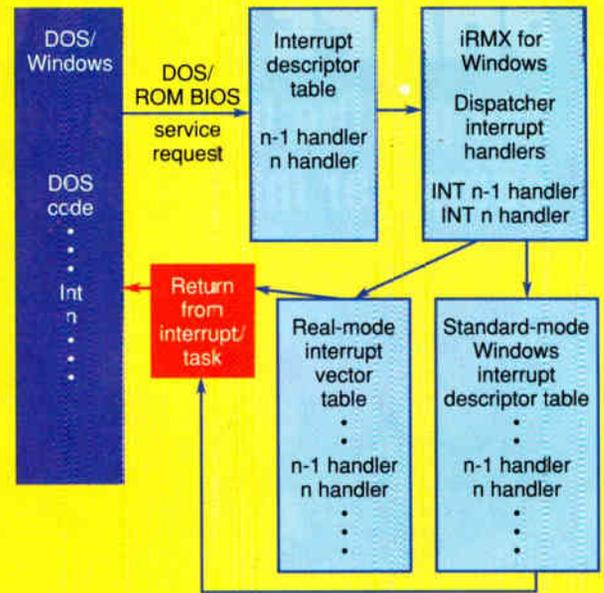
**Figure 4:** Any iRMX task, including DOS/Windows, can initiate hardware interrupts. The system traps DOS/Windows interrupts in Ring 0; reflects them to the appropriate handler, whether real-mode or protected-mode; and then traps the return to route the tasks to the appropriate mode.
