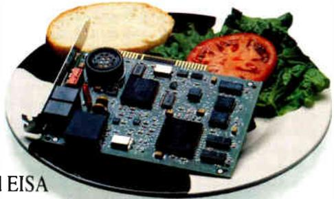
computers. Both ISA and EISA models are based on the Intel486™ DX2 dual speed processor. With a system clock frequency of 25MHz, the internal core of this CPU executes at 50MHz for a 35% increase in performance compared to a 33MHz 486DX system.
