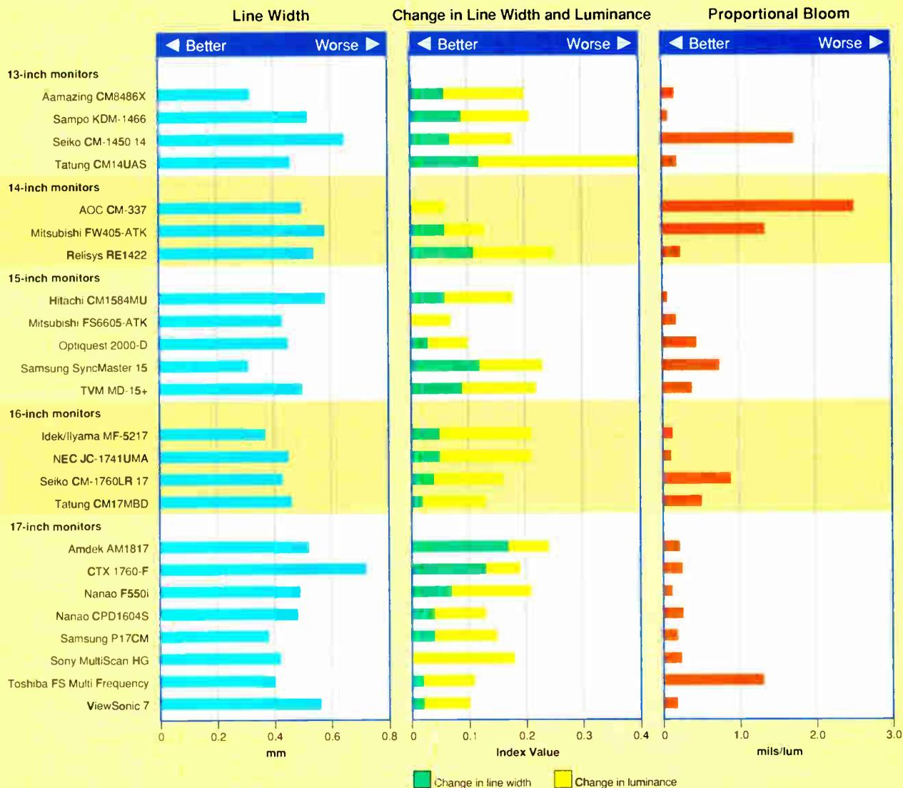
**Figure 1.** This test, which compares the horizontal line widths measured at the center of the screen, measures a monitor's ability to create fine, thin lines. Although no clear winners emerge, the Aamazing CM8486X and Samsung SyncMaster 15 come out slightly better than the others.
