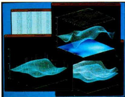
*PV-Wave:GTGrid uses well-location data with water-level information (upper left window) to create continuous mesh surface plots of the underground water table.*
