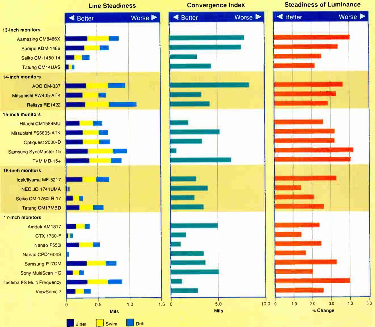
**Figure 4.** This test compares the consistency with which lines are placed on the screen; measurements are made at the center of the screen at 0.5-second (jitter), 10-second (swim), and 60-second (drift) intervals. Large values indicate an image that moves about the screen, which causes distortions in the color and brightness of the image. The NEC JC-1741UMA and Nanao T-560i perform very well in this test.
