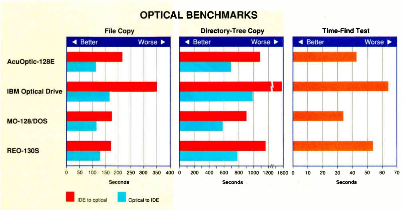
Benchmarks consisted of five components. The File Copy benchmarks measured the time needed to copy a 25-MB file from an IDE drive in the host computer to the optical drive and the time to copy the same file from the optical to the IDE drive. The Directory-Tree tests measured the time to copy tree structures in the same two ways. The Time-Find test measures the time taken to search for a nonexistent file. All results are in seconds.
