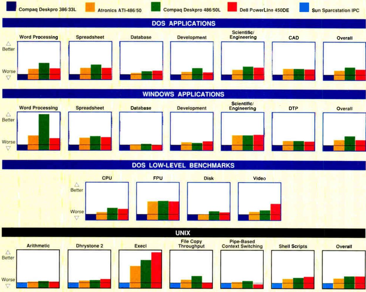
All results are indexed, and higher numbers indicate better performance. For each index in the DOS and Windows tests, a Compaq Deskpro 386/33L running Compaq DOS 5.0 and Windows 3.0 = 1. For each index in the Unix tests, a Sun Sparcstation IPC = 1. The overall index is the average index of the individual tests.
