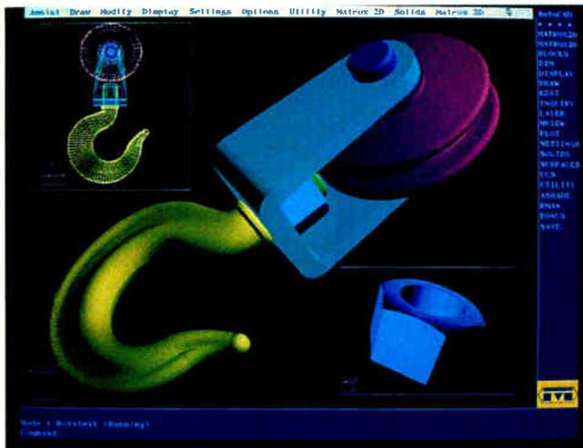
**Photo 1:** This AutoCAD design can be rapidly rotated in real time because the Gouraud calculations are supported by a Matrox MG-3D graphics board. Gouraud shading doesn't produce bright highlights, so the surfaces in this image appear opaque and plastic. (Courtesy of Matrox)
