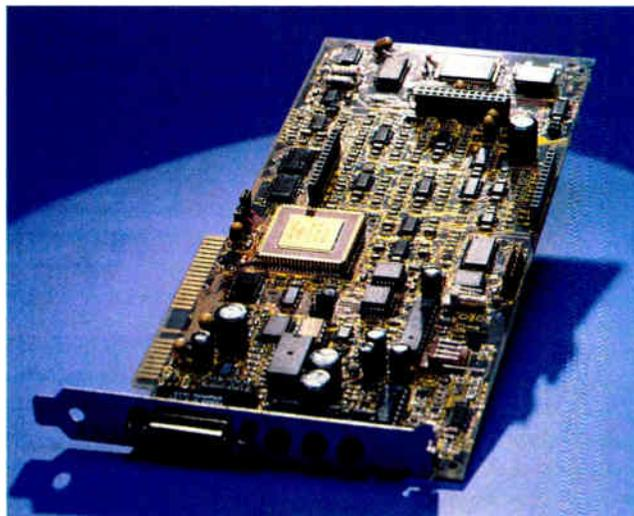
are two independent channels of 12-bit digital audio, which can record and play back 8-, 12-, or 16-bit files at bit rates of up to 44.1 kHz. The two channels can be used together to produce stereo, or they can be separated so that, for example, one can play a digitized musical score while the other offers running verbal commentary.
