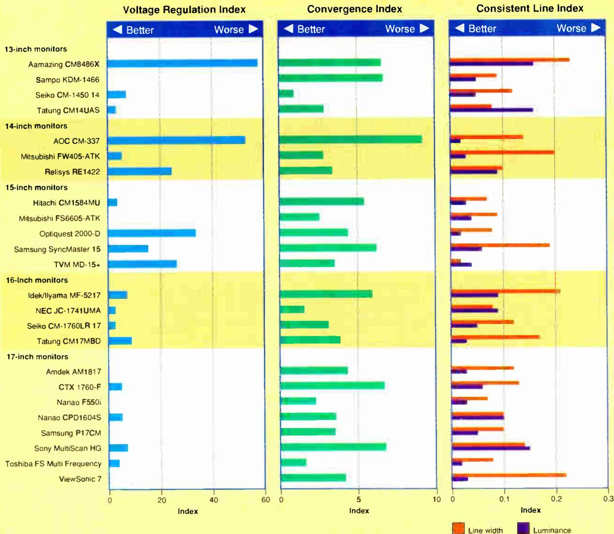
**Figure 7.** This test indicates how well a monitor can maintain a consistent image size as the contents of the screen change. A monitor's ability to maintain the size of an image is particularly important for multimedia applications such as full-screen movies. Six of the monitors tested do not show any noticeable change.
