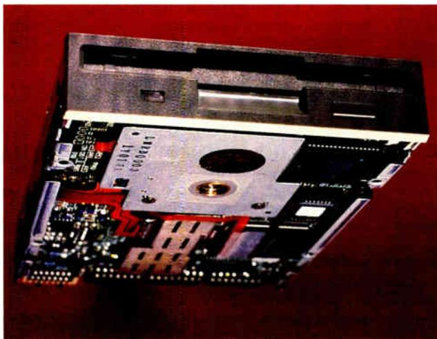
track pitch. Floptical uses closed-loop servo-positioned heads that read rings that are preprinted on special disks. The result is that Insite can cram 1245 tracks per inch
