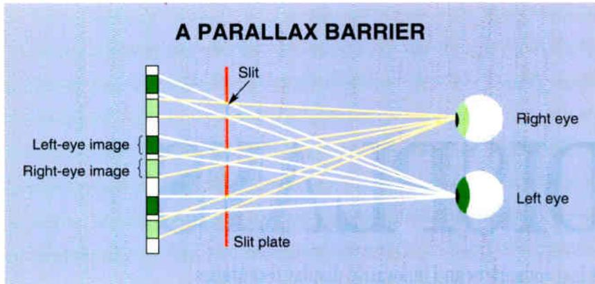
**Figure 1:** This cross section of a parallax-barrier system, seen from above, shows how the system sends different images to each eye. When you are the proper distance from the slit plate, each eye sees only the image strips meant for it. The slit plate occludes information meant for the other eye.
