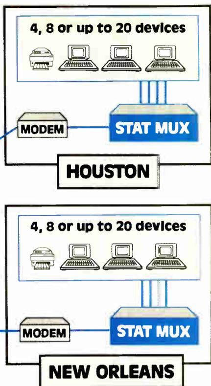
The Telplex® line of asynchronous statistical multiplexers by BayTech are designed to provide user flexibility and to maximize speed by effective utilization of high speed modem technology. Telplex stat muxes support hardwire connectivity for distances to 4000 feet.
