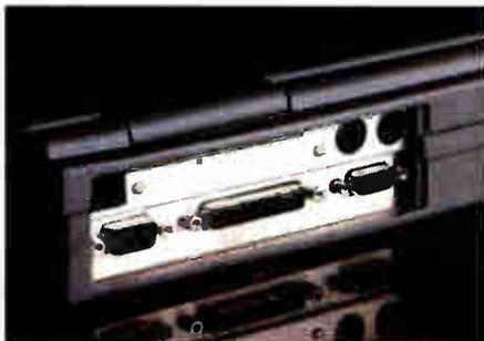
1 serial, 1 parallel port; fax/modem; keyboard; mouse; VGA monitor connections.
