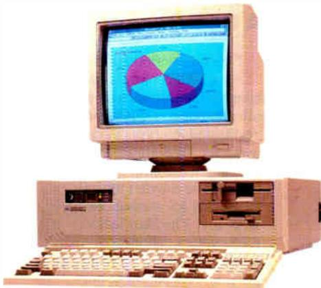
Step up to even greater expansion capability! Northgate's full-size desktop case is your best choice when space is no object. A 200 watt power supply provides plenty of power for your toughest applications. Expansion capacities include eight expansion slots plus space for three exposed and two internal 5.25" half-height devices.
