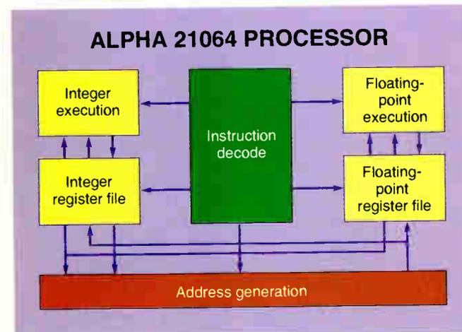
**Figure 2:** Avoiding bottlenecks is the goal of the Alpha core architecture, shown here with distributed floating-point and integer register files and execution logic.
