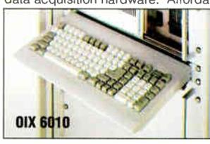
The rugged & reliable Elma keyboard shown here is made in the USA. It features extended 101-key layout, full-travel keys for touch-typing, and is only 1 rack-space (1.75") high. Call for information.
