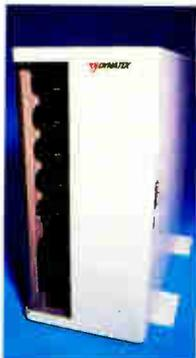
combination modules. Since each disk module includes its own power supply, there is no master power supply to become a single point of failure.
