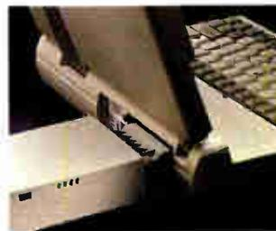
up to 15 Mbps, the unit is available in 40- to 180-MB capacities. The 1½- by 3½- by 7-inch unit includes a 3-hour battery, hardware data encryption, and user password protection. EasyStor's Easy-Step device driver software quickly configures most PCs to automatically recognize its presence.
