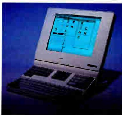
Combines Space-Saver Keyboard, LCD Monitor and 20 Mhz 386sx CPU w/2 Meg RAM (4 Meg optional) in a single very small footprint (27.4 X 26.0cm). Network ready with 10 Base2, 10 BaseT NE-2000 compatible network adapter built-in. Unit does not fold for portability.
