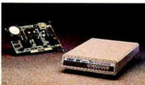
correction and data compression for 57,600-bps throughput. Including time-scheduled transmission, multiple-file broadcasting, and polling capabilities, the modems can also view, rotate, and print incoming faxes. The external version is available for Windows, DOS, and the Mac.
