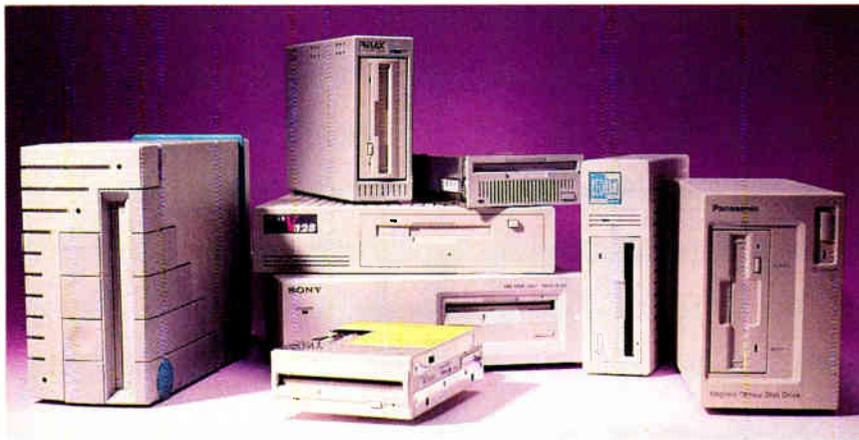
**Photo 1:** A collection of internally and externally mounted MO drives.
