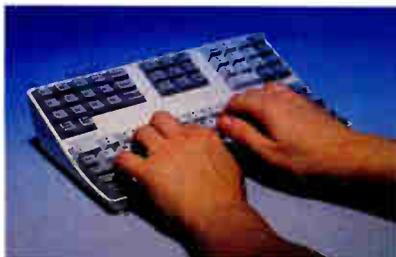
First successful alternative to conventional keyboard saves 60% desk space with a foot print of 27.3 x 15.2 cm. Has full travel tactily responsive keys with standard left-right spacing for easy touch typing. 100 keys, compatible with IBM XT/AT PS/2. Many language versions available.
