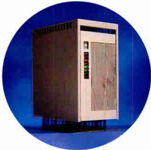
Get up to 4GB of fault-tolerant disk storage with the OmniArray parallel disk array. Northgate RAID technology uses four drives plus a fifth parity drive giving you true high disk fault tolerance and high data availability. Novell certified.
