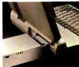
up to 15 Mbps, the unit is available in 40- to 180-MB capacities. The 1½- by 3½- by 7-inch unit includes a 3-hour battery, hardware data encryption, and user password protection. EasyStor's Easy-Step device driver software quickly configures most PCs to automatically recognize its presence.
