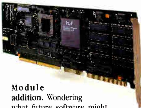
**Module addition.** Wondering what future software might require of your hardware? Our 486M PC's have a LocalBus slot for hardware accelerators that can solve long-term software problems.
