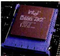
Pick your power! 486SX-25 thru the 486DX2-66. And upgrading is easy with our Zero Insertion Force (ZIF) socket. Note the extra row of pins for the future P24T!
