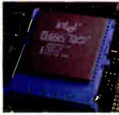
Pick your power! 486SX-25 thru the 486DX2-66. And upgrading is easy with our Zero Insertion Force (ZIF) socket. Note the extra row of pins for the future OverDrive™ CPU based on Intel's P5 technology.
