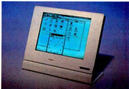
This 10" black on white monitor is easy-to-read, yet compact. Resolution is 640x480 with sharp, flicker-free image. Sharp's high refresh rate, triple supertwist nematic technology with back lighting provides a super bright, low radiation screen with a wide viewing angle. The adjustable monitor base is only 29x14 cm. It lets you mount the LCD monitor on vertical surfaces or fold for transport. Comes with 1.5 m cable and VGA adaptor card. No external power required. IBM AT compatible.
