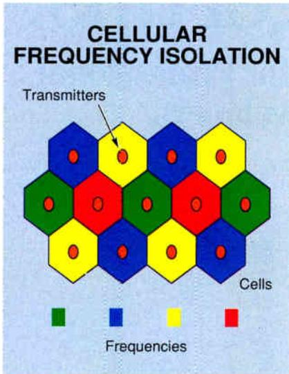
**Figure 1:** In cellular transmissions, the same frequencies can't be used in adjacent cells. Frequencies must be isolated to avoid interference.
