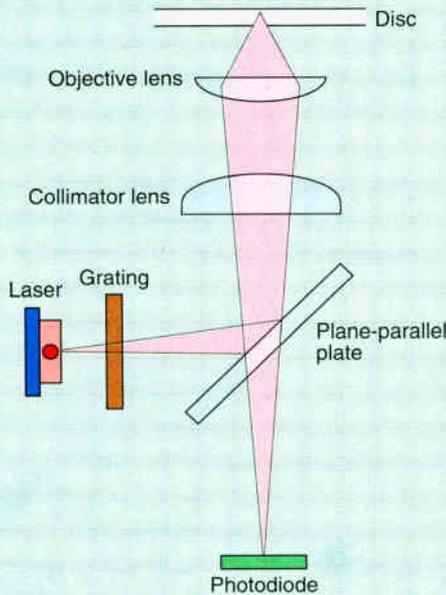
**b) CD-R drive laser mechanism**
