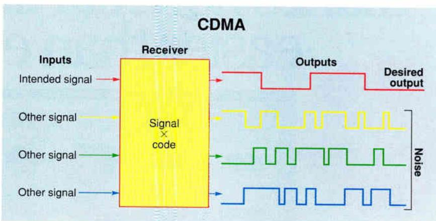
**Figure 2:** With CDMA, all users share the same frequency, but each signal is created with a unique code—the spreading code—that replicates the original signal when multiplied by the signal. As long as the receiver uses the same code, only one signal at the receiving end will decode clearly—that is, as something other than noise.
