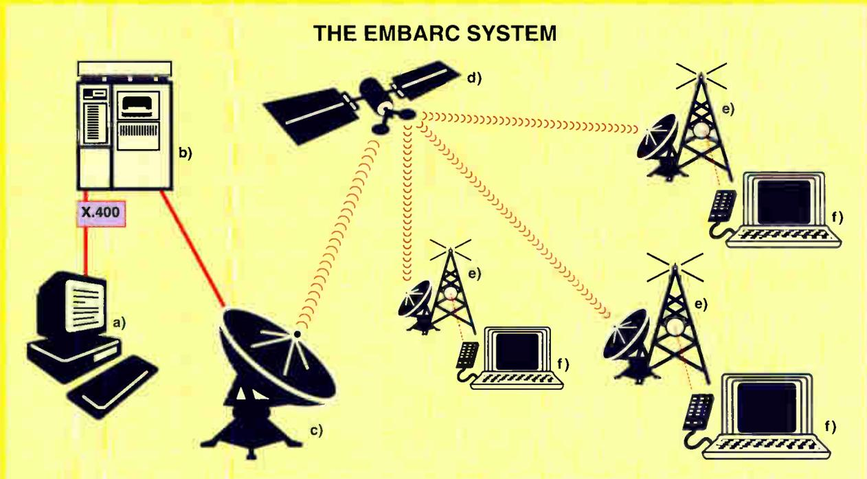
**Figure A:** You send an EMBARC message from your computer or workstation (a) using X.400 to the central EMBARC switch (b), where a satellite uplink (c) transmits it to a satellite (d). The satellite sends the message to downlink stations (e), which relay them to NewsStream receivers (f).
