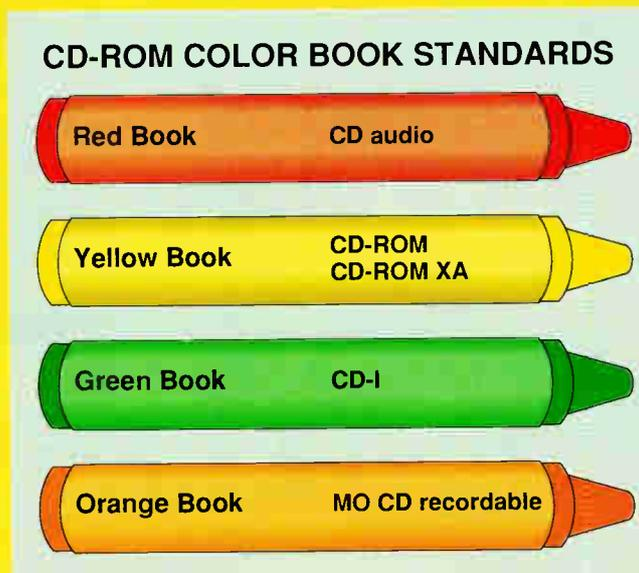
Figure A: CD-ROM standard specifications are categorized by color. The new color is Orange, which covers MO and CD-R.
