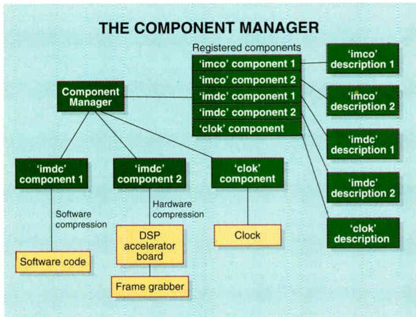
**Figure 3:** The Component Manager functions as a database that classifies objects by function and provides run-time binding to functional objects using the standard Toolbox routines. It allows applications to find predefined classes of software and objects and registers hardware resources. Here, 'imdc' represents the image decompression manager, 'imco' represents the compression manager, and 'clock' represents the system clock.
