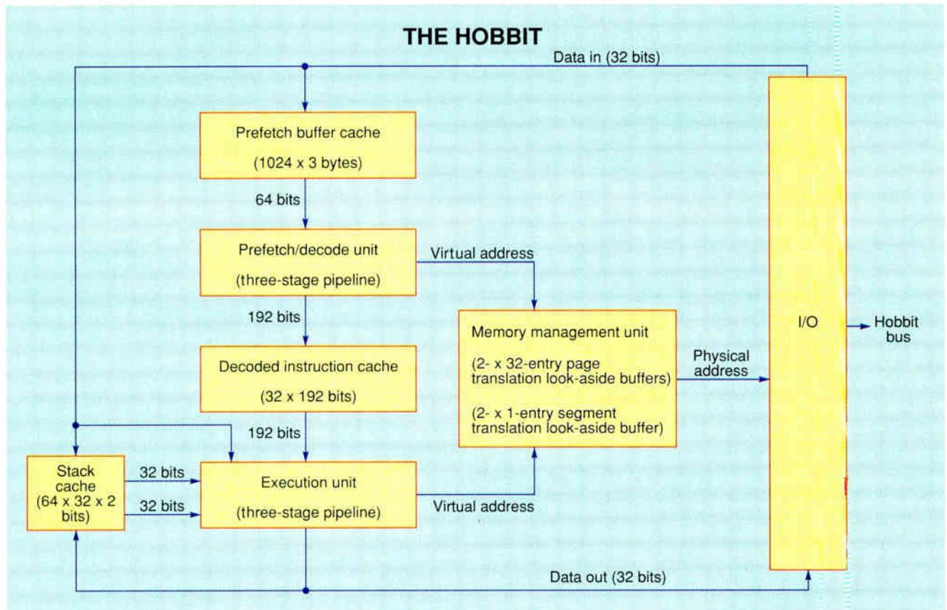
**Figure 1:** The primary execution pathway in the Hobbit consists of two three-stage pipelines coupled by a cache. The prefetch/decode unit transforms instructions into the 192-bit format that the execution unit requires. The execution unit determines addresses, fetches operands, and computes and stores results. If an operand is in the stack cache, it's available to the pipeline without delay. (Courtesy of AT&T Microelectronics)
