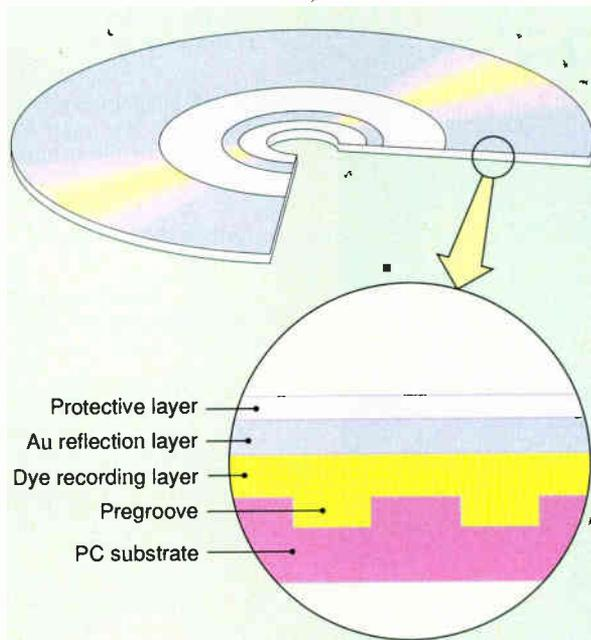
**Figure 2:** The CD-R media consist of four layers: the top protective layer, the gold (Au) reflection layer, the dye recording layer, and the PC substrate. The CD-R laser heats the reflection, recording, and substrate layers. As a result, the recording layer fuses and is impressed by the expanding substrate layer. (Figure courtesy of Philips Consumer Electronics Co.)
