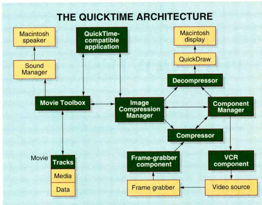
**Figure 1:** QuickTime applications interact with the Image Compression Manager, which shields the application from compression details, and the Movie Toolbox, which controls access to movie data. The ICM interacts with the Component Manager, compressor, and decompressor. In this figure, QuickTime elements appear in green.
