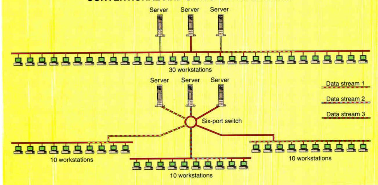
**Figure 2:** In a conventional Ethernet network with three file servers shared among 30 workstations, only one conversation can take place at a time. With a three-by-three switch added to the network, you can have three conversations on the network at once.
