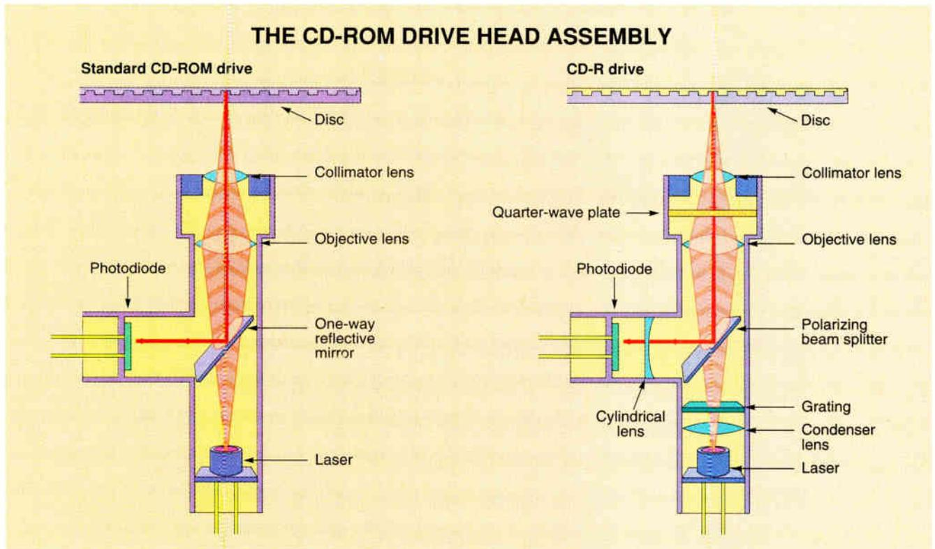
**Figure 2:** In standard CD-ROM and CD-R drives, a laser beam passes through a one-way mirror or polarizer and a set of lenses on its way to the disc. Reflected light passes through the lenses and is redirected to a photodiode.
