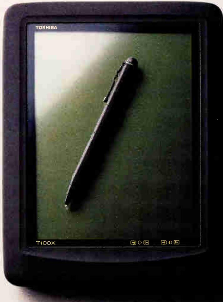
The Toshiba Dynapad makes most of its predecessors look clunky by comparison. Packed into this sleek, little 3.3-pound tablet is a 9.5" transreflective-sidelit display, 40MB hard drive and two PCMCIA 2.0 slots. Clearly a 3rd-generation pen computer, the innovative engineering in the pen market has
