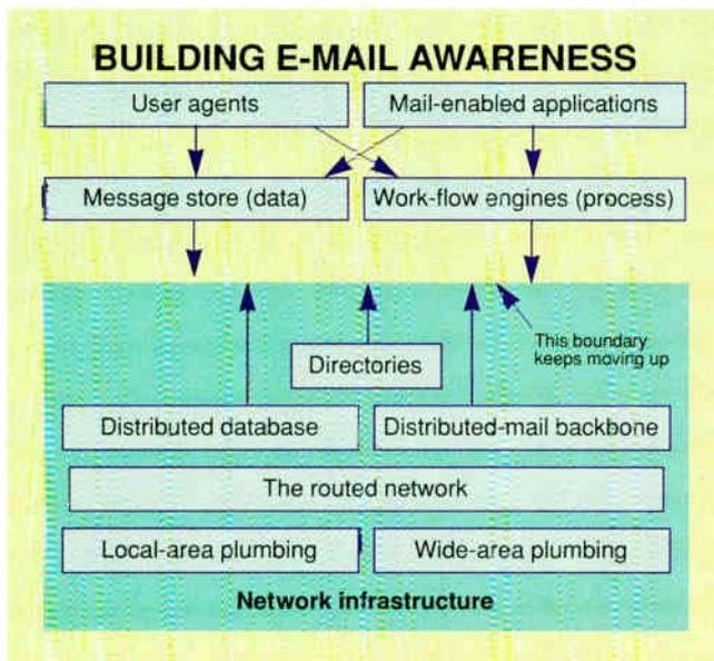
**Figure 1:** The messaging architecture of the future will let mail-enabled applications and messaging agents communicate interchangeably with message stores and work-flow engines. This layered design permits users to use the networks, mail services, and front ends of their choice.
