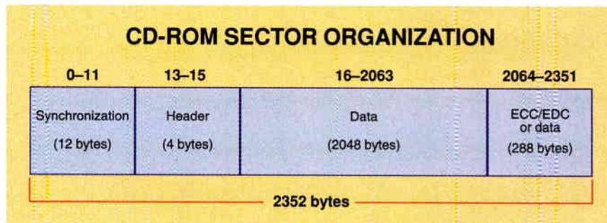
**Figure 4:** A typical CD-ROM disc sector can contain either 2048 bytes of error-corrected data or 2336 bytes of uncorrected data. Dispensing with error correction (which is recommended only for more tolerant audio or video data) expands the disc capacity by more than 50 MB.
