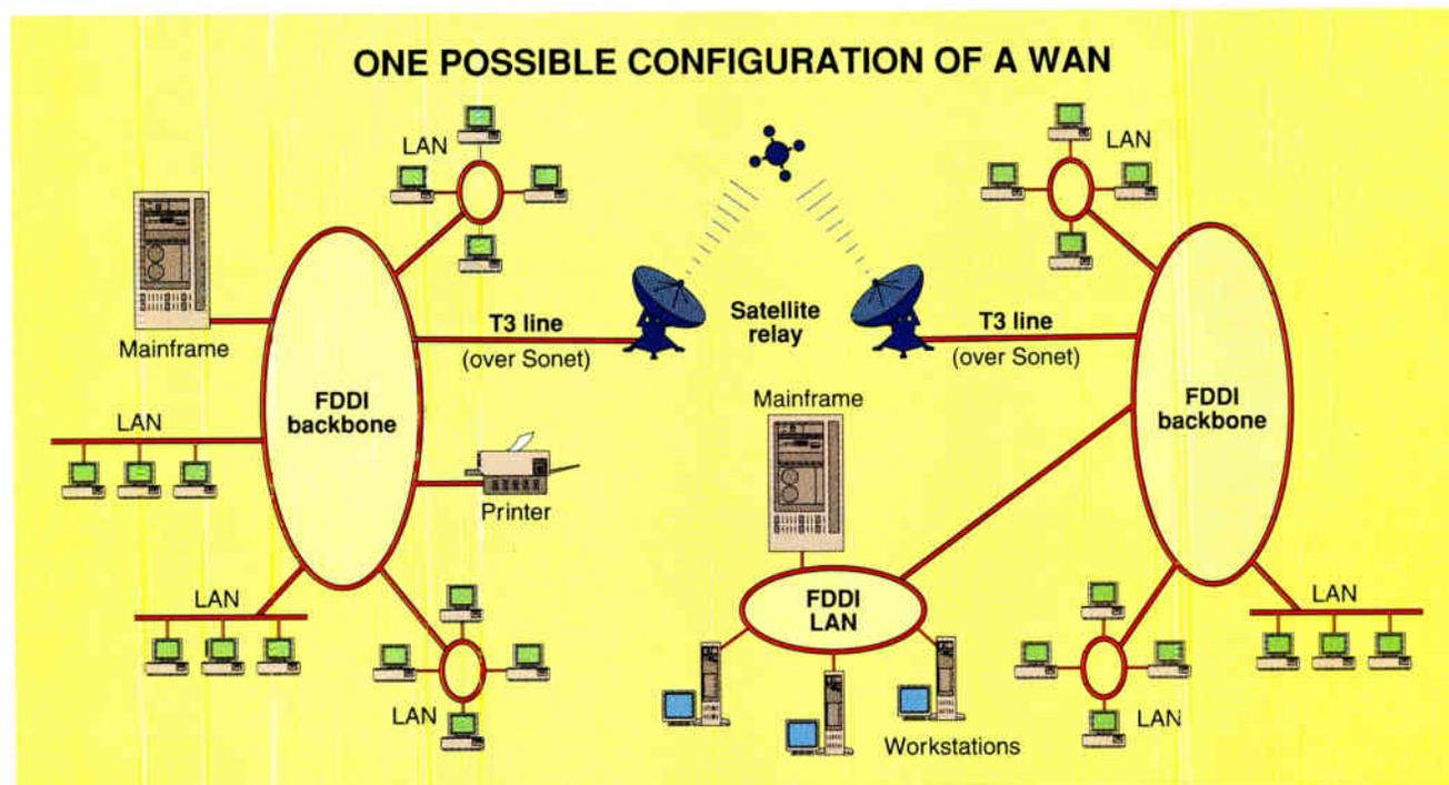
**Figure 1:** LANs connect to each other over a backbone network. In this example, FDDI, a 100-Mbps optical-fiber network, provides the connection. Backbone networks can be connected to each other via a variety of private and public services, including leased lines and satellite links.
