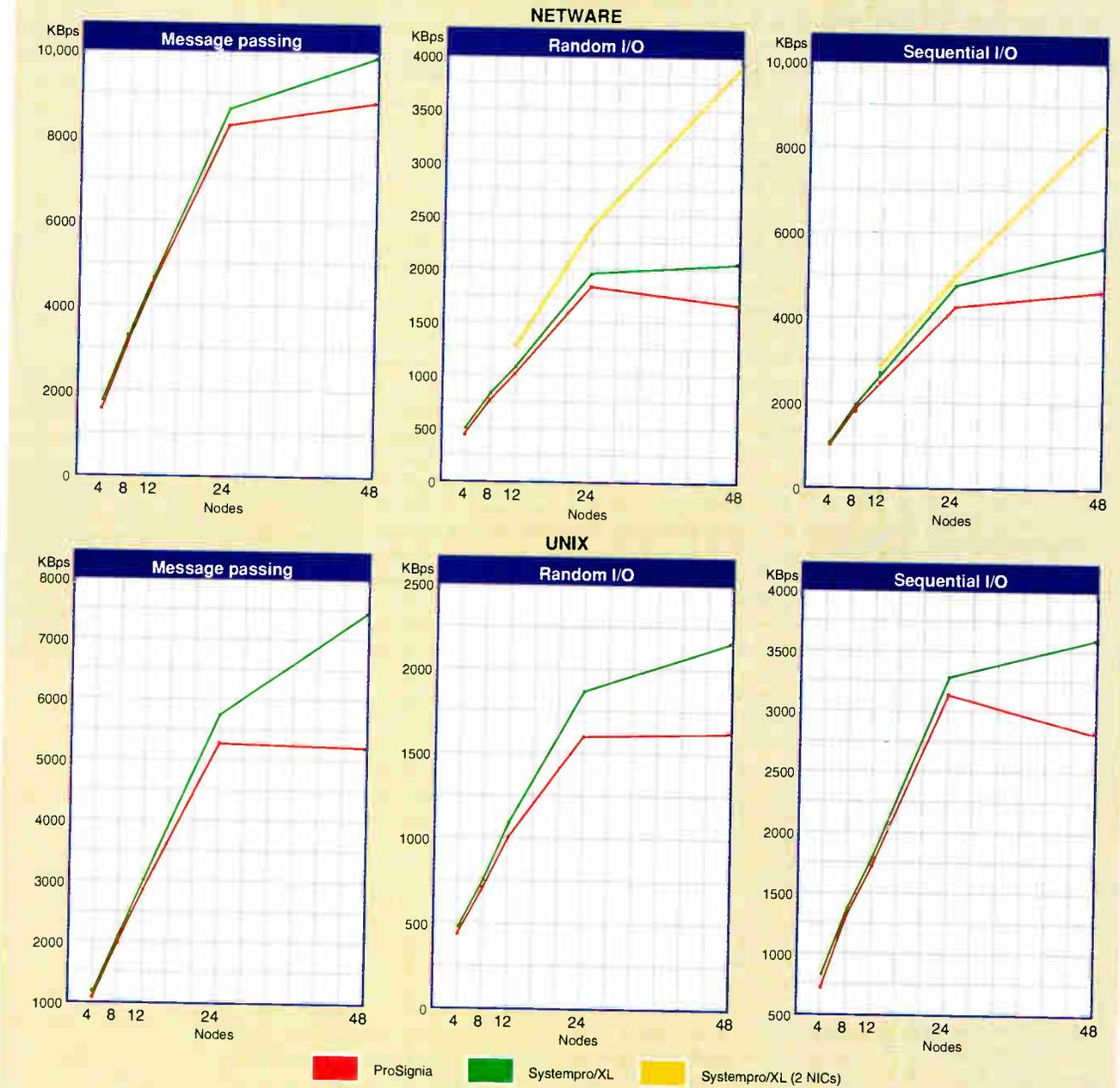
Figure 1: NetWare benchmark results show that both servers are fast but that the Systempro/XL has considerably higher capacity than the ProSignia. The XL shows no degradation at all with two NICs installed. It ran in a dual-processor configuration on the Unix tests, but because I/O is such a significant component of the BYTE Unix Network Benchmarks, the XL doesn't show much benefit.
