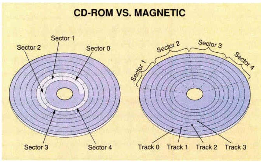
**Figure 1:** CD-ROM discs use a continuous spiral track that has sectors of equal length (left). Magnetic hard disks organize data into concentric circular tracks and divide the tracks into sectors of varying sizes (right). This design has a marked effect on performance.
