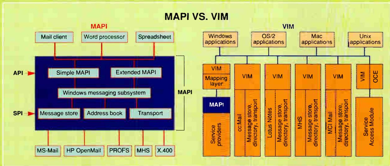
**Figure A:** Microsoft's MAPI and Lotus's VIM specifications offer top-level APIs that let applications talk to mail back ends. In the Windows-only MAPI, the layer interfaces to mail engines via drivers, while in the cross-platform VIM, the layer is actually part of the engine itself.
