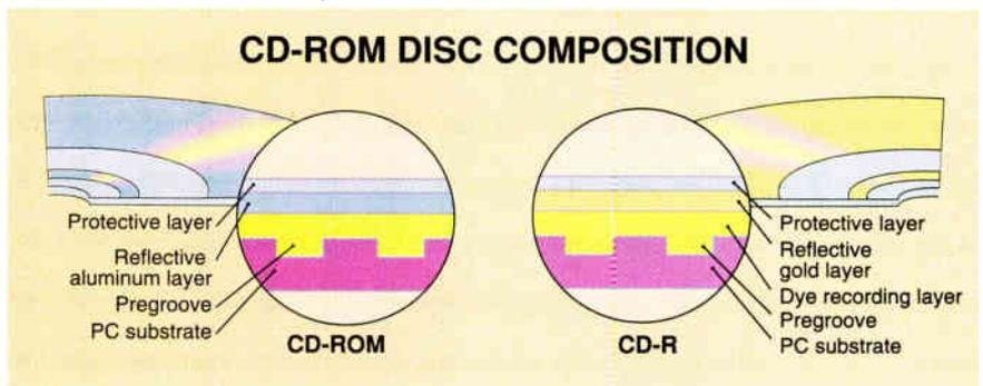
**Figure 3:** In a standard CD-ROM disc, a manufacturer impresses a pattern of lands and pits into a transparent polycarbonate substrate, which is backed with a reflective aluminum film, a coat of lacquer, and the vendor's label. The drive reads the disc from the bottom, through the substrate. The substrate layer on a CD-R disc is coated with an organic-dye recording layer, a gold layer, and a lacquer coating.
