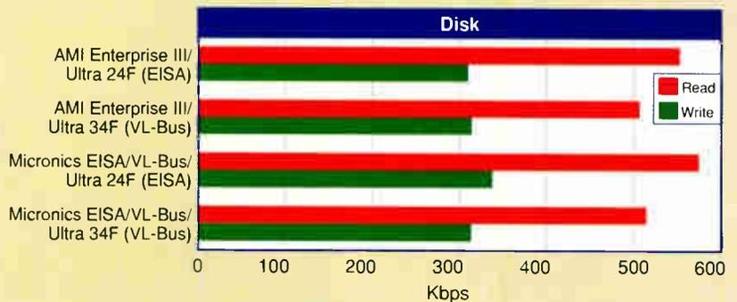
**Figure 1:** Disk tests show similar performance for both system boards using VL-Bus peripherals. However, the Micronics EISA/VL-Bus System Board is somewhat faster as the basis for an EISA design.
