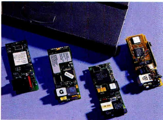
**Photo 2:** Internal modems for the PowerBook (from left to right): PSI Integration's PowerModem IV, Global Village's PowerPort/Gold, Supra's SupraFaxModem 144PB, and Applied Engineering's DataLink PB.
