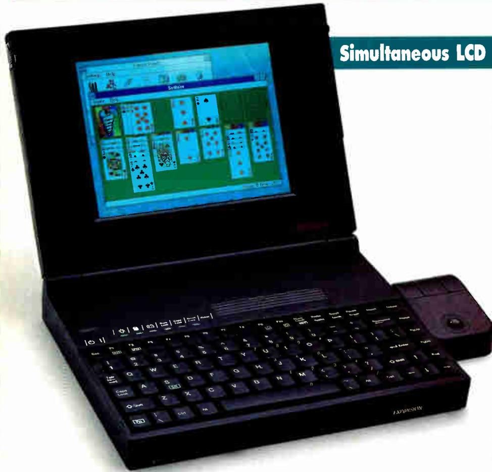
Simultaneous LCD & External SVGA!
