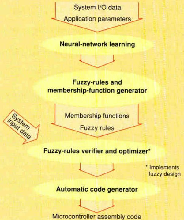
National Semiconductor's NeuFuz system combines fuzzy logic and neural networks, which learn the system behavior based on I/O data, and a rules generator, which creates fuzzy rules and membership functions based on the neural-network learning process. A fuzzy-rule verifier validates and optimizes the number of generated rules and functions. Finally, an automatic code generator converts these rules and functions into an embedded controller's assembly code.
