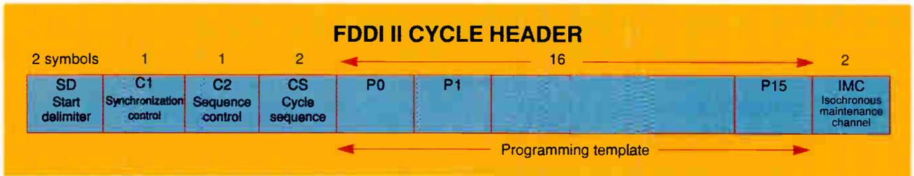
**Figure 3:** The cycle header appears at the start of each cycle. It provides synchronization and housekeeping information and defines the channel allocation used.
