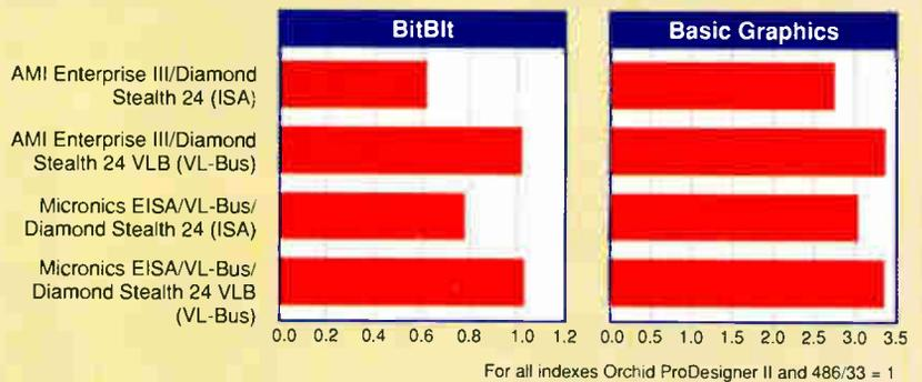
**Figure 2:** Video benchmarks for both motherboards, running over ISA and over VL-Bus. The BitBlt test, especially, shows a substantial performance increase when run through a VL-Bus video card.
