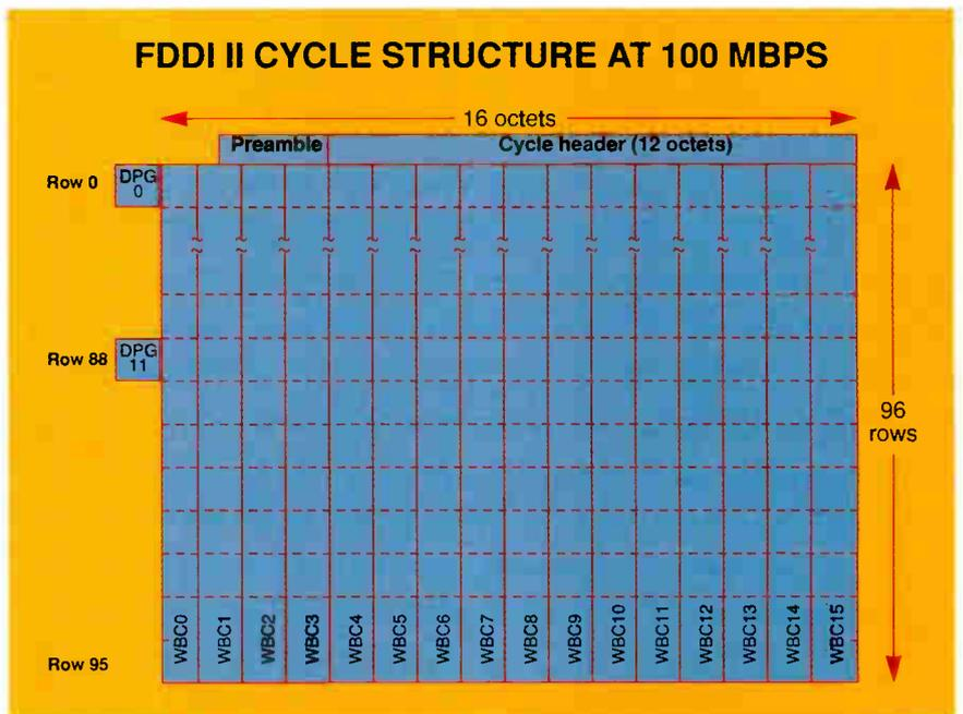
**Figure 2:** FDDI II imposes a framing structure on 100-Mbps traffic. The specification divides this structure into several channels to provide both packet-switching and circuit-switching facilities.
