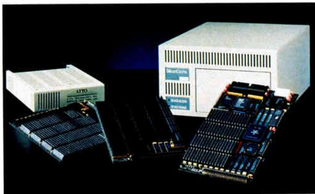
*SiliconCache uses special caching hardware and adaptive software for access times under 0.03 ms. The device can manage up to 512 MB of cache memory.*
