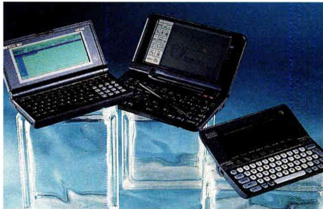
**Photo 2:** *Palmtop computers can usually fit in a coat pocket. They can handle scheduling, note-taking, and some pretty serious spreadsheet work—but forget touch-typing.*
