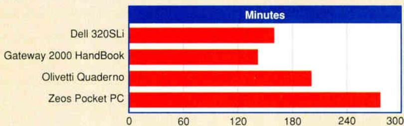
Tests performed by the BYTE Lab indicate the type of battery life you can expect without power-conservation features. The Zeos Pocket PC used alkaline batteries; the other units were tested with rechargeable batteries.
