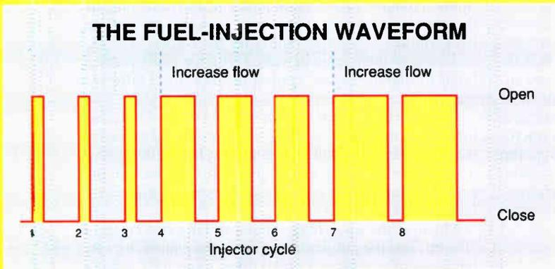
**Figure A:** Fuel injectors work by pulse-width modulation of fuel flow. Computers such as Ford's EEC-IV can easily generate such waveforms to control the fuel-injection process.
