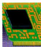
**DAUGHTERCARD:** This board plugs into a special connector on the motherboard and links the Pentium to a secondary cache at CPU speed over a 64-bit bus.
