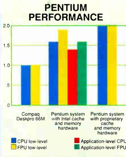
**Figure A:** Pentium systems can provide nearly twice the performance of a Compaq Deskpro 66M with a 66-MHz 486DX2. One Pentium system, which had its own CPU support circuitry, did better than the other systems we tested.
