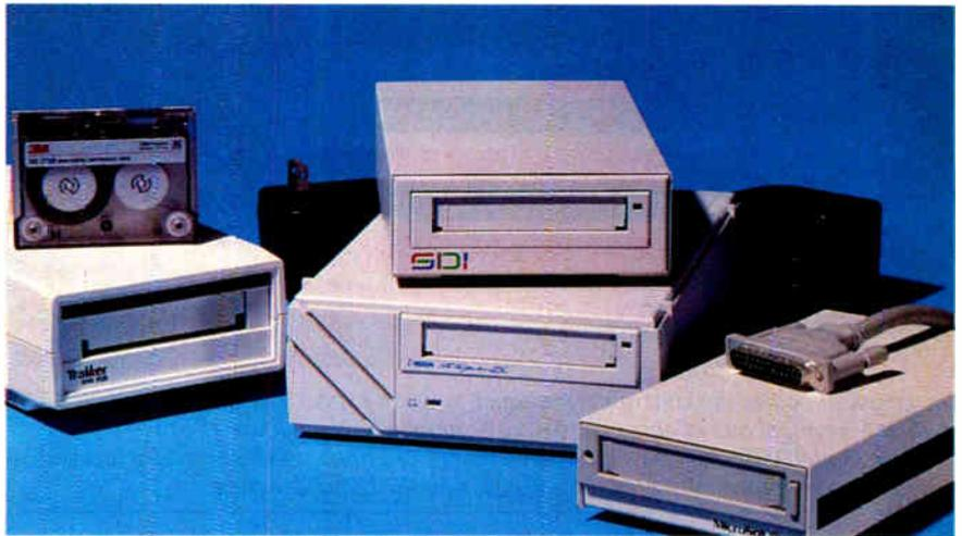
*Portable tape drives connect to your PC through a standard printer port and provide tape backup-and-restore functions. Pass-through connections let you keep your printer connected at the same time. From left to right: Colorado Memory Systems' Jumbo Trakker 250, SDI's Model 250P (top), Iomega's Tape250, and Micro Solutions' Backpack tape drive. All except the Iomega Tape250 use an external power brick (the Trakker's is a bit large for portable use).*
