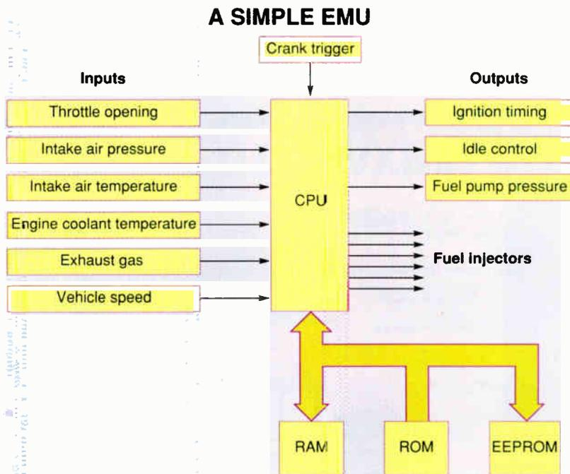
**Figure 1:** A typical EMU processes multiple inputs using engine "maps" in RAM, ROM, or EEPROM to control engine fuel injectors and ignition and idle controls. The turning crankshaft serves as the CPU clock.
