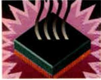
**HEAT DISSIPATION:** The Pentium runs hot. Intel is providing system vendors with thermal models, but vendors will have to pay close attention to fan and component location.
