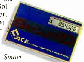
*Smart cards coupled with unique identification numbers for each user are one way of authenticating system users. (Photo courtesy of Security Dynamics)*
