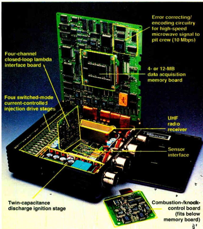
**Photo 2:** The Tagtronic 2.12F multiprocessor racing control system includes seven Siemens 80C166 CPUs and three Analog Devices 2101-2111 DSPs (hidden from view) that crank out 106 MIPS. Most processing cycles are spent handling I/O from over 40 inputs. A data acquisition board performs real-time diagnostics that are transmitted to pit crew engineers via a microwave link. The engineers then transmit modified engine data maps to the unit's UHF receiver on the fly.
