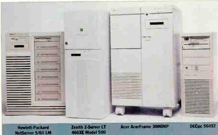
Look for designs that allow adequate air-flow through the system; Intel recommends a minimum of 400 feet per minute.
