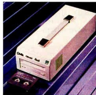
the drive can achieve capacities of up to 8 GB. The TS5450 is available with a SCSI connection in lieu of the parallel port and comes with software for DOS, Windows, OS/2, Unix, Xenix, and NetWare.
